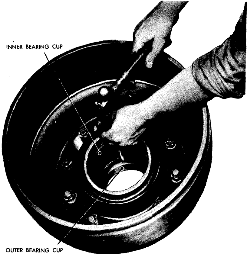
Figure 57—Removing Bearing Cups
