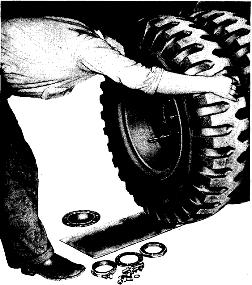
Figure 35—Removing Wheel and Hub Assembly
