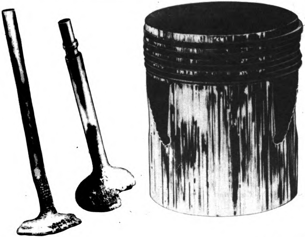
Figure 33 – Burned Valves and Scored Piston, Damaged by Overheating
