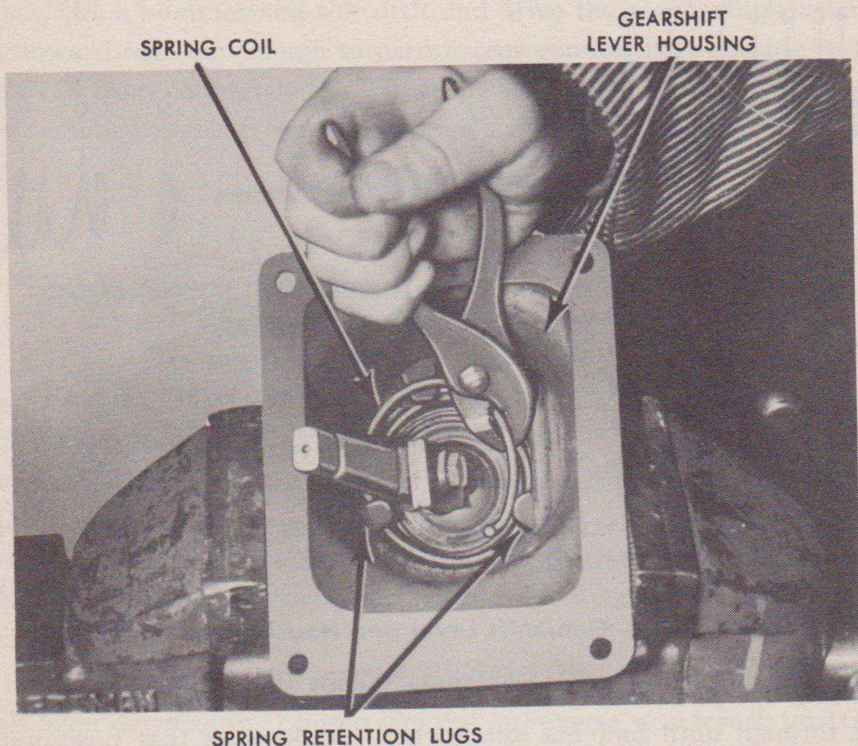
Figure 24 — Removing Ball Spring
