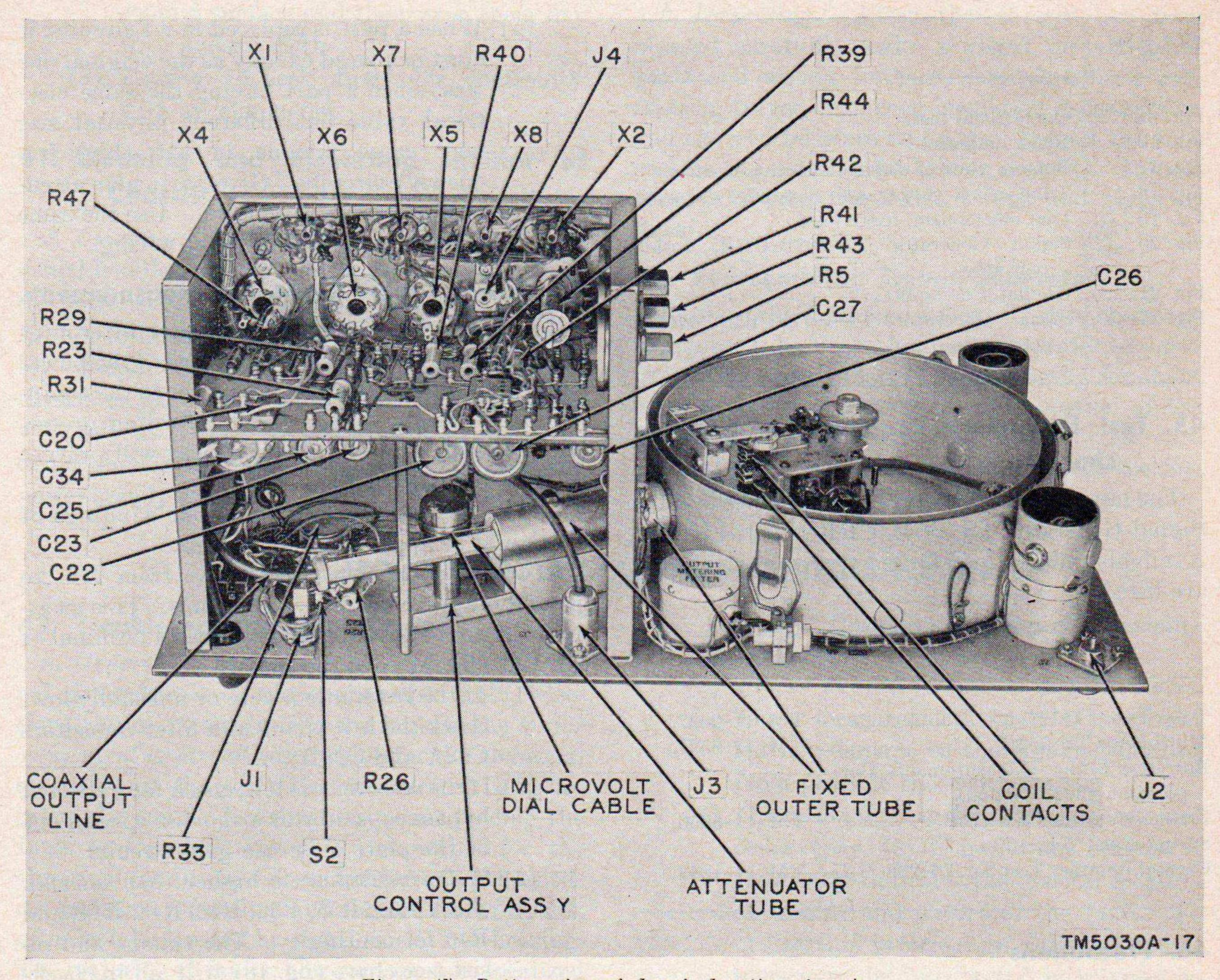
Figure 17. Bottom view of chassis, location of parts.
