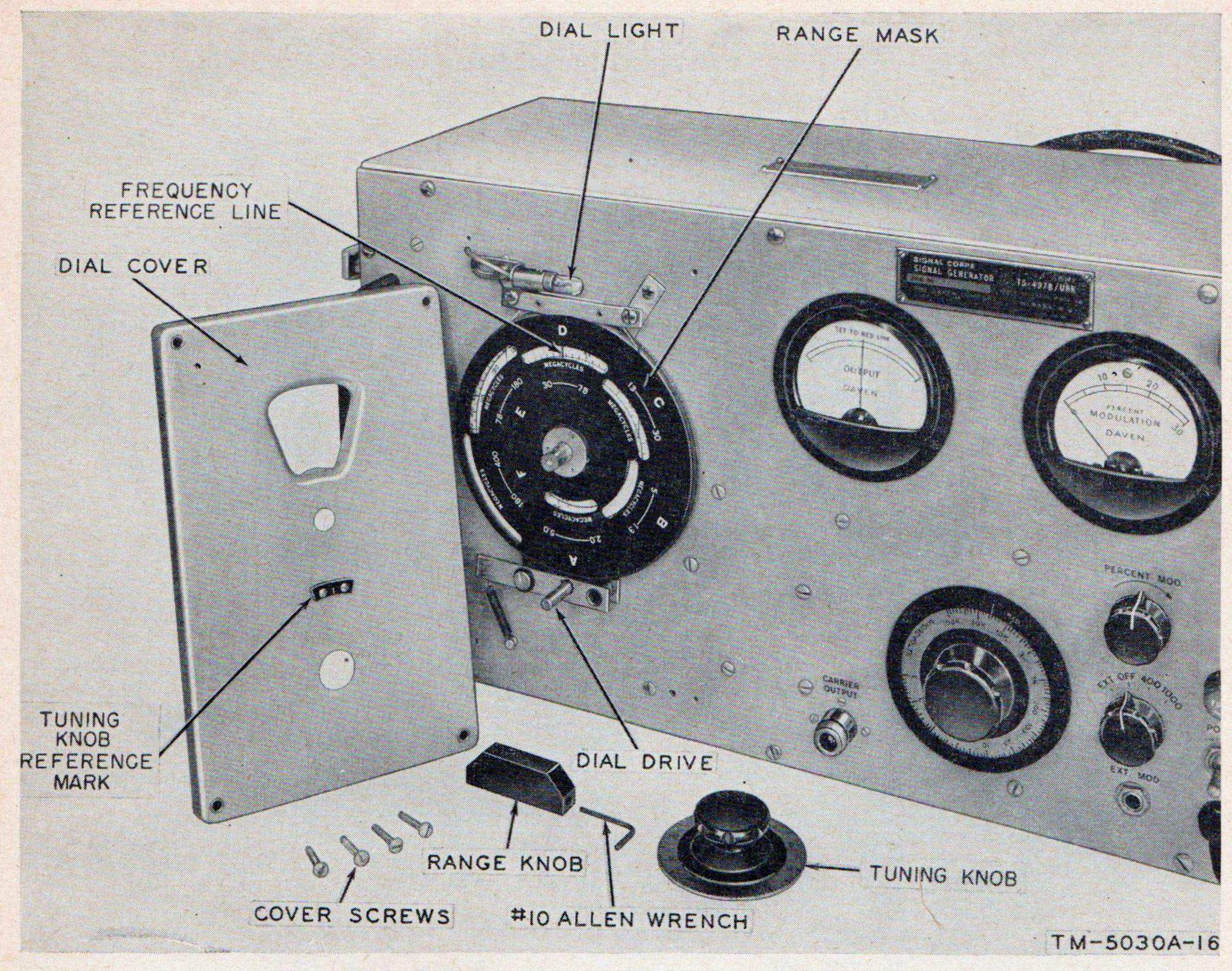
Figure 19. Dial mechanism, front view.
