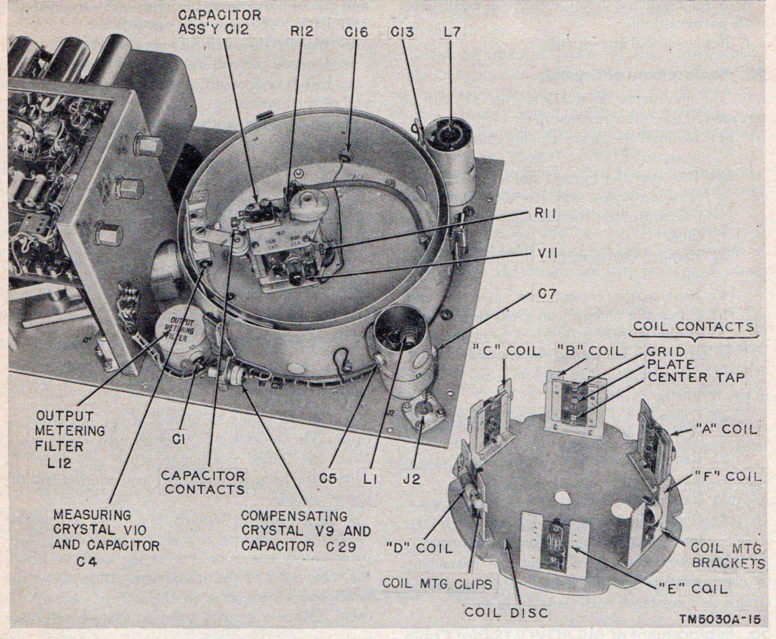
Figure 21. Oscillator assembly.
