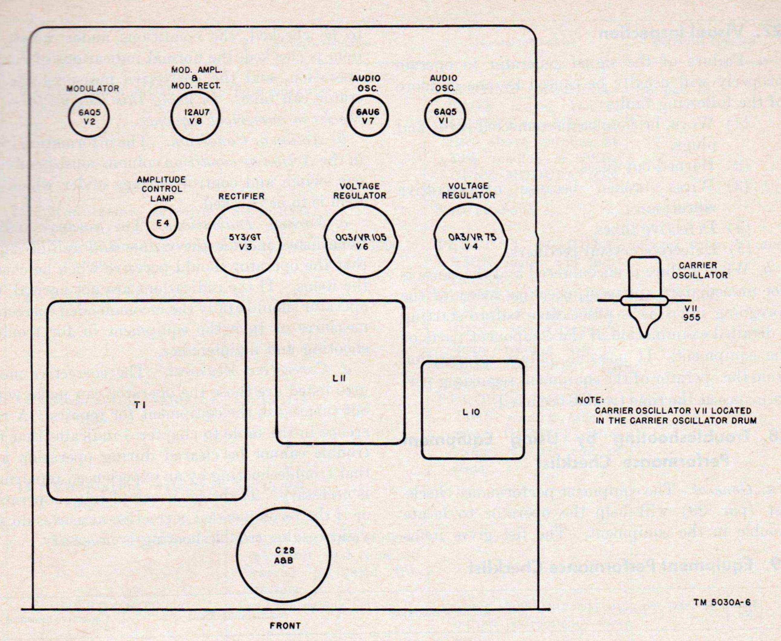
Figure 9. Tube location diagram.
