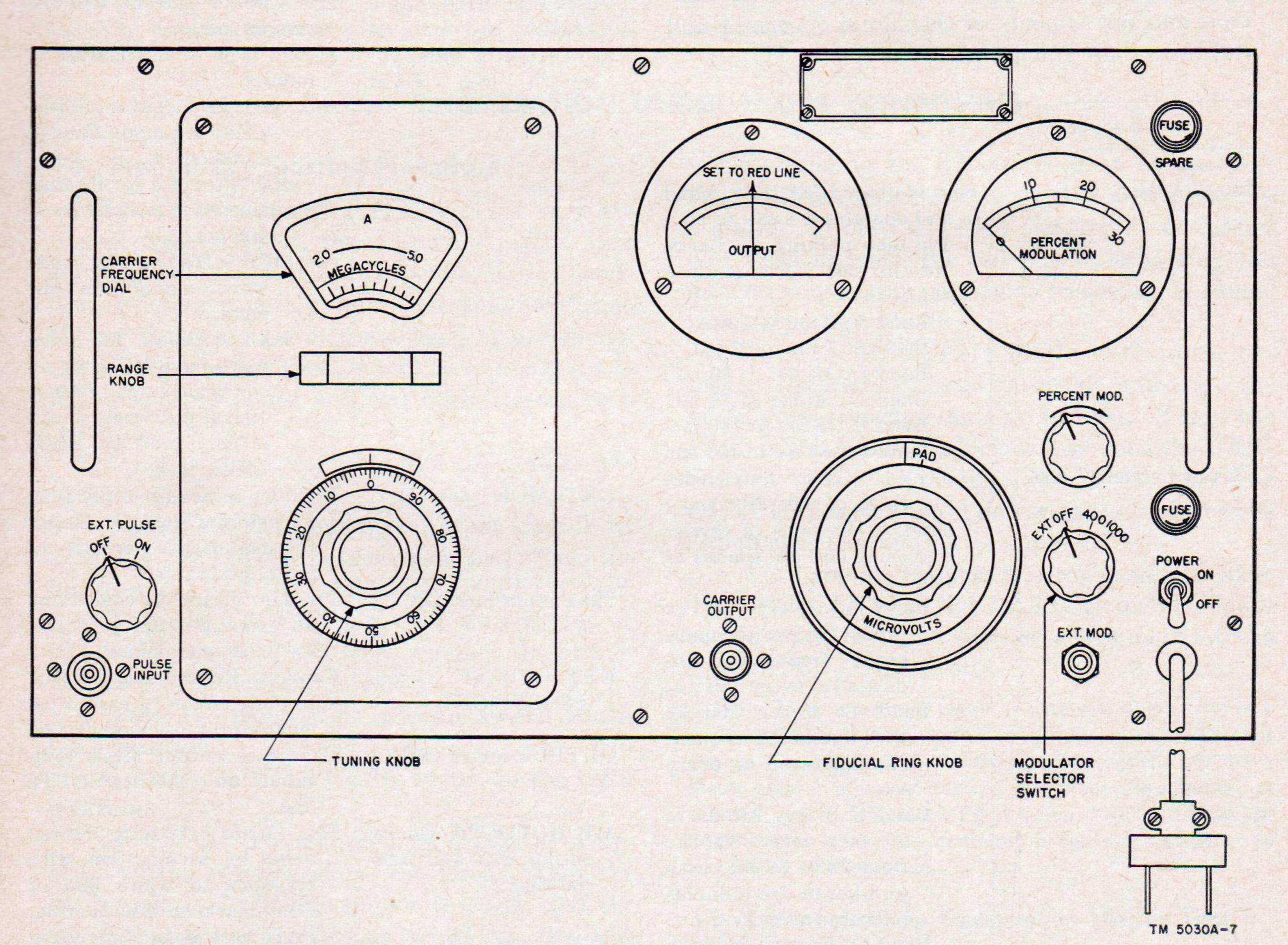
Figure 5. Signal Generator TS-497B/URR, front panel.
