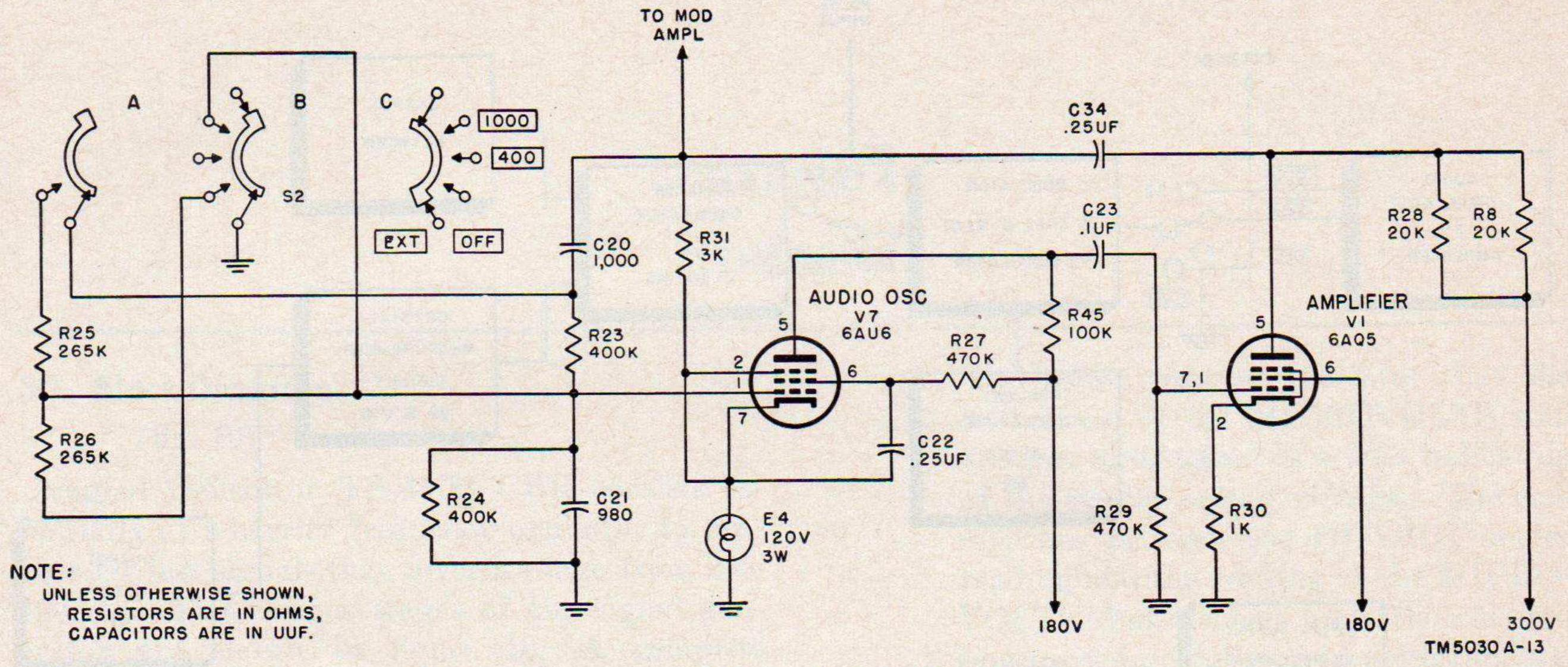
Figure 11. Audio oscillator schematic.
