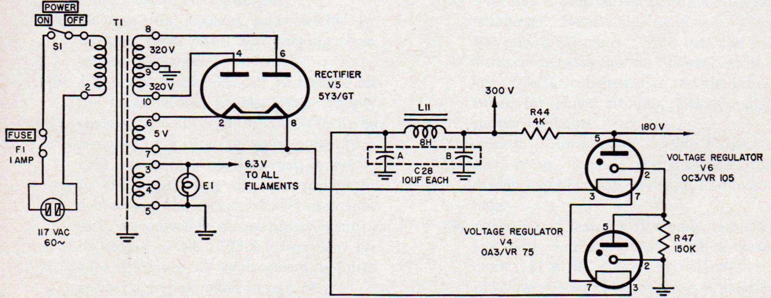
Figure 16. Power supply schematic.
