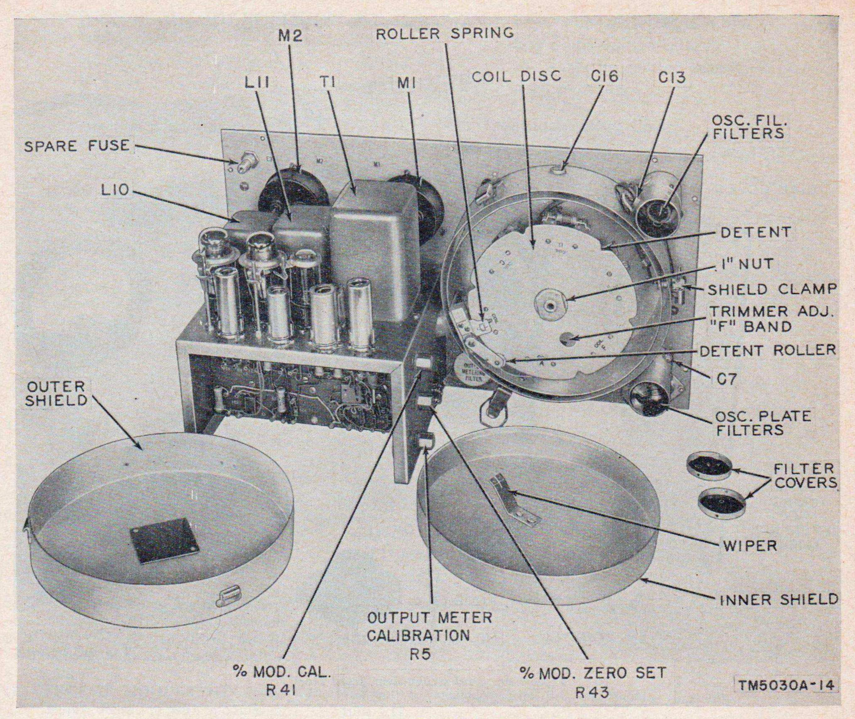
Figure 20. Signal Generator TS-497B/URR, inside rear view.
