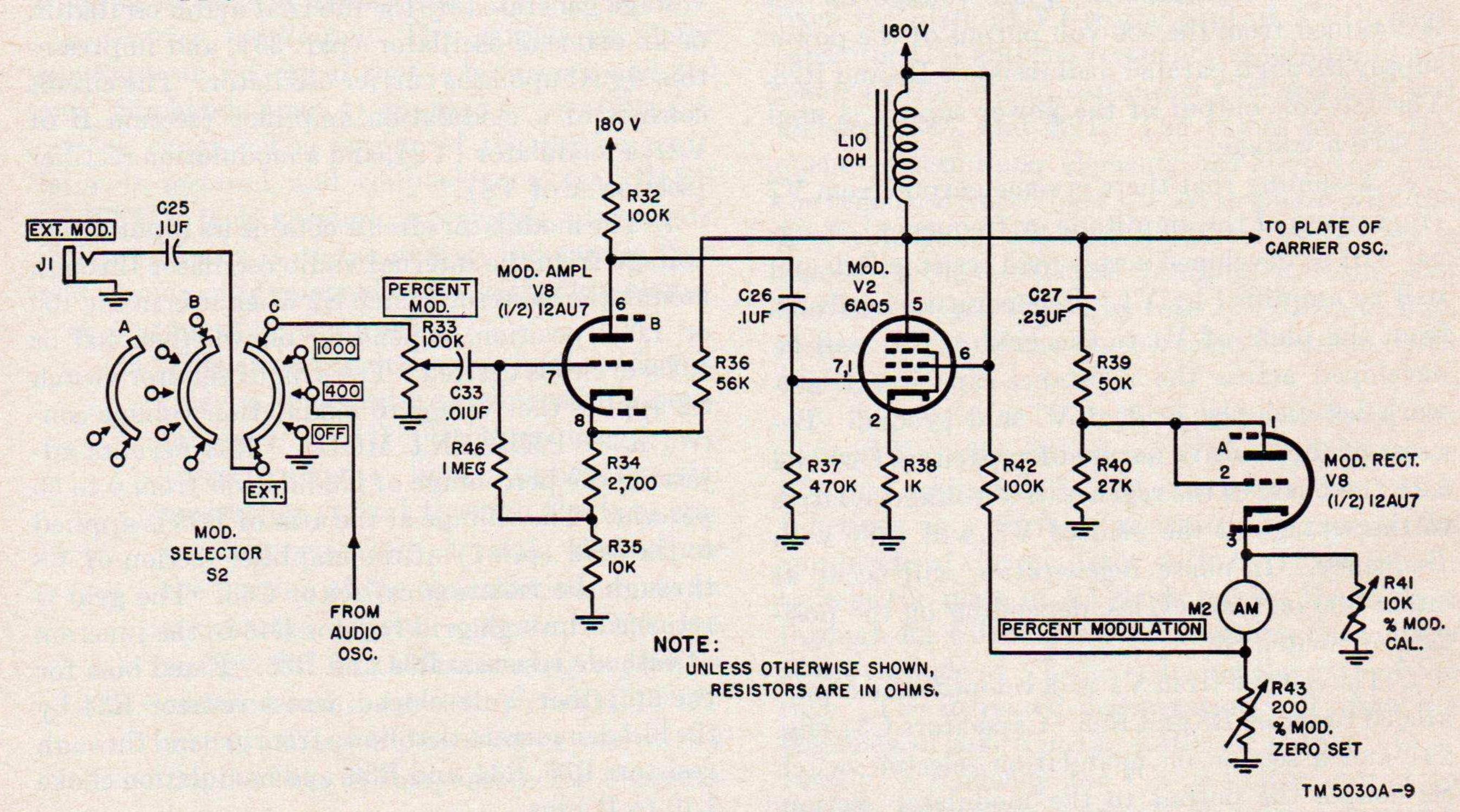
Figure 12. Sine-wave modulator schematic.
