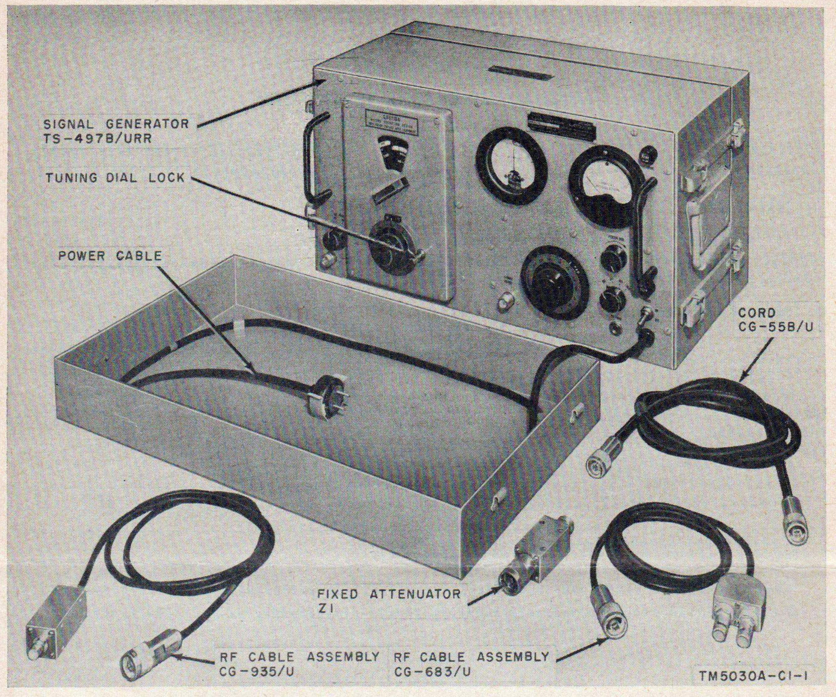
Figure 2.1. (Added) Signal Generator TS-497B/URR, front view (equipments bearing Orders No. 33772-Phila-53 and 25661-Phila-54).
