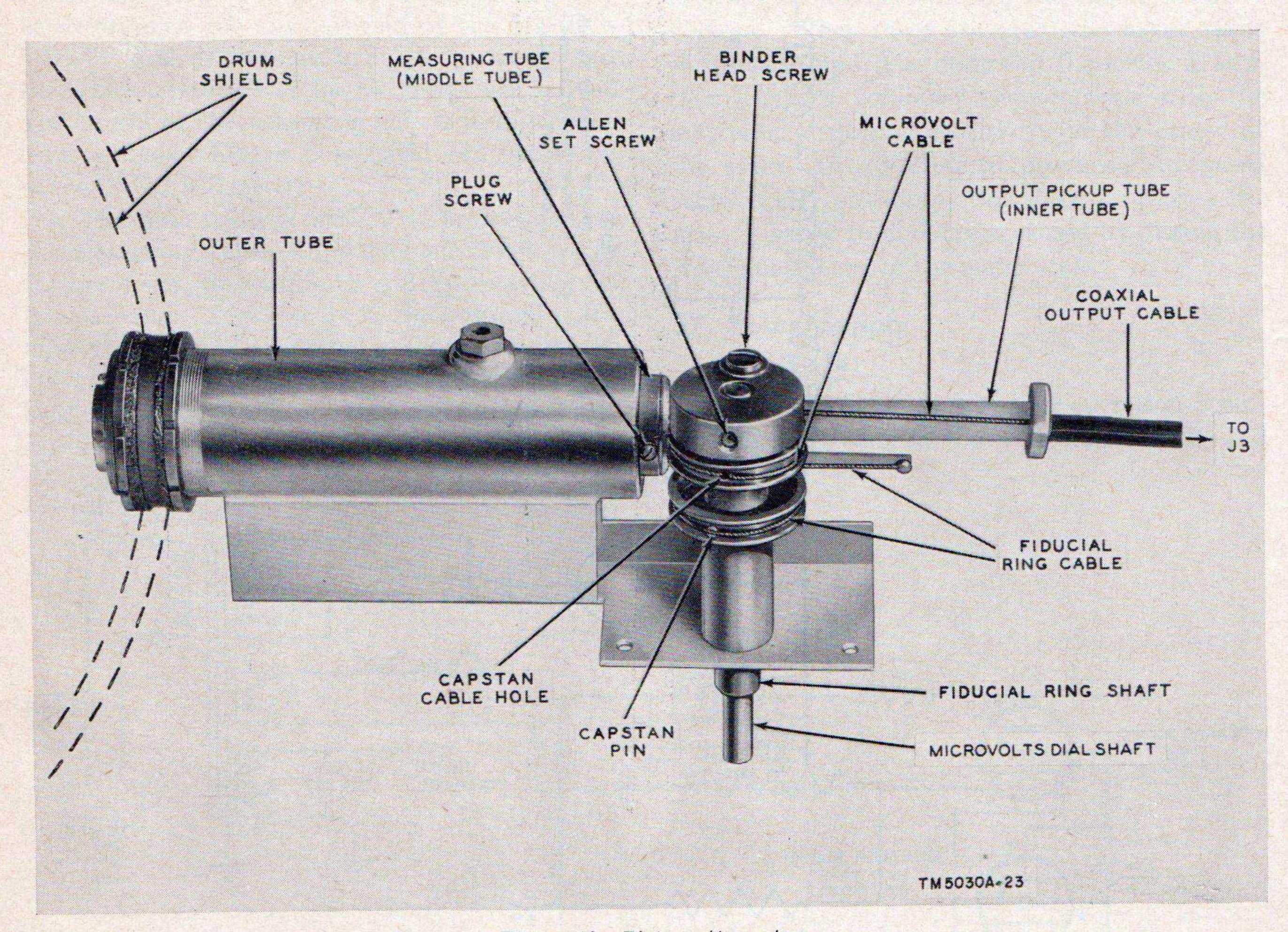
Figure 14. Piston attenuator.
