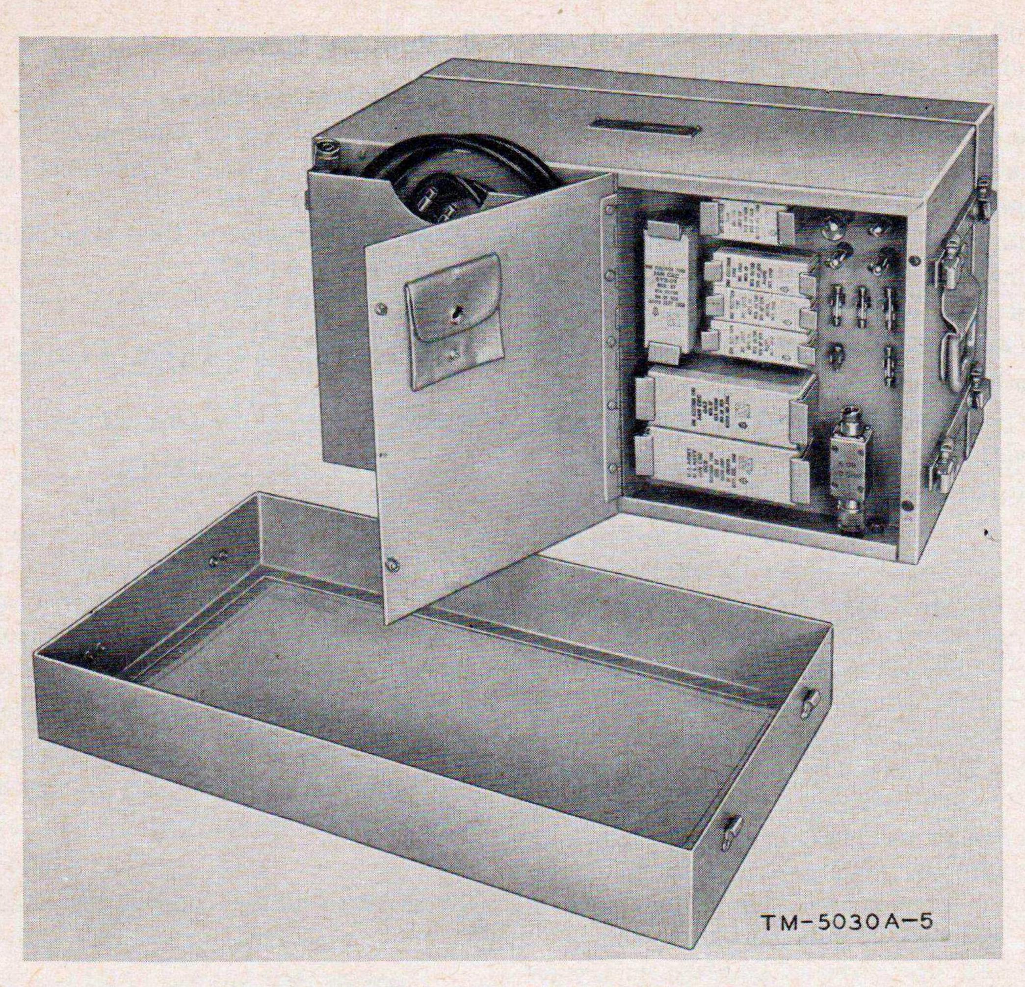
Figure 3. Signal Generator TS-497B/URR, rear view.
