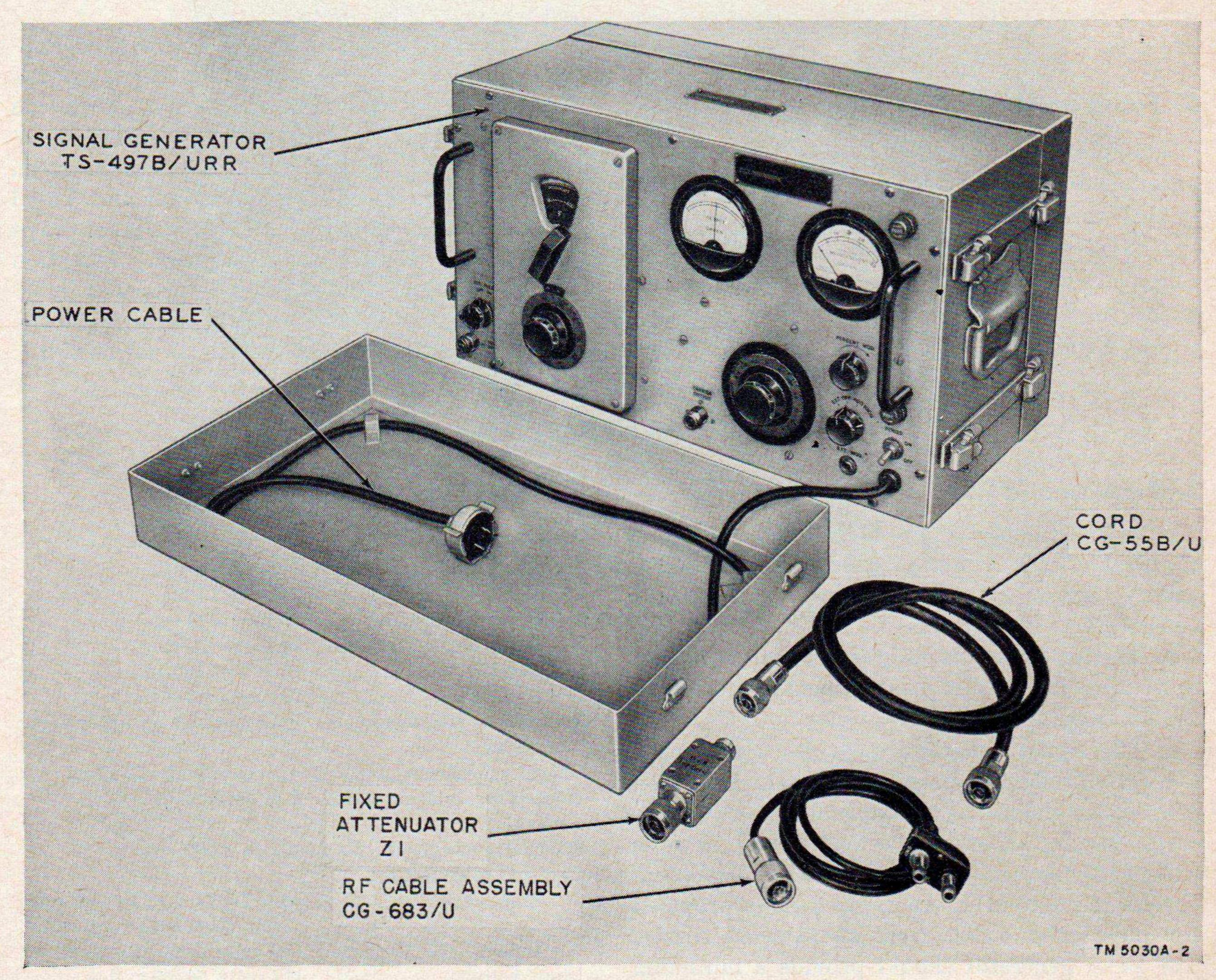
Figure 2. Signal Generator TS-497B/URR, front view.
