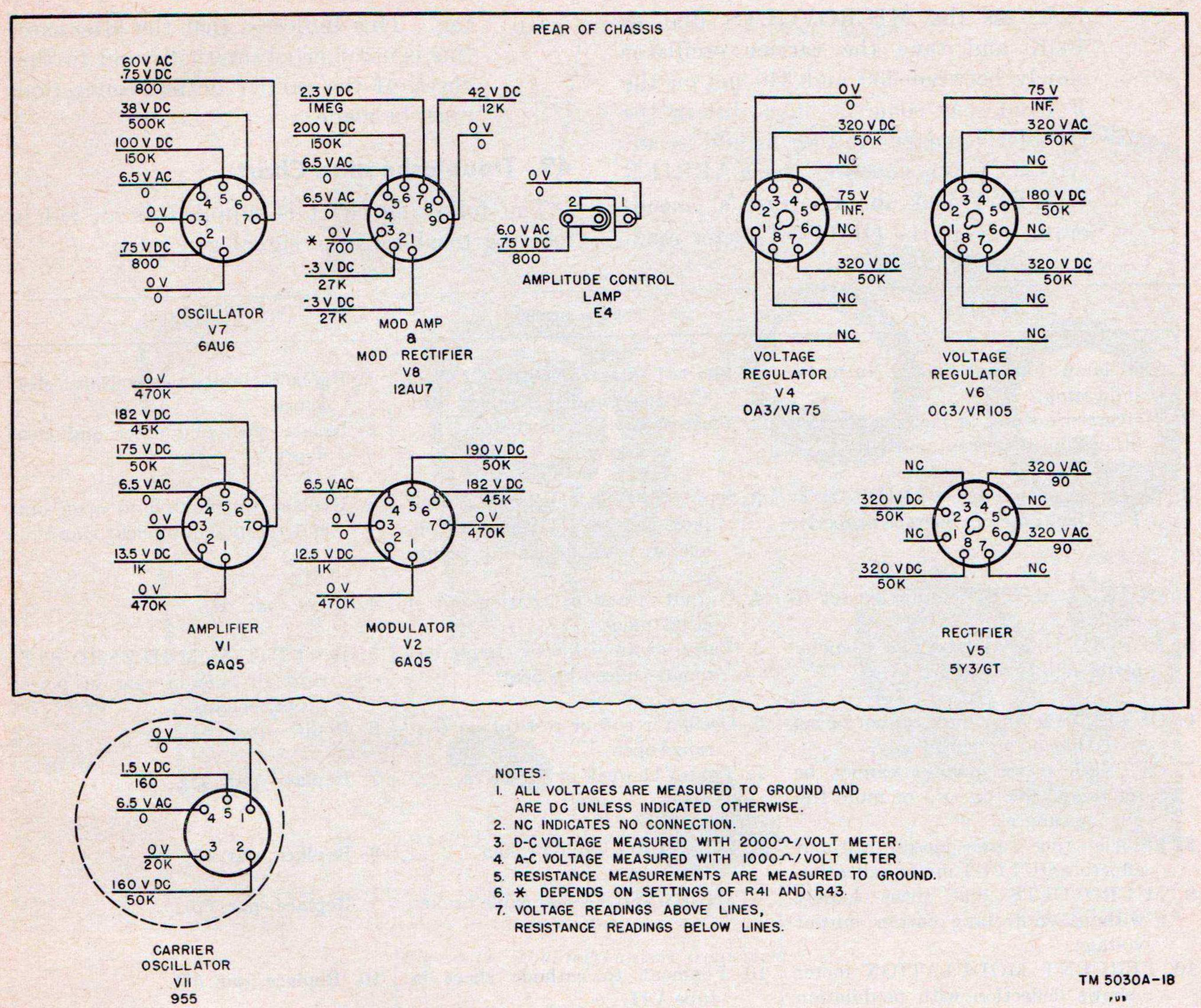
Figure 18. Tube socket voltage and resistance diagram.
