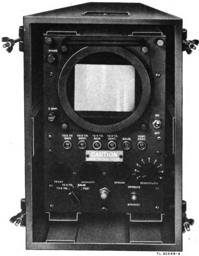
Figure 13—Control Unit BC-1378, front panel.
