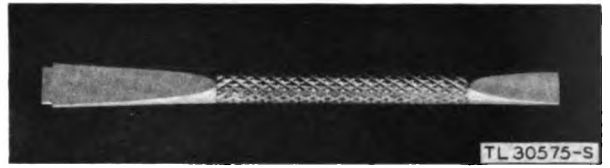
Figure 30—Special screwdriver for CALIB. controls.
