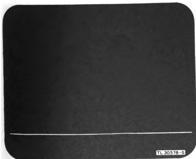
Figure 39—Sweep positioned correctly for operation.
