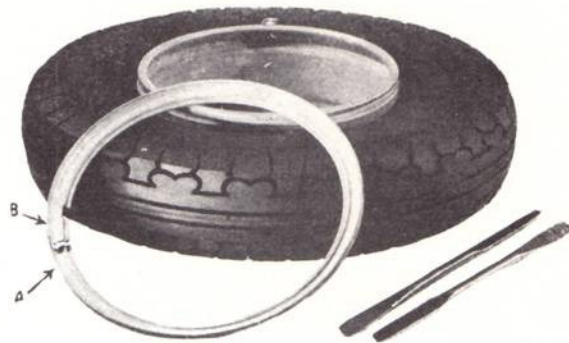
Type LTS side ring application —Place end "A" of ring in gutter of rim base.
