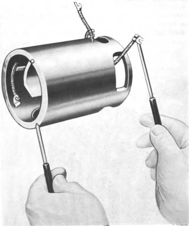
Figure 90. Testing field coils for ground.
