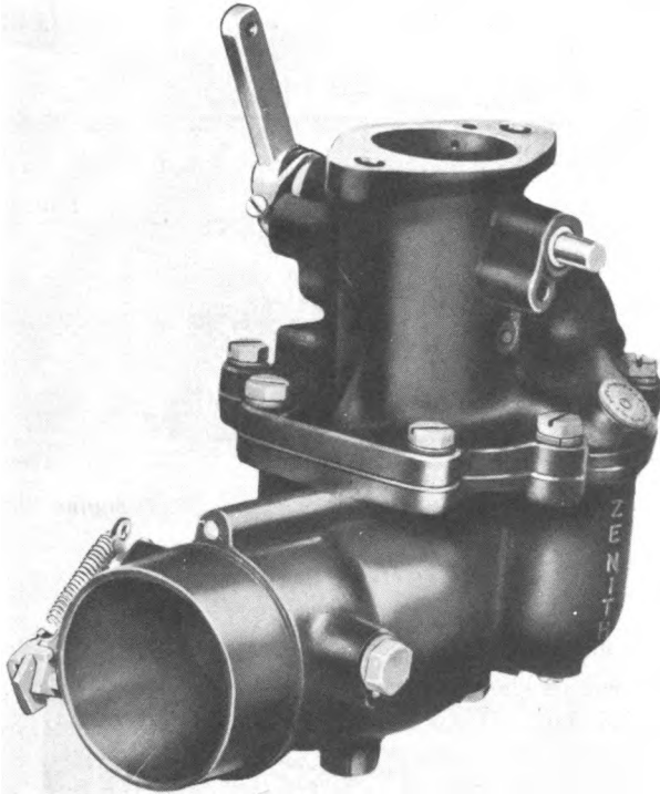
Figure 9. Carburetor identification, JXC engine.
