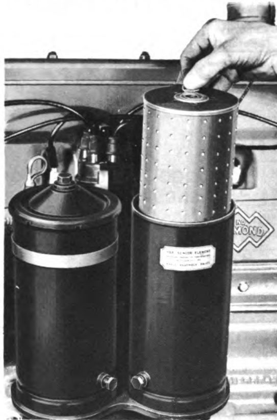
Figure 26 – Oil Filter Cartridge – Installation
