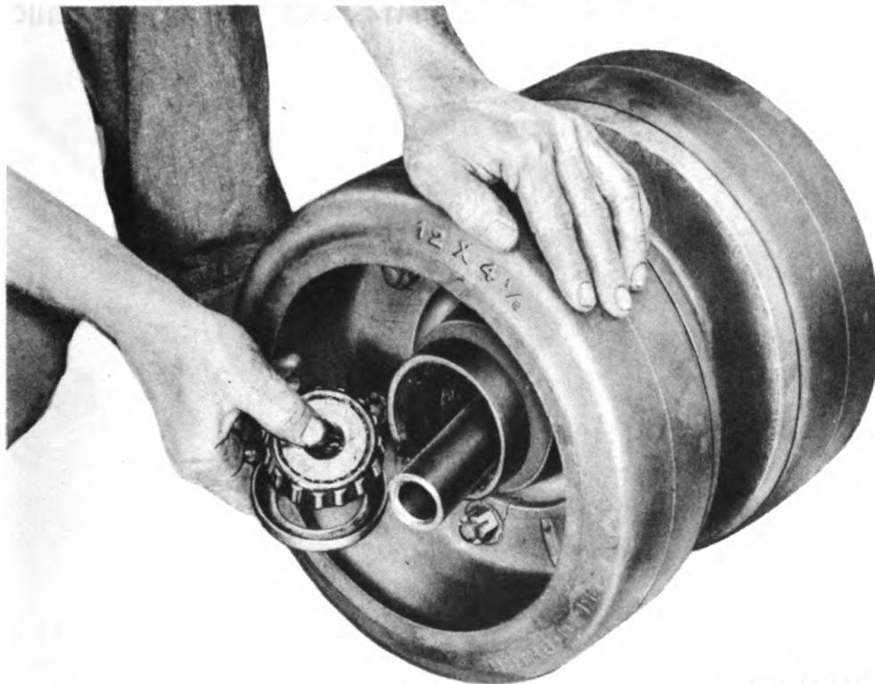
Figure 78 – Bogie Roller Bearings – Removal
