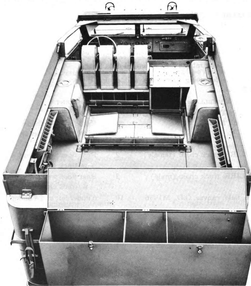
Figure 32 — Stowage Compartments — Open (M14)
