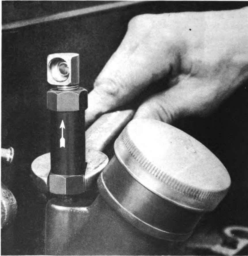
Figure 220 – Ventilator Metering Valve – Installation
