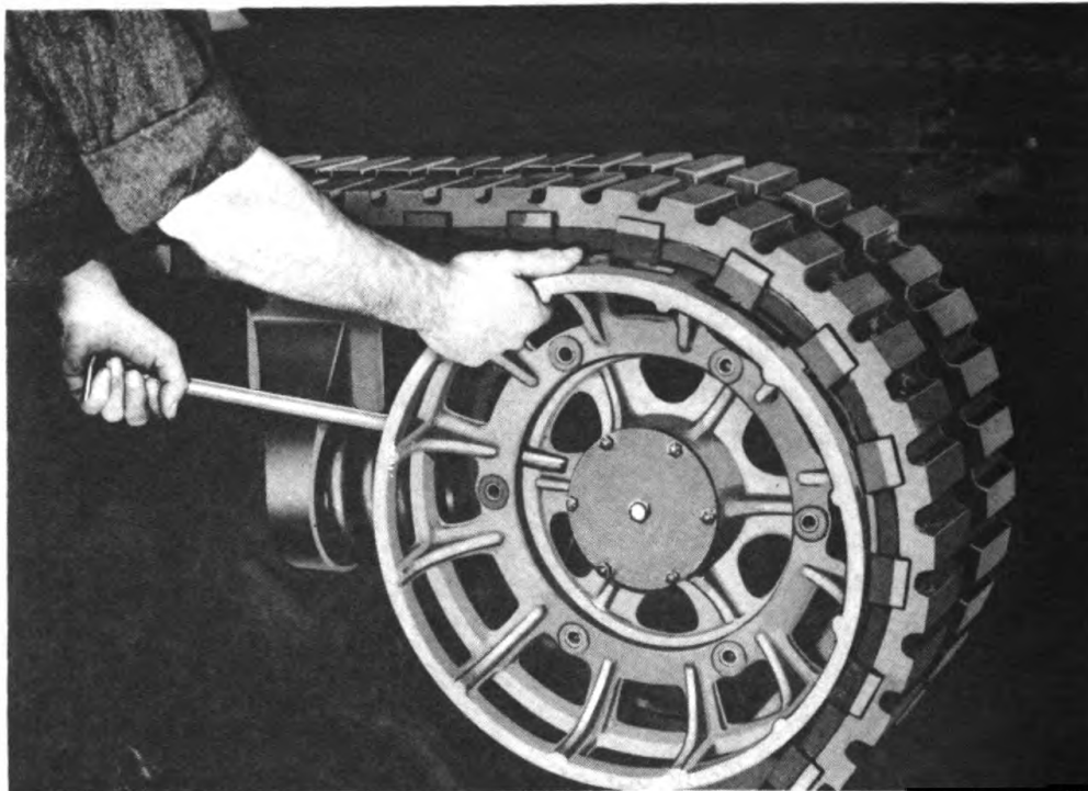
Figure 71 – Idler Flange – Removal
