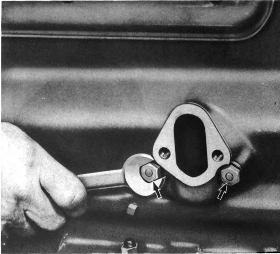
Figure 236 – Adapter to Crankcase Cap Screws – Removal
