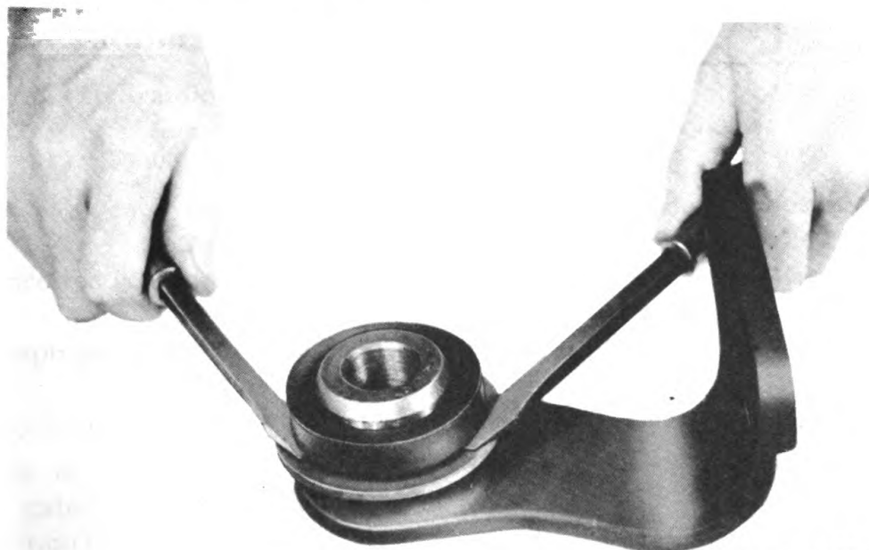
Digitized by Google Figure 97 – Upper Roller Seal – Removal Original from UNIVERSITY OF CALIFORNIA
