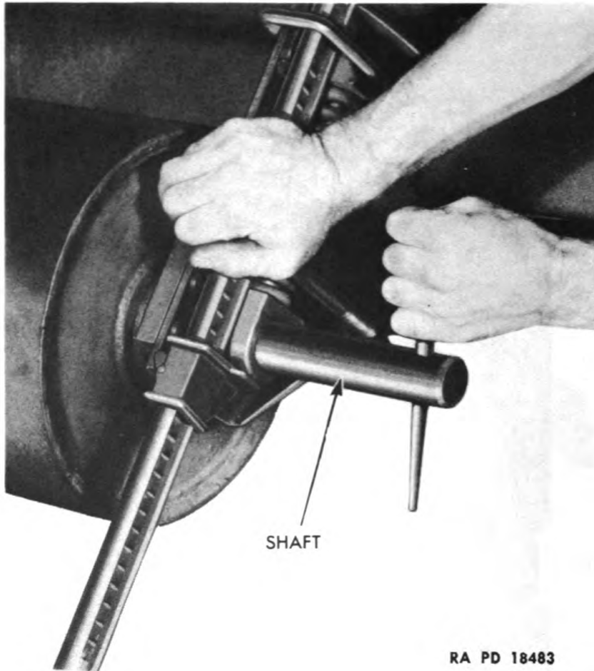
Figure 230 – Roller Shaft – Removal
