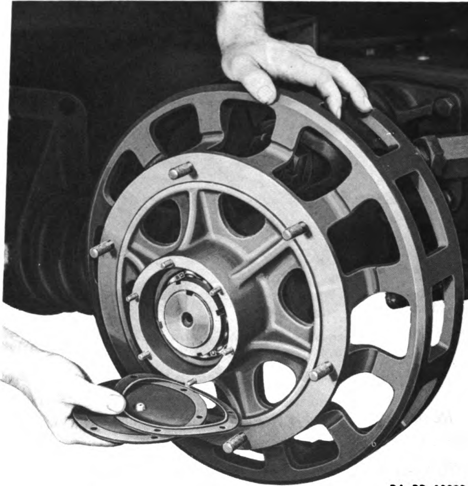
Figure 86 – Idler Cap and Gasket – Removal
