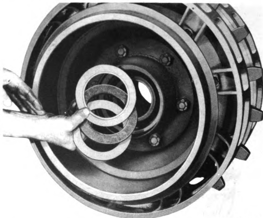
Figure 283 – Drive Sprocket Grease Seal – Removal
