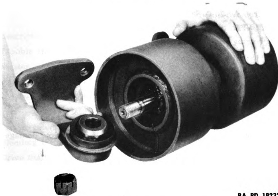
Figure 96 – Upper Roller Bracket – Removal
