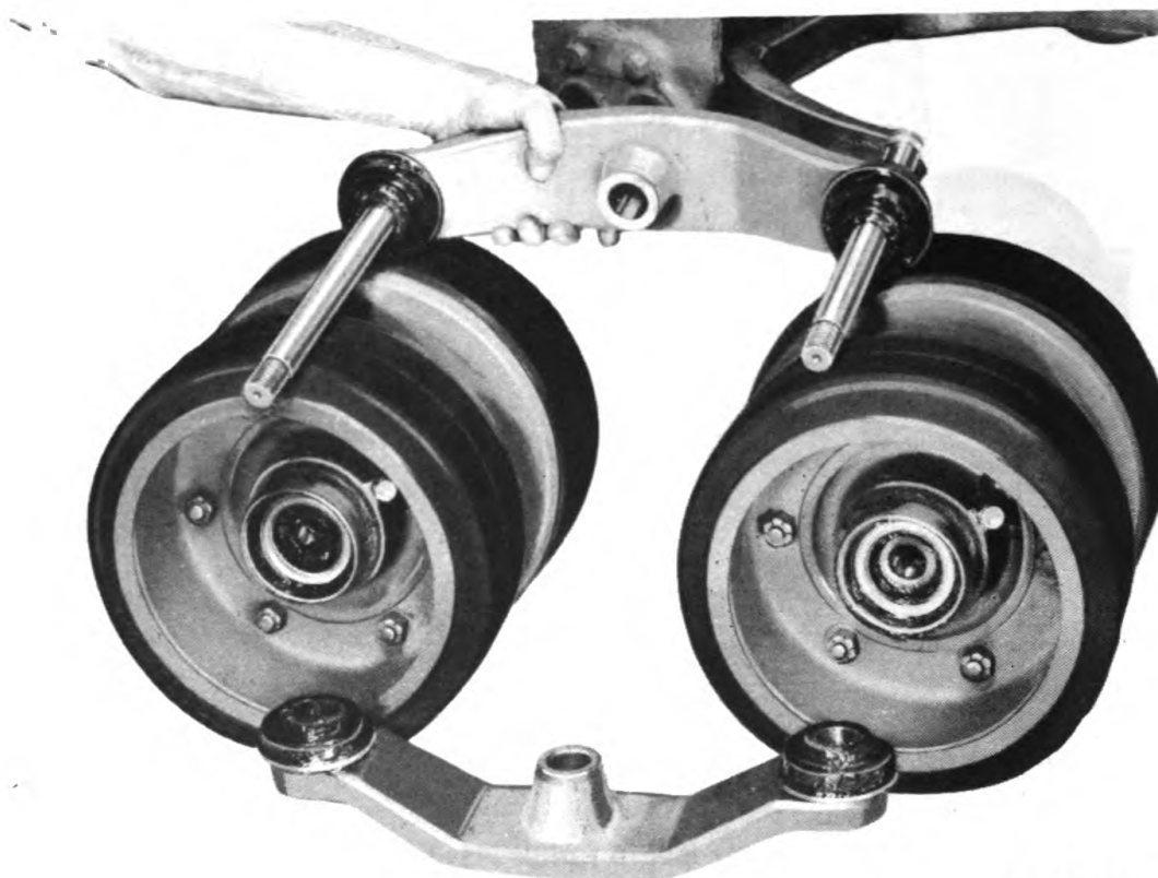
Figure 77 – Bogie Inner Frame – Removal
