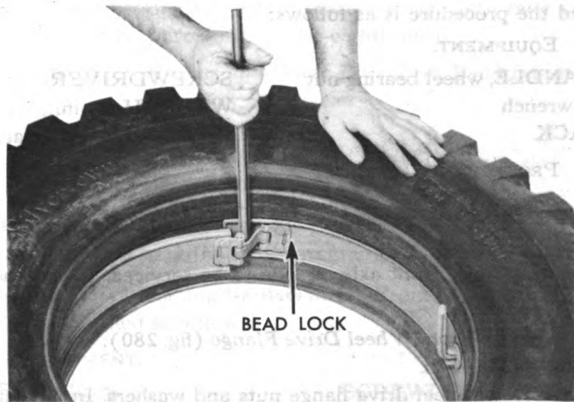
Figure 277 — Removing Tire from Rim
