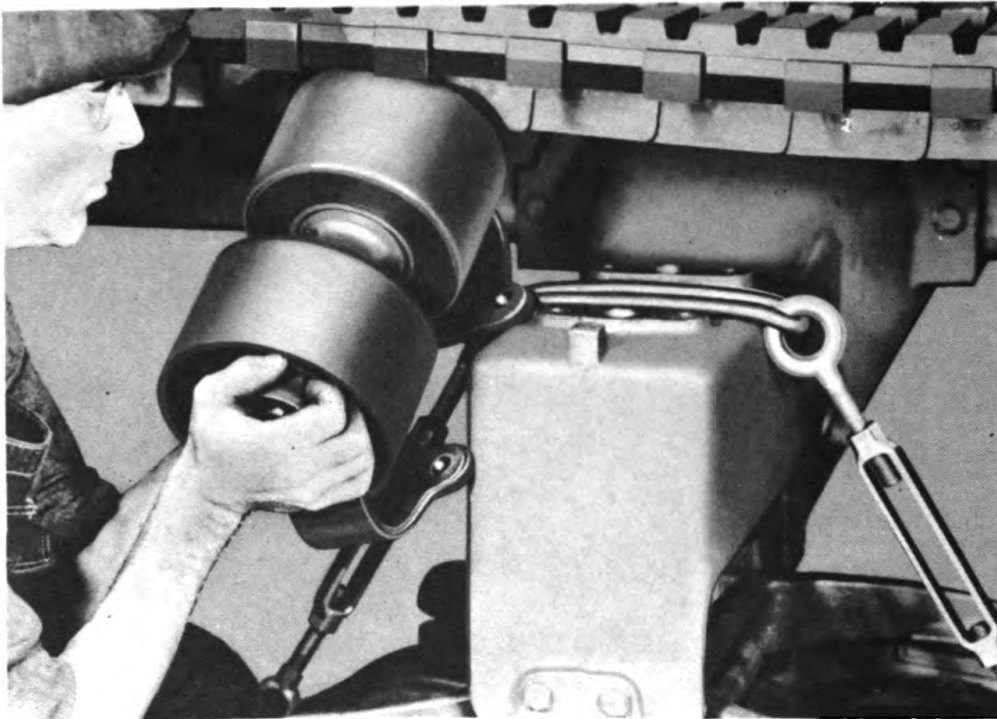
Figure 70 – Upper Rollers – Removal
