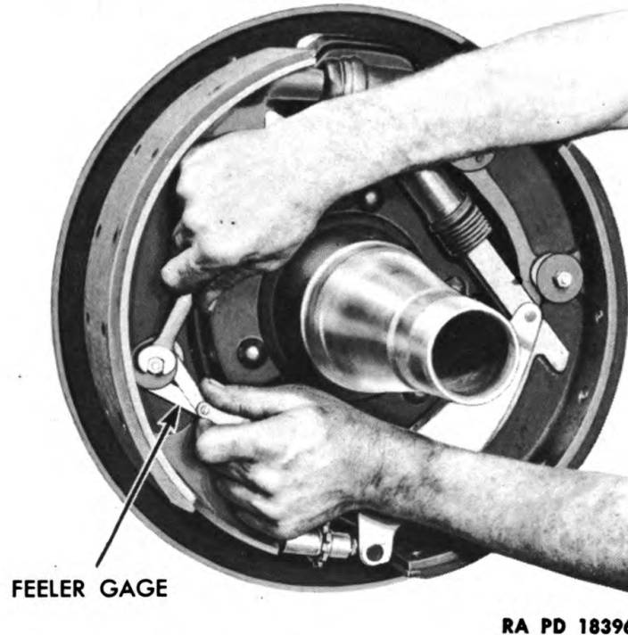
Figure 129 – Brake Shoe Guide Bolt Adjustment
