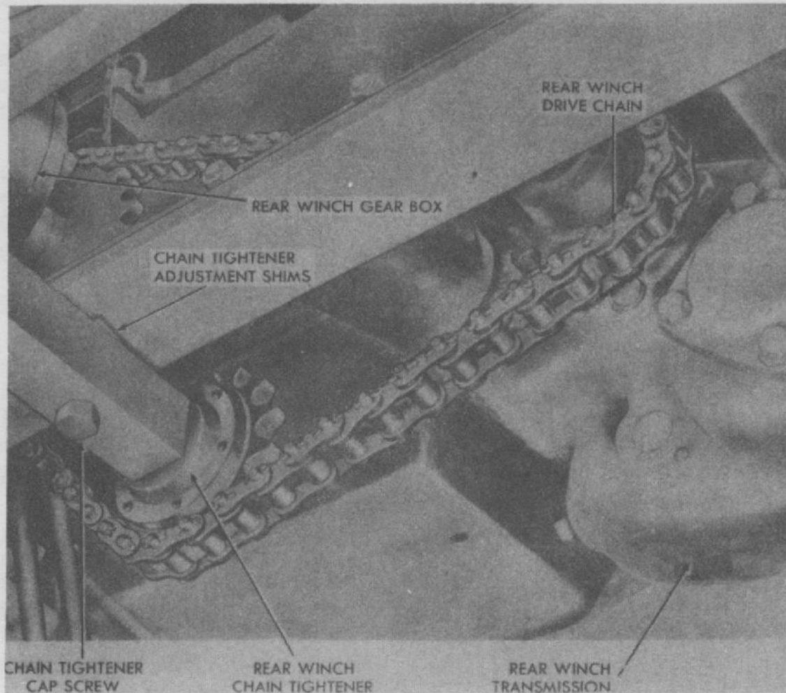
Figure 176—Rear Winch Drive Chain Replacement
