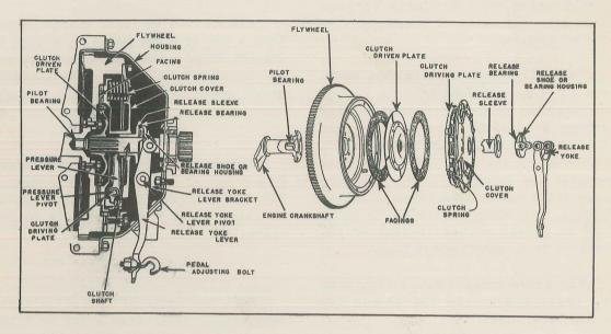
The clutch is probably the most used unit on a motor vehicle. Each time the operator changes to a different gear, the clutch must be disengaged and then engaged. Each time the clutch is released or engaged there is a considerable amount of friction between the clutch driving disk and the driven plate, which is usually fastened to or part of the flywheel. This friction generates heat, and the clutch usually is designed so that heat can be quickly and equally distributed to prevent spot burning.
