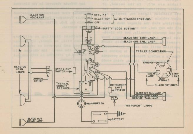
Tail lamps are equipped with a ruby red filter, stop lamps with an amber filter, while blackout lamps on the front of the vehicle have blue filters. In repairing these lamps, care must be exercised to see that the proper color filter is used for each lamp, that all rubber gaskets and seals are flat and in place, and that the cover retaining screws are tight.
