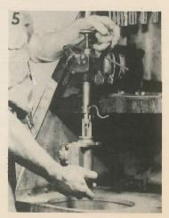
Honing the cylinder places a sharp edge around the by-pass port. This should be burred off to prevent it from wearing the piston rubber cup. Special pliers are available, having a sharp dowel slightly smaller than the port. This dowel is inserted in the port, and a slight pressure applied to remove the sharp edge.
