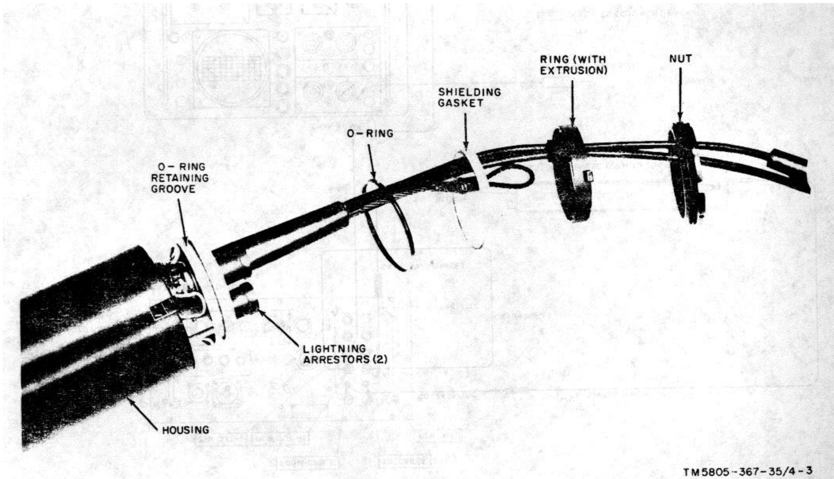
Figure 3-2. Restorer, Pulse Form TD-206/G, exploded view.
