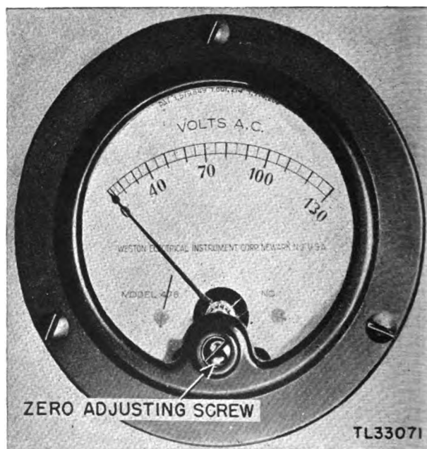
Figure 11. Meter zero-adjustment screw.
