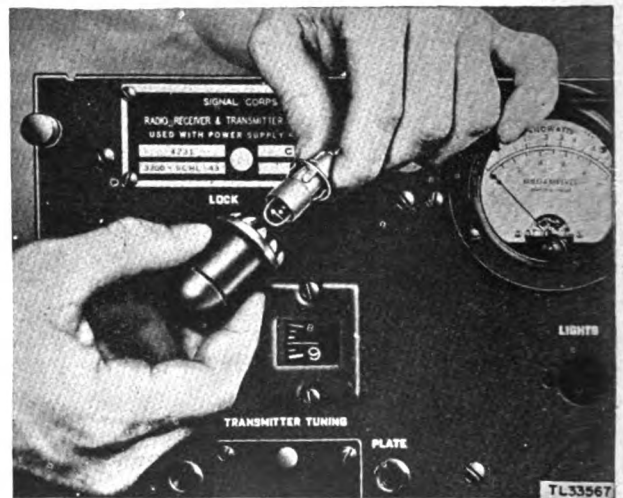
Figure 8. Replacing pilot lamp.
