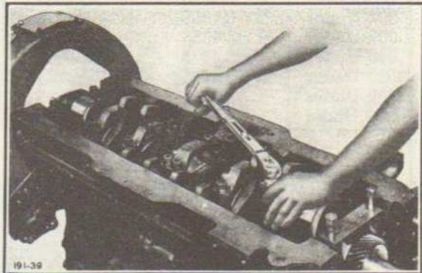
Fig. 80—Tightening Main Bearing Capscrews (Tool—J. H. Williams Part No. S-57)
