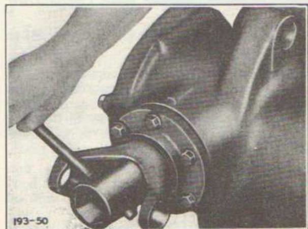
Fig. 13—Removing Rear Flange Nut (Tools—Snap-On-Tool Part No's. L-643 & L-53)
