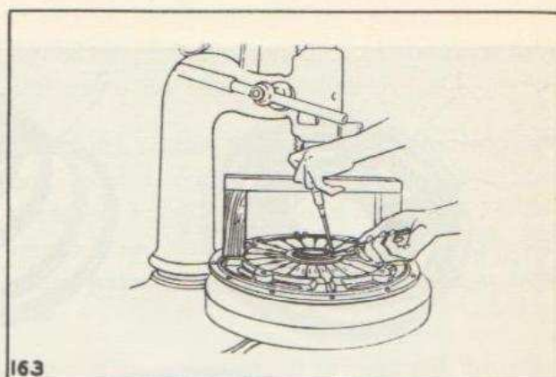
Fig. 7—Removing Snap Ring (Tool—Federal Stock No. 41-P-1993)
