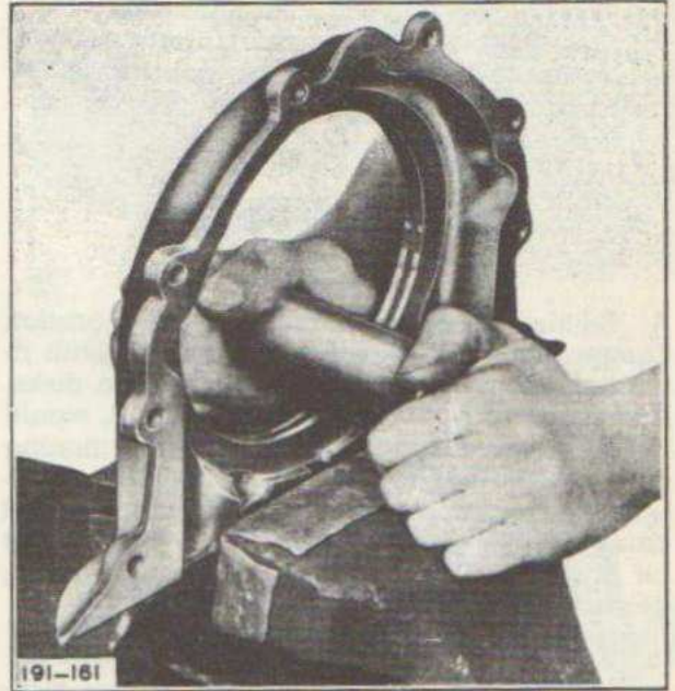
Fig. 83—View Showing Method for Sizing Lead, Oil-sealing Ring
