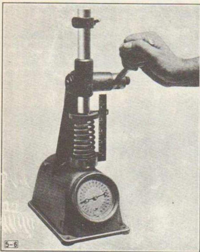
Fig. 103—Testing Valve Spring (Tool—Federal Stock No. 41-T-1600)
