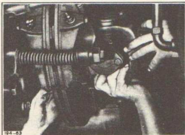
Fig. 88—Installing Propeller Shaft to Forward Rear Axle
