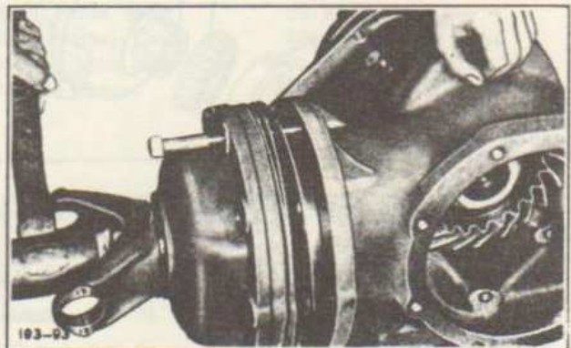
Fig. 64—Re-installing Bevel Pinion Assembly
