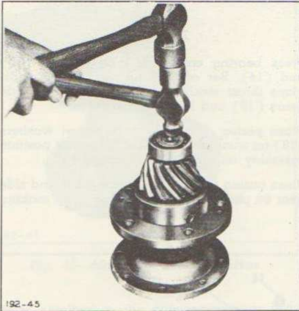
Fig. 41—Peening Shaft to Retain Bearing
