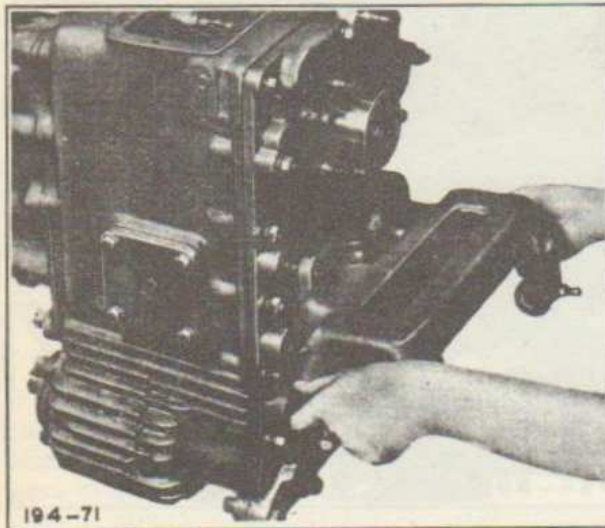
Fig. 14—Removing Countershaft Rear Bearing Cover and Brake Bracket
