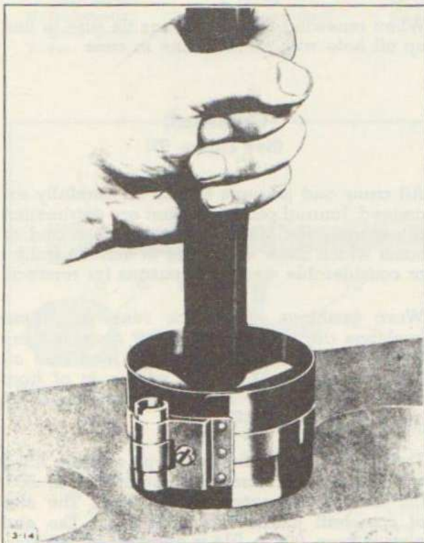
Fig. 93—Inserting Piston Using Ring Compressor (Tool—Federal Stock No. 41-C-2550)
