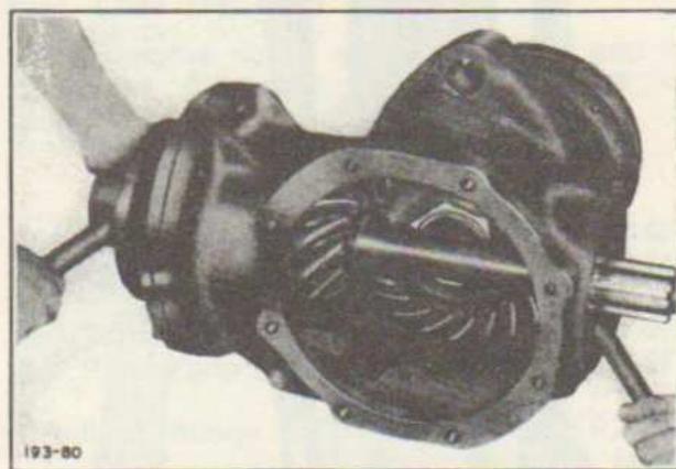
Fig. 48—Applying Pressure to Bevel Gears
