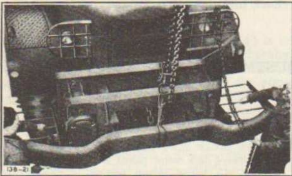
Fig. 4—View Showing Bumper Being Removed
