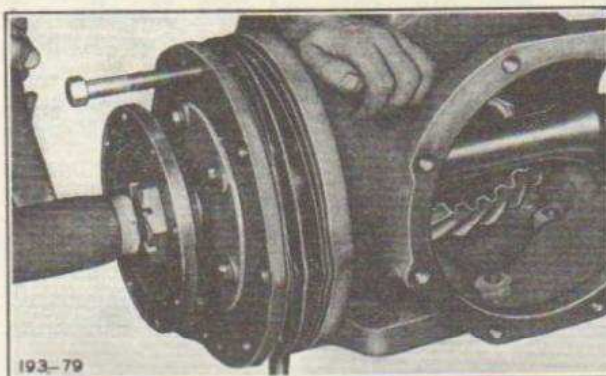
Fig. 47—Installing Bevel Pinion Assembly
