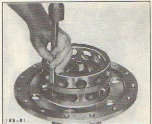
Fig. 50—Installing Outer Ring
