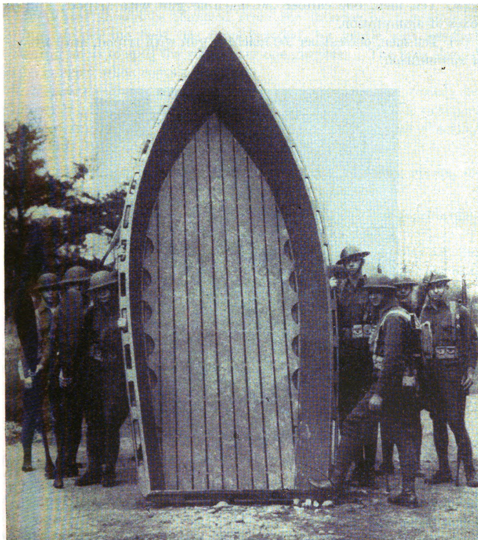
FIGURE 2.—Interior view of assault boat. (The carrying rail does not extend across the transom in the newer model.)
