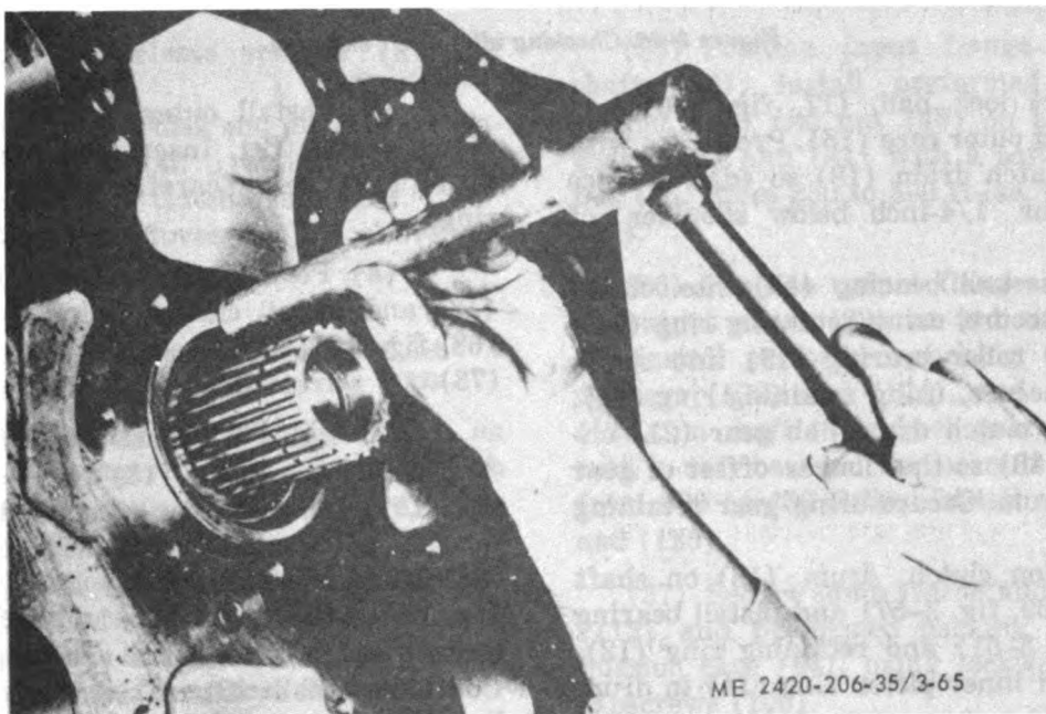
Figure 3-65. Installing tapered roller bearing cup.
