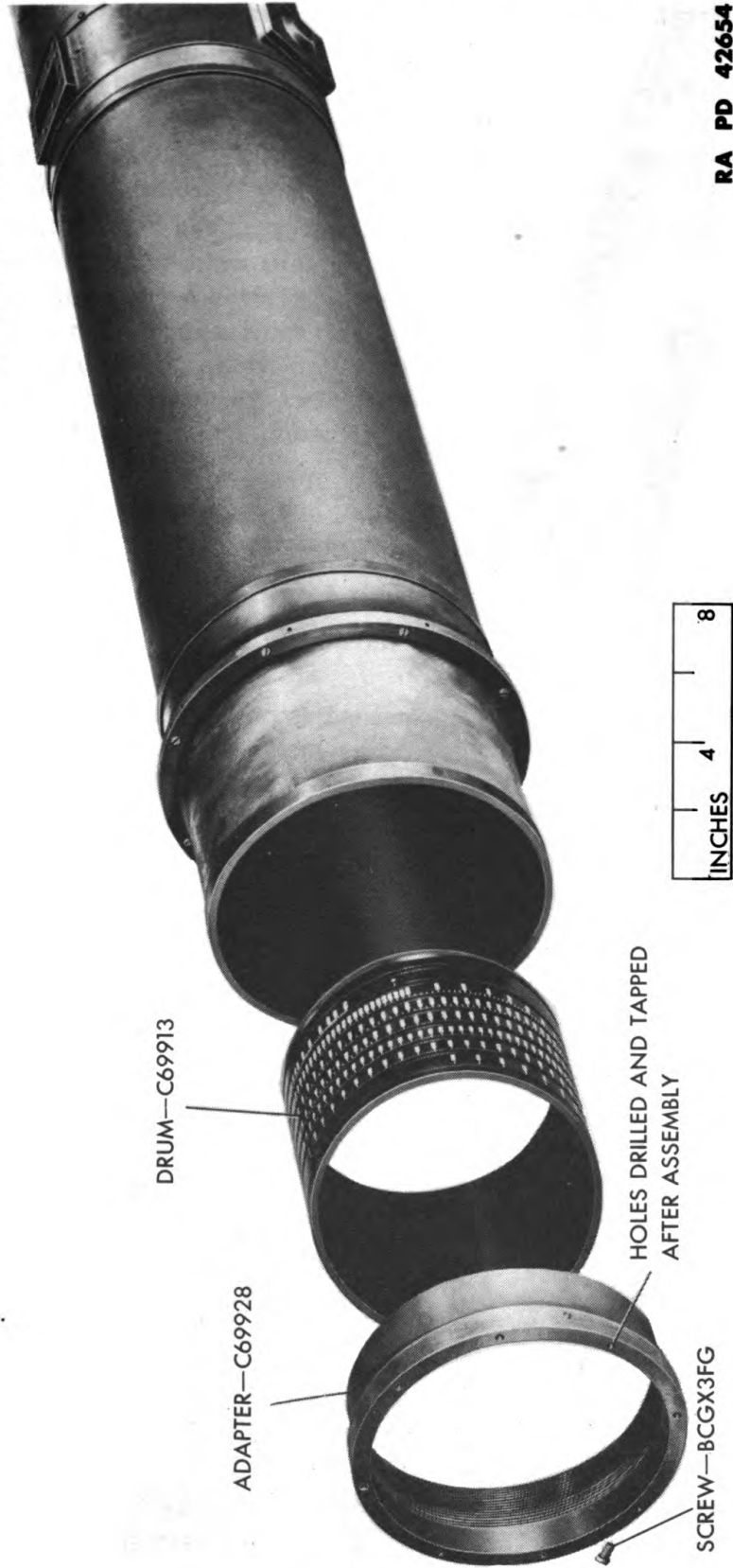
Figure 137 — Removal of End Adapter and Inner Tube Bearing Roller Assemblies
