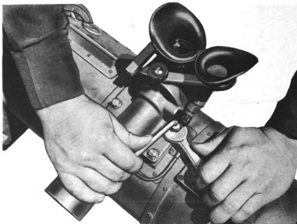
Figure 159 — Adjusting Alinement of M7 Telescope
