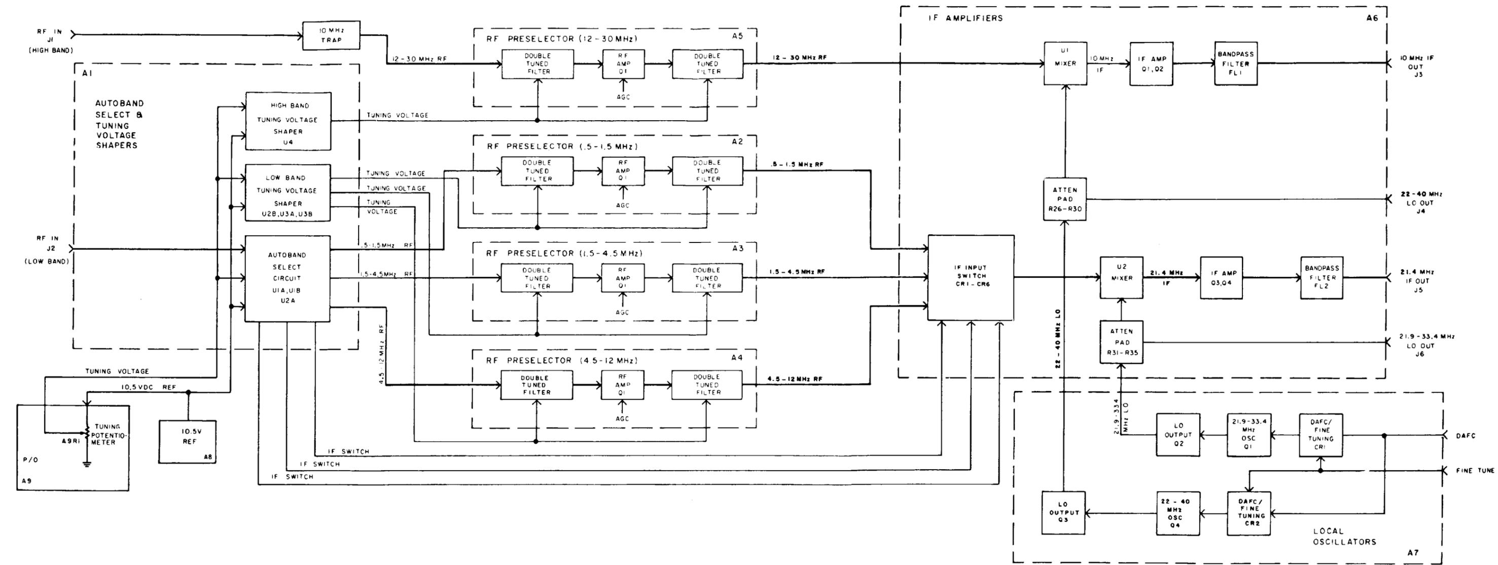
Figure 3-1. Type WJ-9120 Functional Block Diagram
