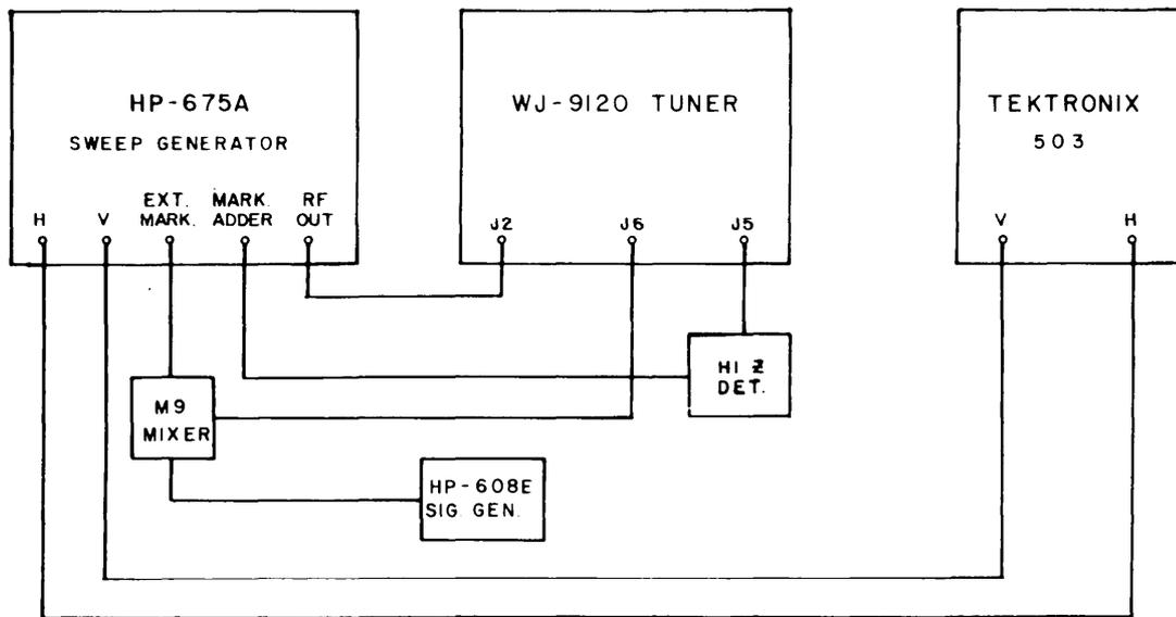
Figure 4-10. Equipment Connections, Low Band RF Preselectors
