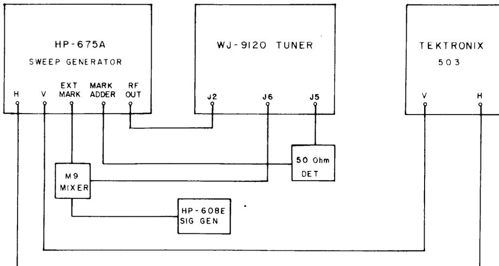
Figure 4-5. Equipment Connection, Gain Measurement
