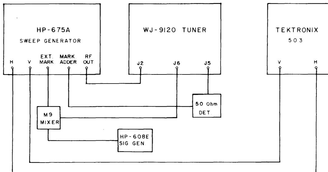
Figure 4-4. Equipment Connections, Gain Measurement
