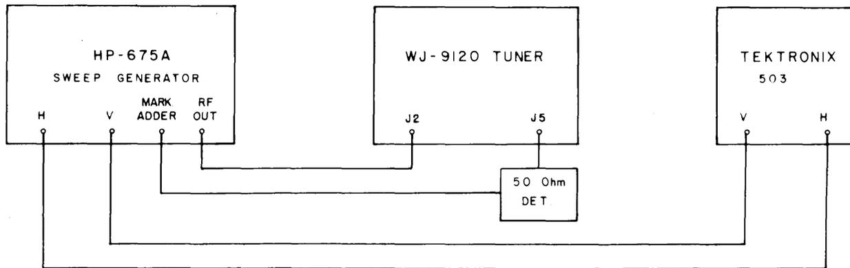
Figure 4-16. Equipment Connection, Overall Gain Adjustment (Low Band)
