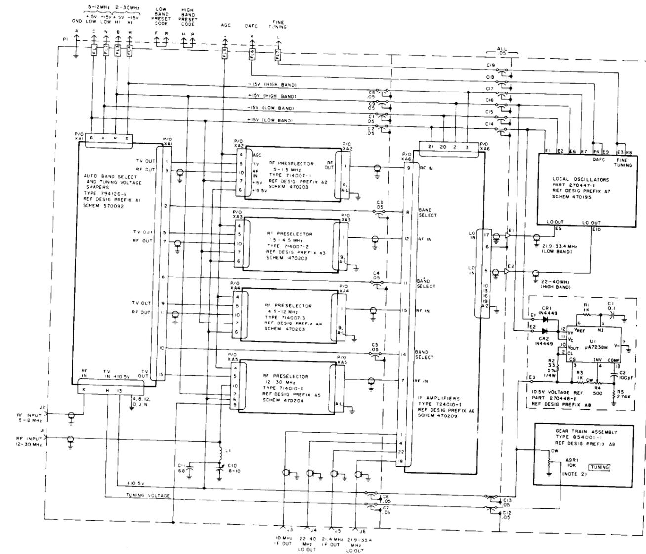
Figure 6-6. Type WJ-120 HF Tuner, Schematic Diagram 570098
