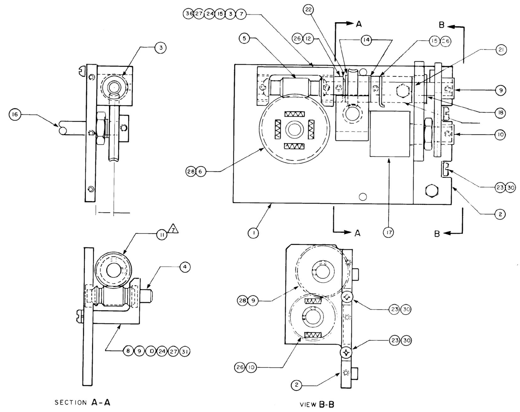
Figure 5-11. Type 854001-1 Tuning Drive Assembly (A8), Location of Components.
