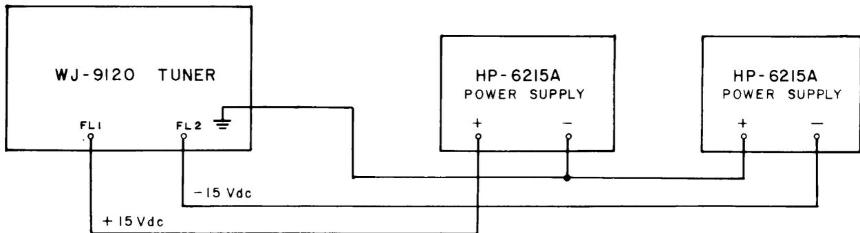
Figure 4-2. Power Connection, Low Band Operation
