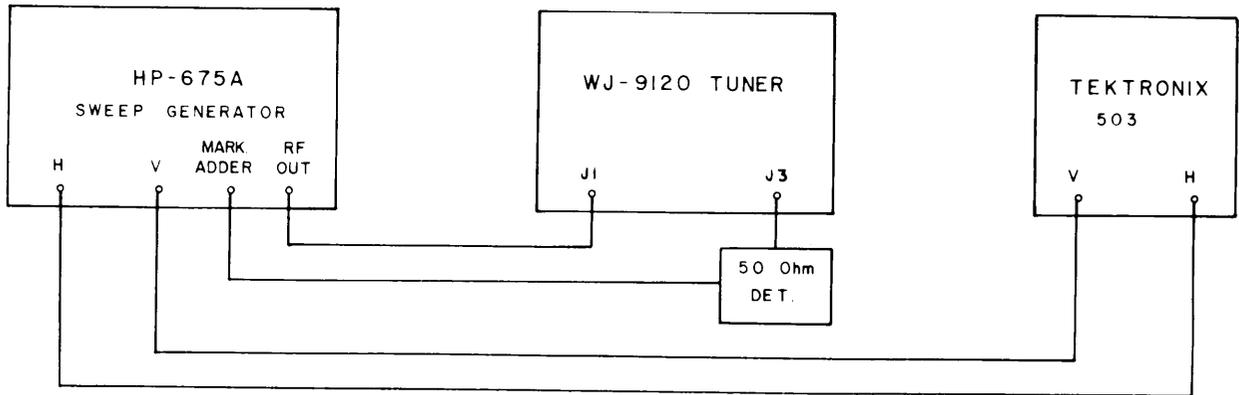
Figure 4-17. Equipment Connection, Overall Gain Adjustment (Highland)
