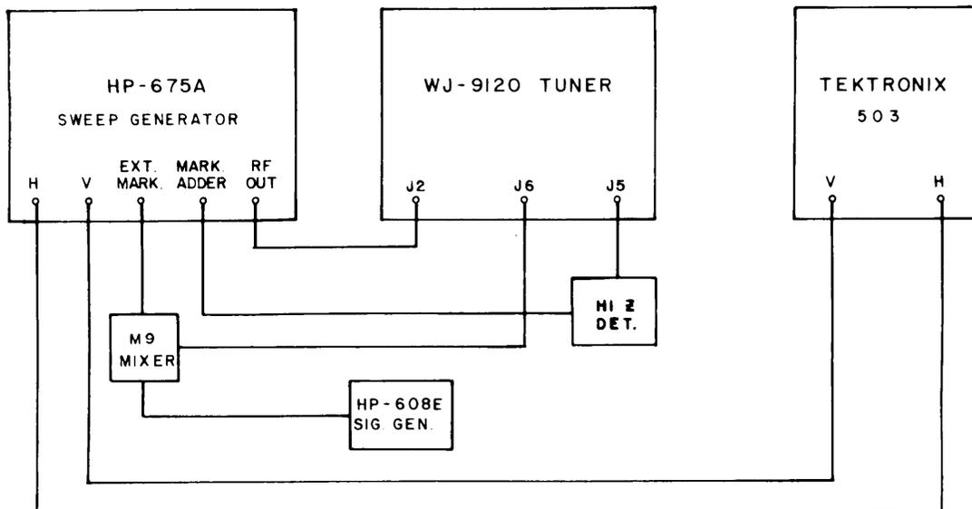
Figure 4-14. Equipment Connections, 12-30 MHz Preselector
