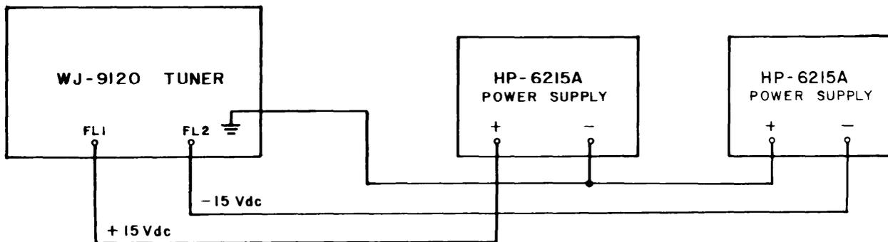
Figure 4-3. Power Connection, High Band Operation
