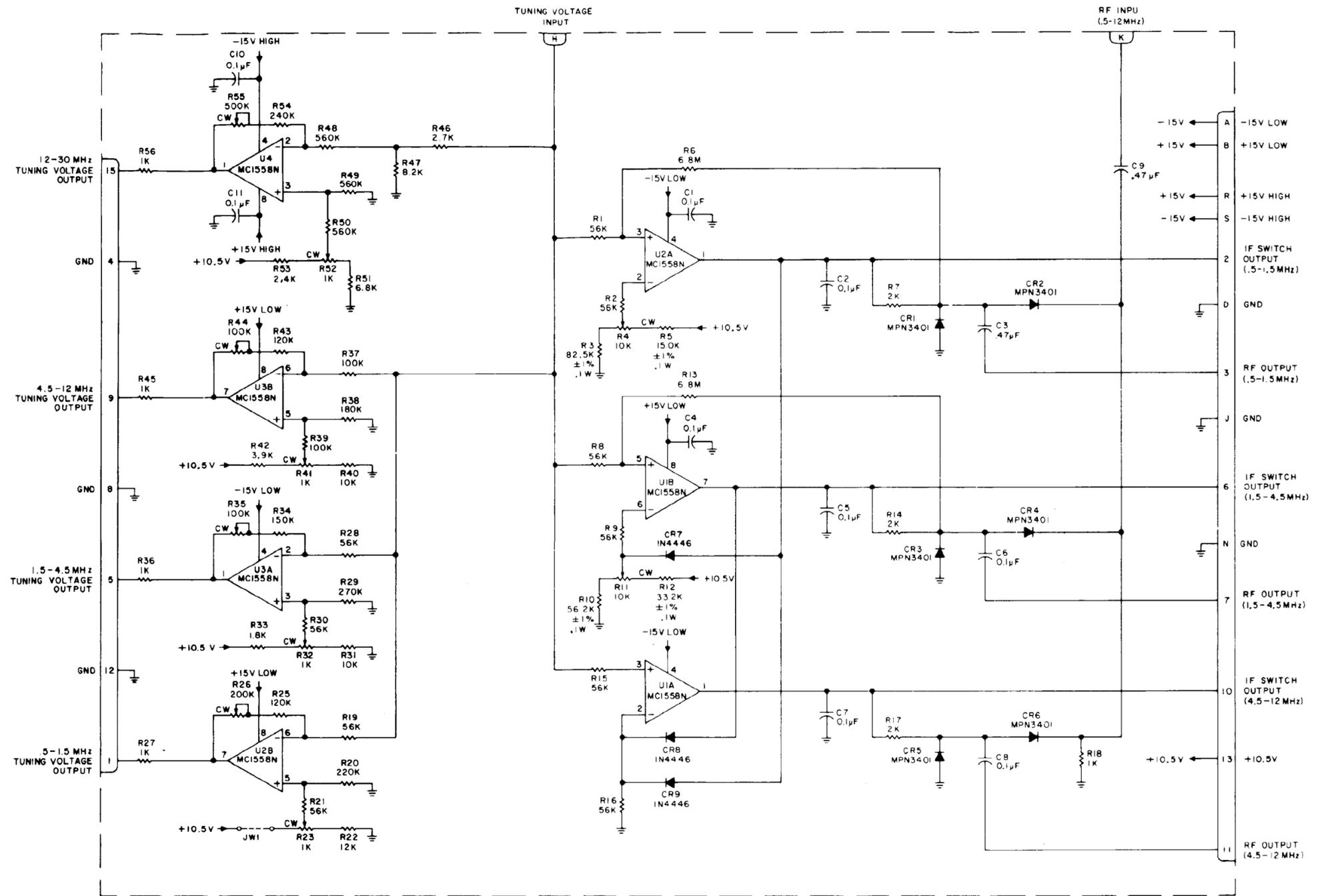
Figure 6-1. Type 794126-1 Auto Band Select and Tuning Voltage Shapers (A1), Schematic Diagram 570092
