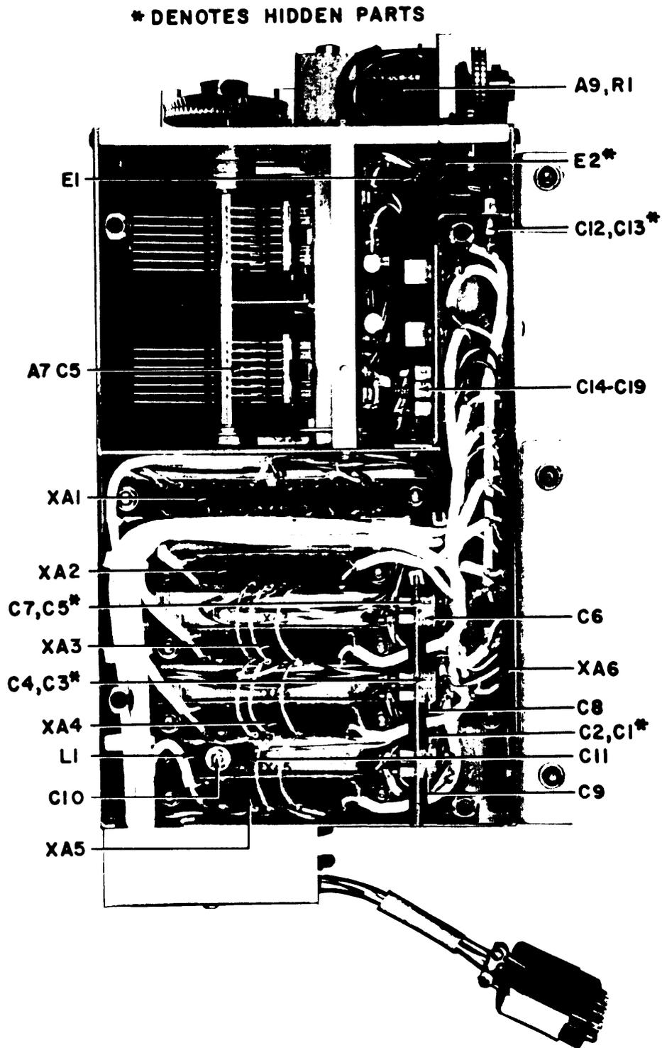
Figure 5-4. Type WJ-9120 0.5-30 MHz Tuner Assembly, Bottom View, Location of Components
