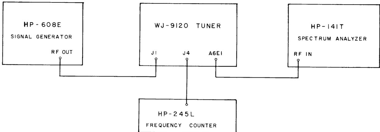
Figure 4-18. Equipment Connection, 10 MHz Trap Adjustment
