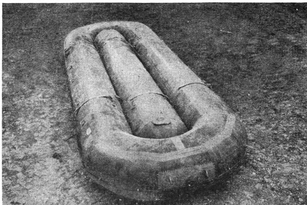
FIGURE 2.—12-ton pneumatic float.
