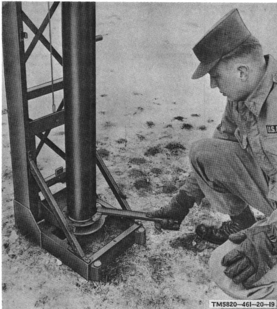
Figure 3-9. Rotating base of Mast AB-577/GRC to change azimuth of antenna on top of mast.
