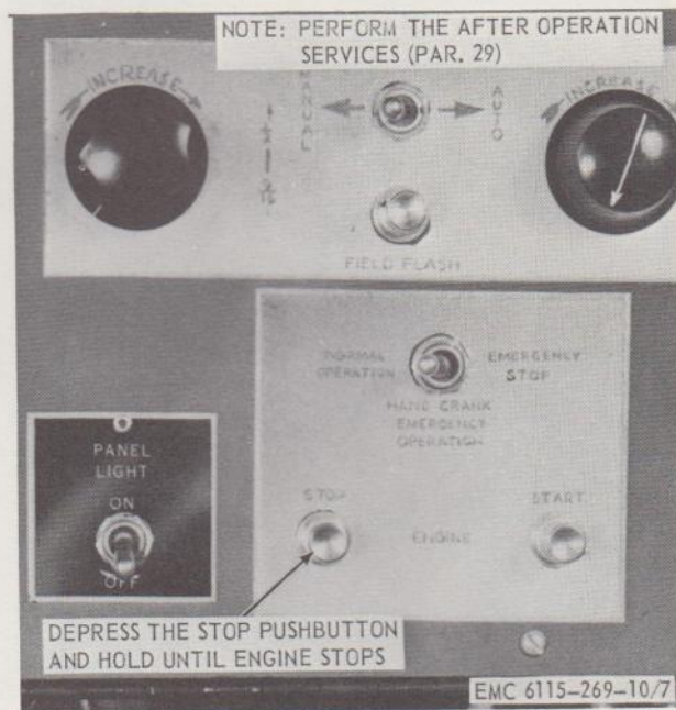
Figure 7. Engine stopping instructions.
