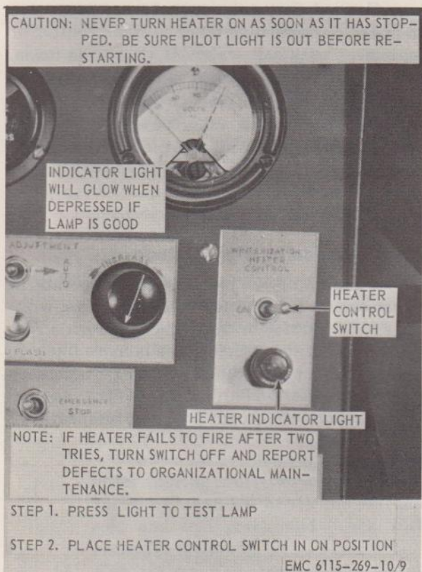
Figure 9. Winterization heater, starting.
