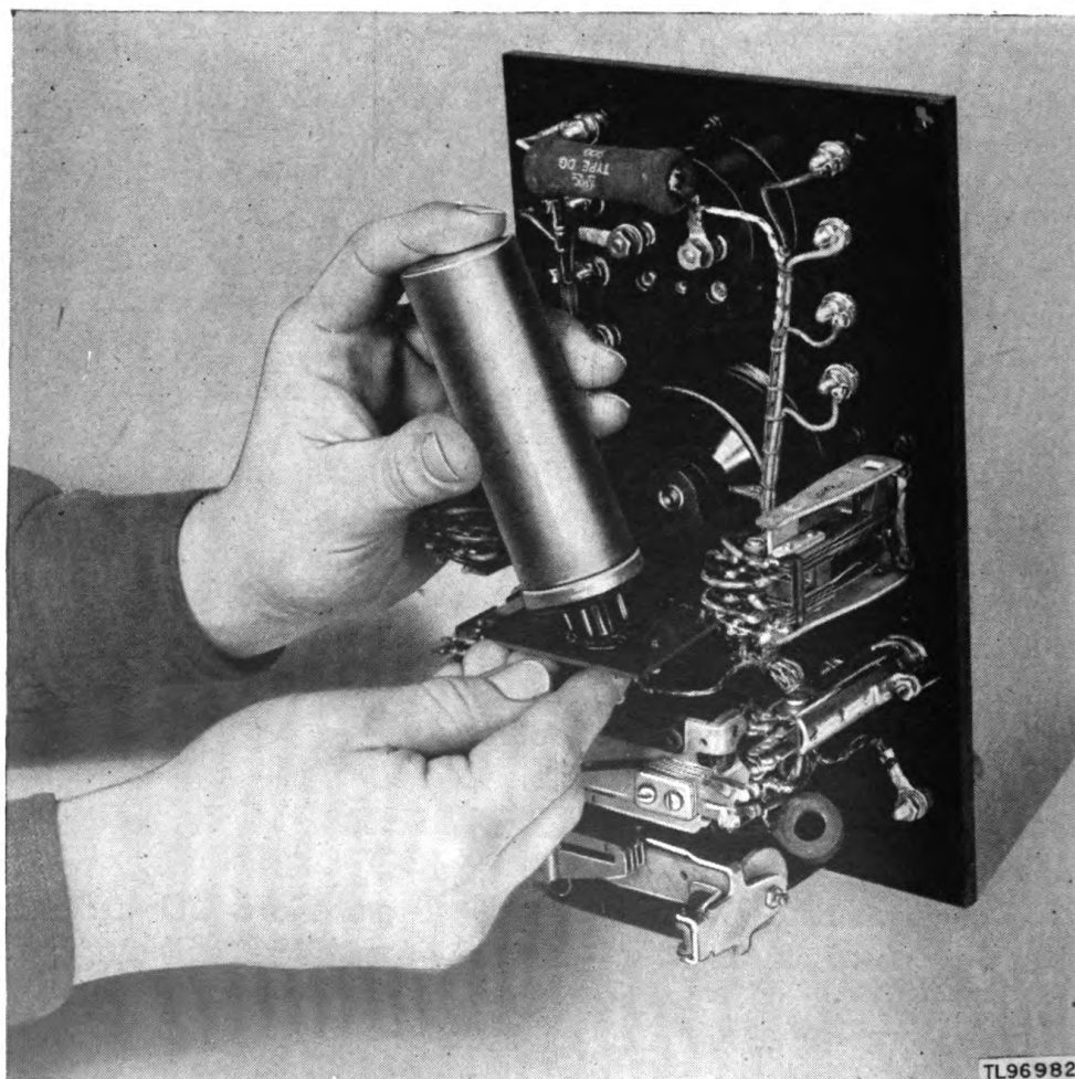
Figure 22. Replacing defective capacitor of Time Interval Device PH-103.
