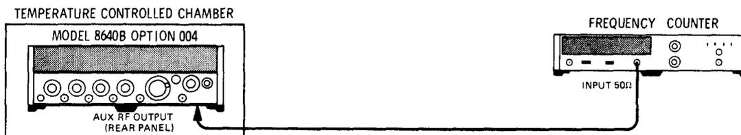
*Figure 4-2. Frequency Stability vs Temperature Test Setup*
