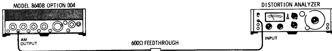
*Figure 4-17. Internal Modulation Oscillator Distortion Test Setup*
