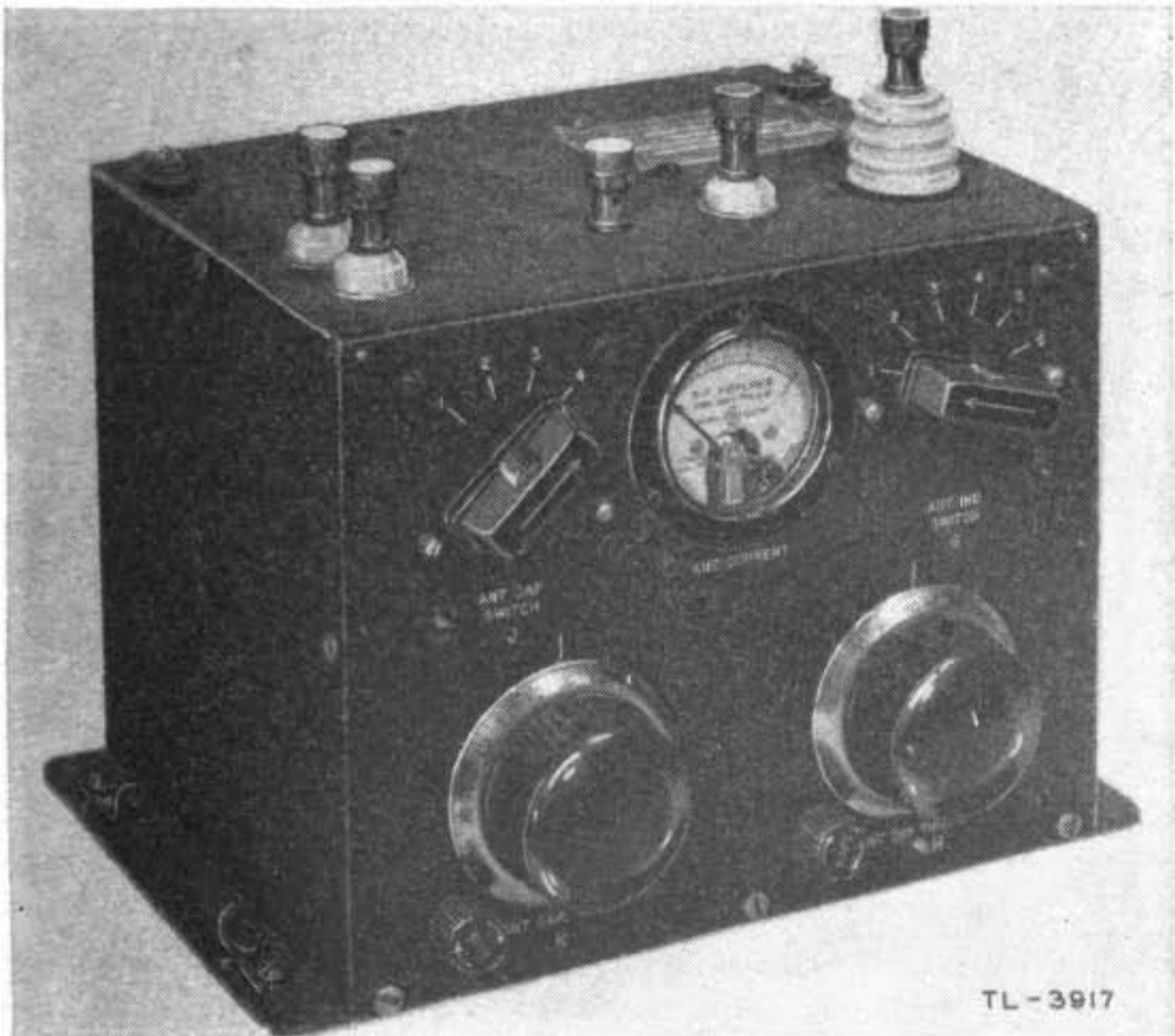
FIGURE 27.—Antenna tuning unit BC-AA-194—front view.
