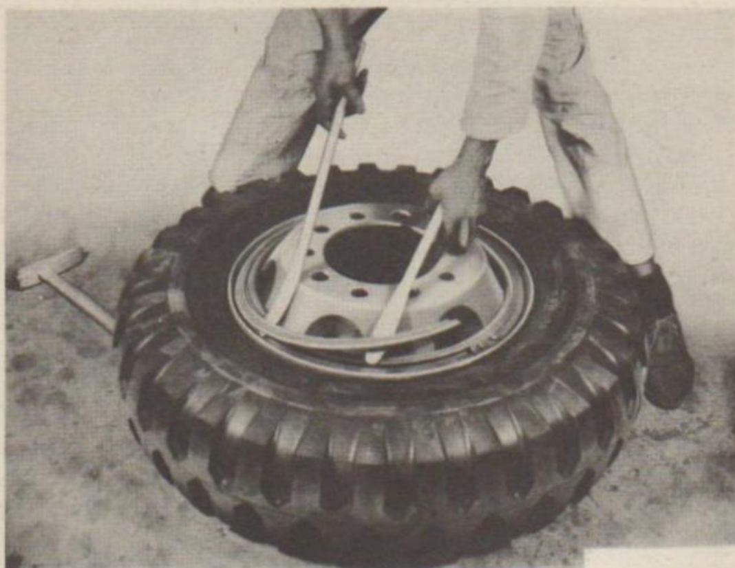
Figure 21—Removing Tire Lock Ring
