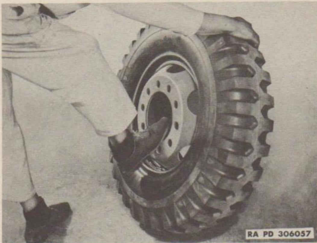
Figure 22—Removing Tire from Wheel
