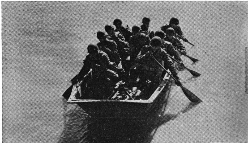
FIGURE 5.—Assault boat carrying 7-man heavy machine-gun squad, three-man engineer crew, heavy machine gun caliber .30, and 13 boxes of ammunition.
