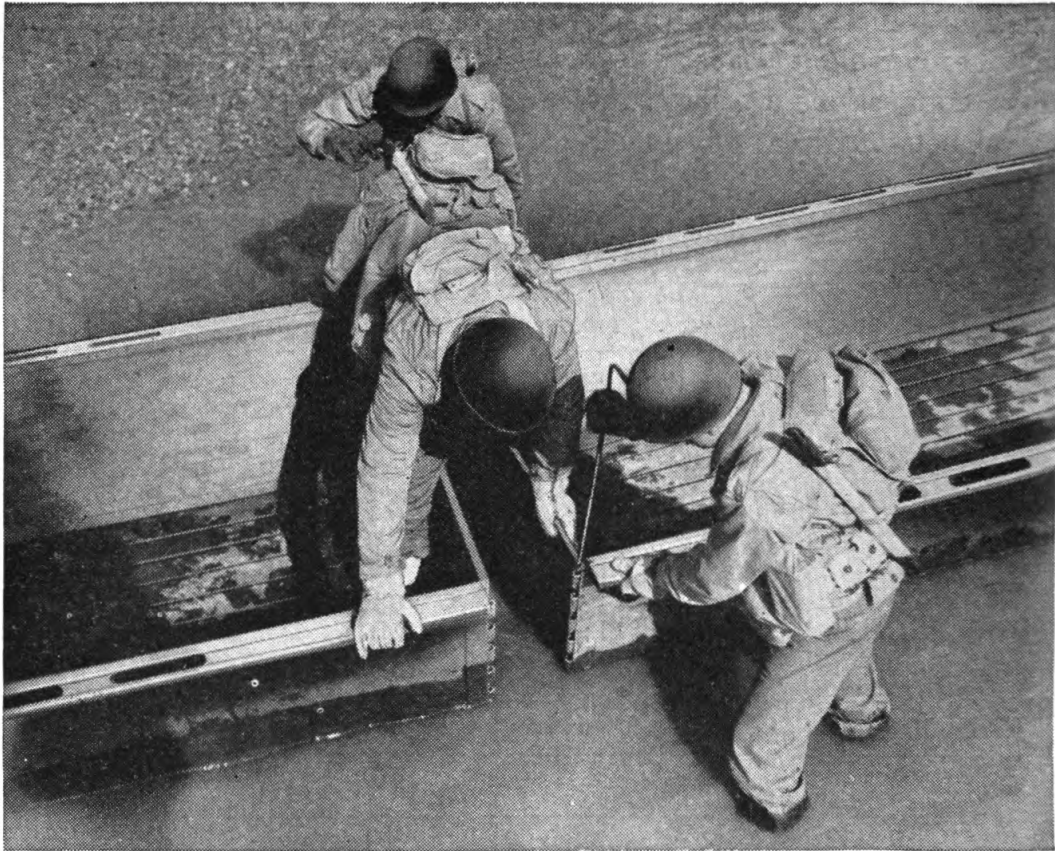
FIGURE 13.—Two assault boats M2 being joined stern-to-stern.
