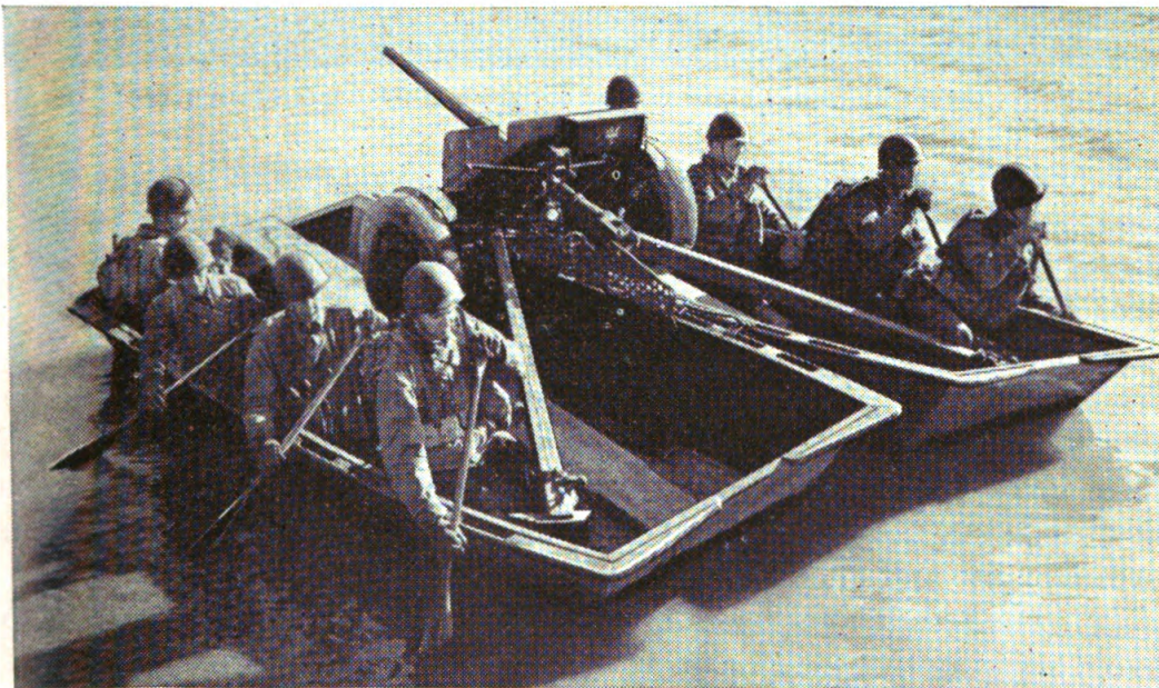
FIGURE 8.—Assault boats carrying five-man antitank gun crew, three-man engineer crew, 37-mm antitank gun, and 100 rounds of ammunition.
