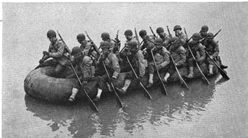
FIGURE 56.—Six-ton pneumatic float employed as an assault boat.
