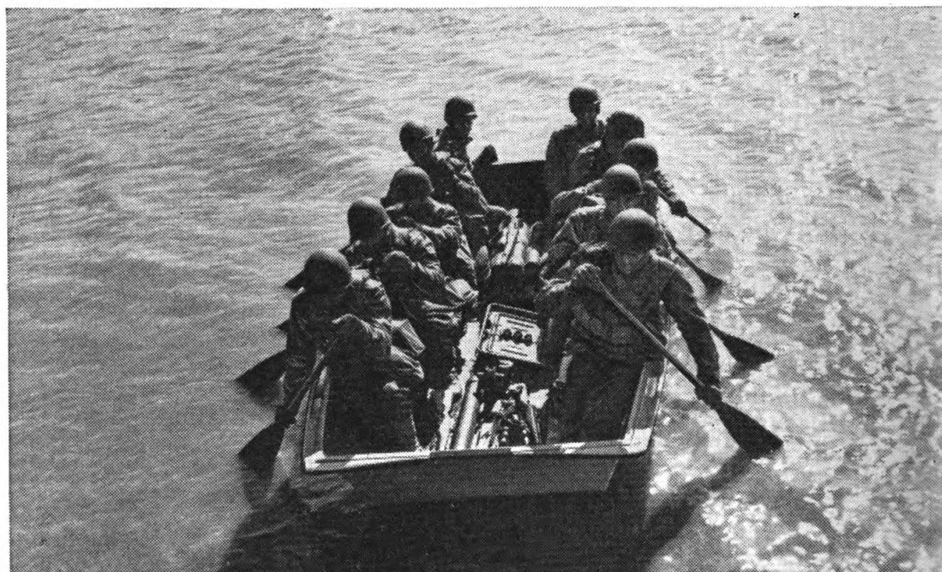
FIGURE 6.—Assault boat carrying seven-man 81-mm mortar squad, three-man engineer crew, 81-mm mortar, and 50 rounds of ammunition.
