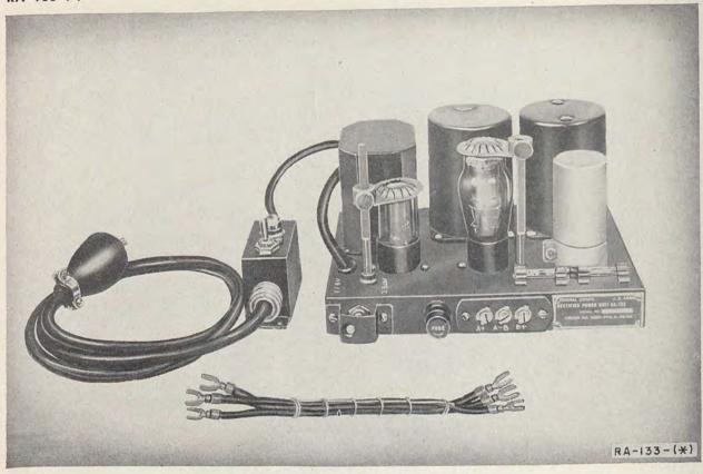
Figure 69. Rectifier Power Unit RA-133.
