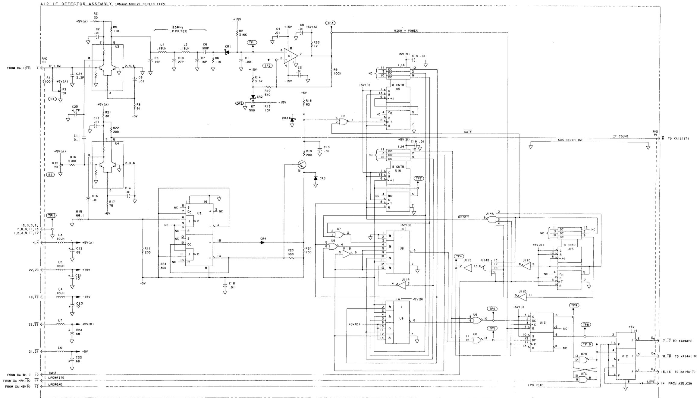
Figure 8-35. A12 IF Detector Assembly
