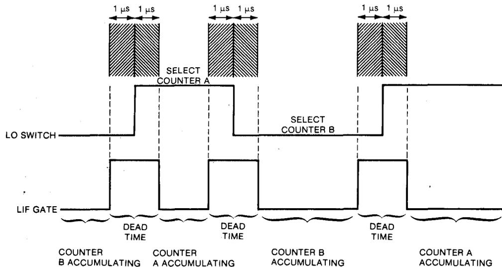
8-254. The dead time in the LIF GATE signal is generated by D flip-flops U9A, U9B, exclusive "OR" U6D, and D flip-flop U15A. The dead time is generated when U6D(11) goes high for two periods of the 1 MHz clock. With U6D(11), high, U10B is disabled and the prs clock at U10C(8) remains high. The reset input to U15A(1) is low during the prs generation so that U15A(5) is low. When the preset input U15A(4) goes low also, the output goes high for the time that the preset
