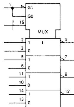
This quad two input multiplexer selects one of two word inputs and outputs the data the data when enabled. The level at pin 1 selects the input word. The outputs are LOW when pin 15 is LOW.
