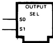
Output selector control block. This symbol is used with a block symbol having multiple outputs to form a decoder. The selection lines enable the output designated 0, 1, . . . .n of each block by means of a binary code where S0 is the least-significant digit. **If the 1 level of these lines is low, polarity indicators ( $\nabla$ ) will be used.**
