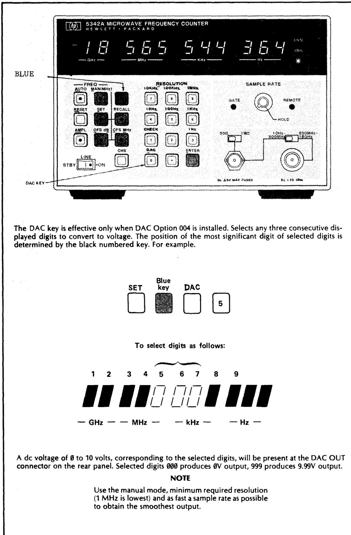
The DAC key is effective only when DAC Option 004 is installed. Selects any three consecutive displayed digits to convert to voltage. The position of the most significant digit of selected digits is determined by the black numbered key. For example.
