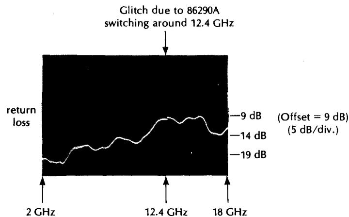
FOR AMPLITUDE OPTION, put the 5342A in diagnostic **mode 5** (press SET, SET 5) to prevent switching between the sampler input and the peak detector input. Measure SIR as described above and verify that for amplitude measurements, return loss is >9.5 dB for frequencies from 2 GHz-18 GHz. Next put the 5342A in AUTO and frequency only so that amplitude measurements are not made. Verify that the return loss is >3.5 dB for frequencies from 2-18 GHz (SIR <5:1).
