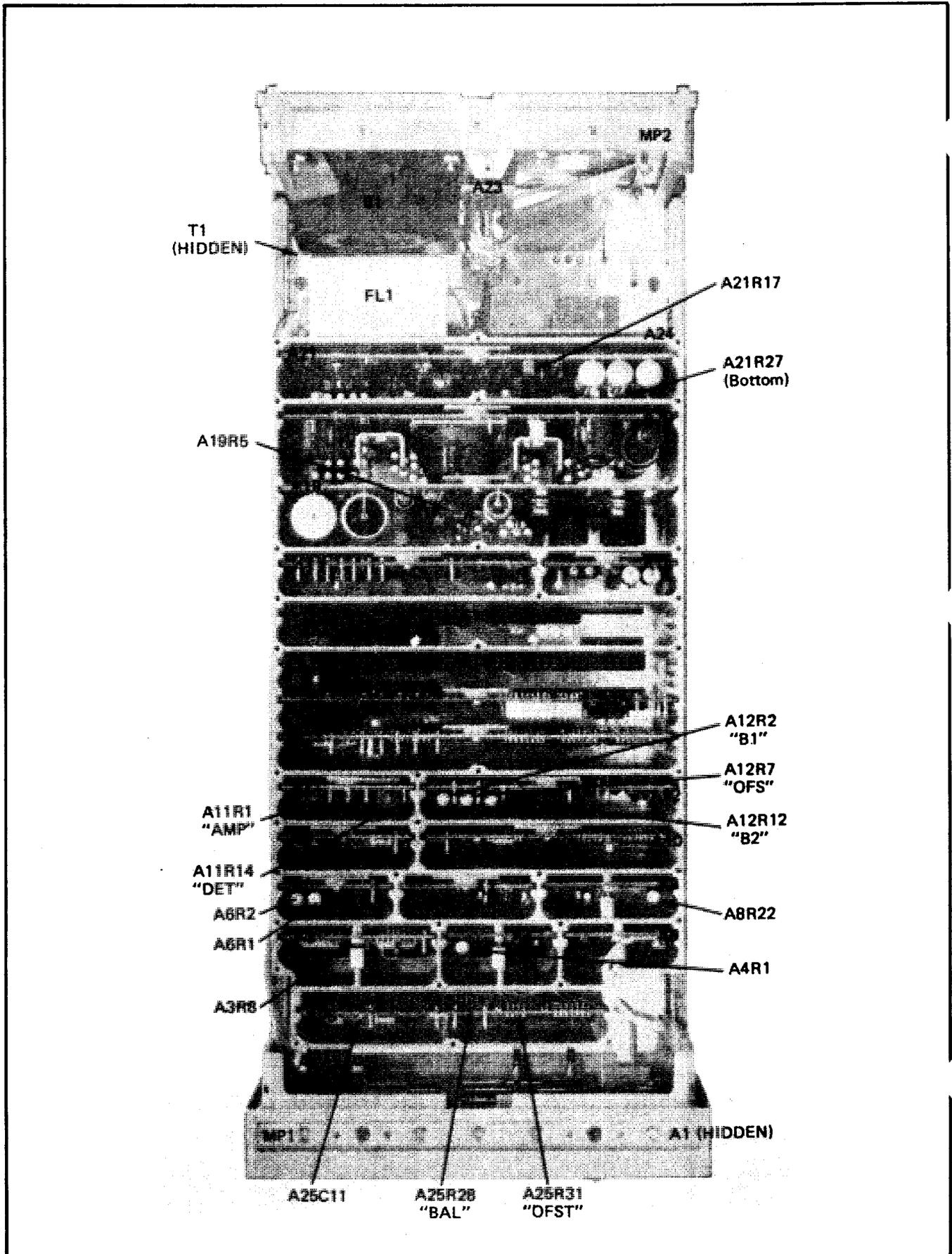
Figure 8-21. 5342A Top View (Assembly Locations and Adjustments)
