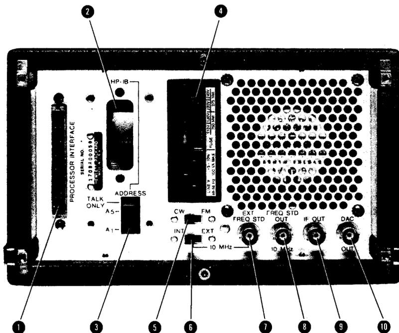
1. PROCESSOR INTERFACE connector A22#JI. Not used. This connector is part of cable # which is connected to A22 motherboard as an interface to the A14 Microprocessor address and data lines. This interface is provided for future use with companion instruments.
