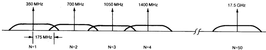
8-104. If there were gaps, then there could be a signal in the 0.5-18 GHz range which would not appear in the down converted IF. Thus, this signal, even if it were the largest, could not be measured.
