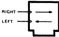
Shift register control block. These symbols are used with any array of flip-flop symbols to form a shift register. An active transition at the inputs causes left or right shifting as indicated.
