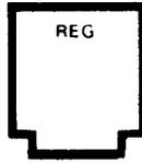
Register control block. This symbol is used with an associated array of flip-flop symbols to provide a point of placement for common function lines, such as a common clear.
