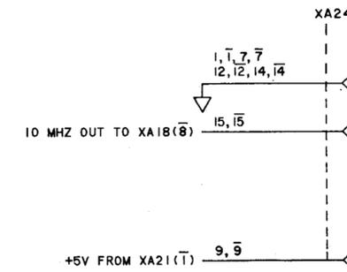
A24 STANDARD 10 MHZ OSCILLATOR ASSEMBLY (05341-60047) SERIES 1804
