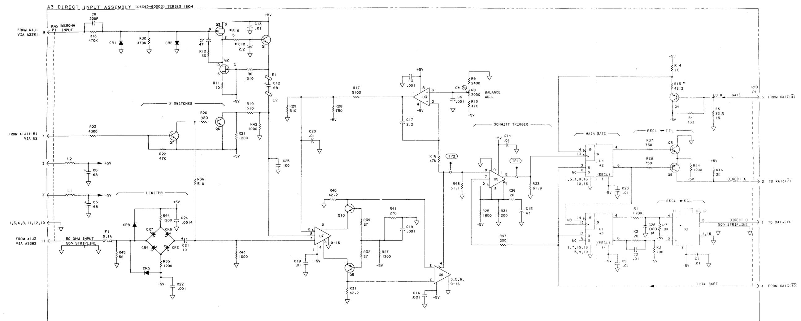
Figure 8-26. A3 Direct Count Amplifier Assembly
