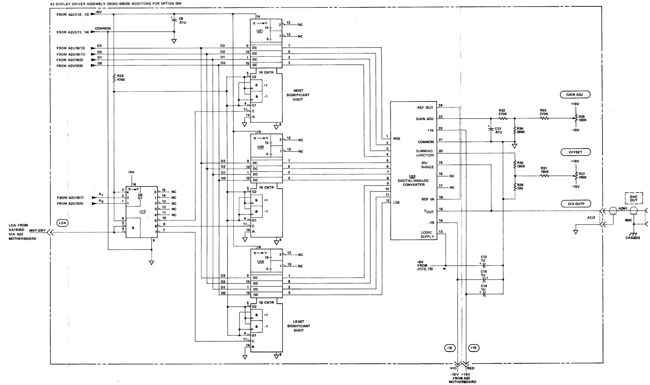
Figure 8-25. Option 004 Display Driver Additions on A2 Assembly
