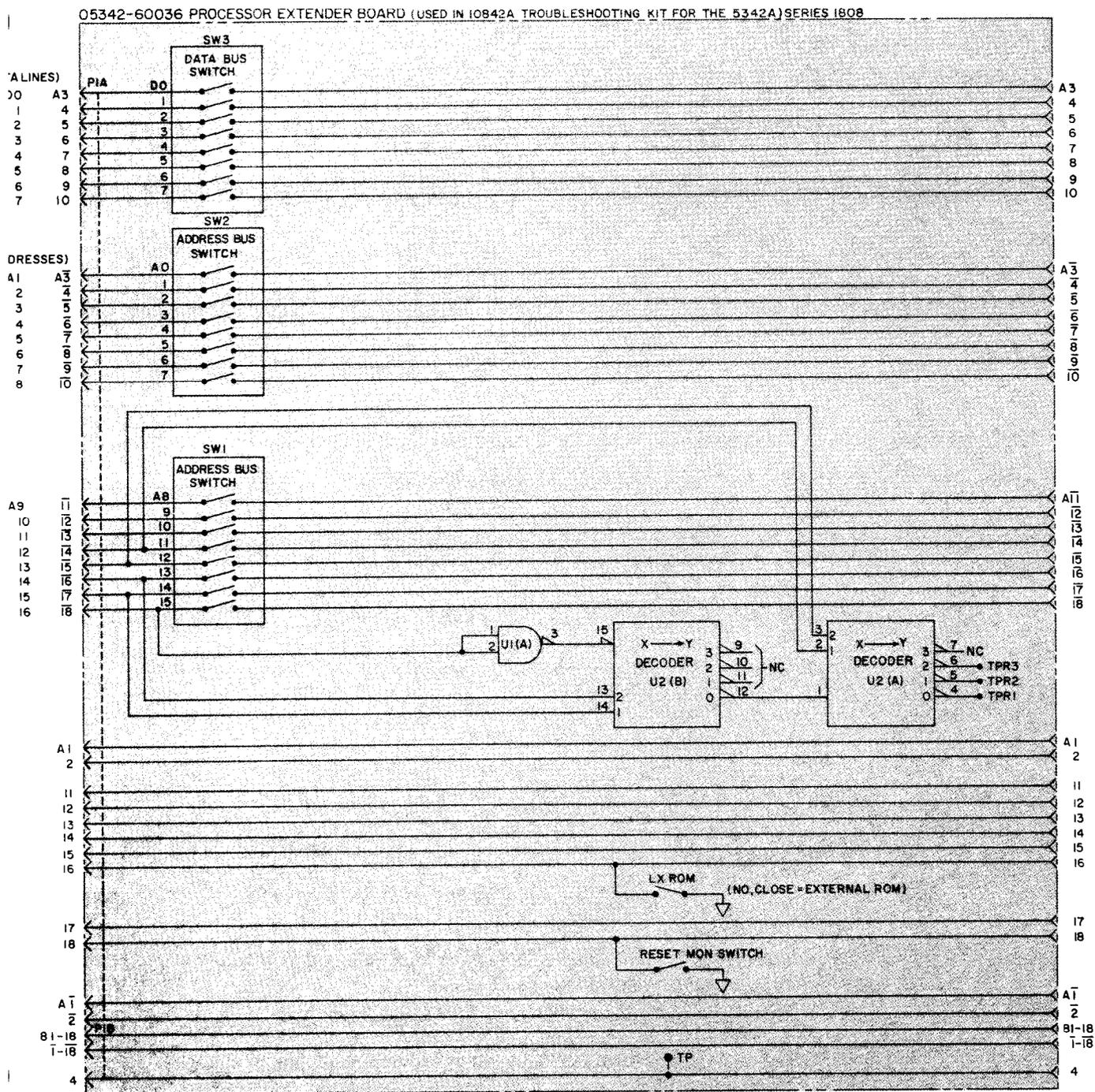
Figure 8-5. Extender Board (05342-60036) Schematic Diagram
