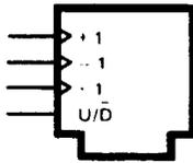
Counter control block. The symbol is used with an array of flip-flops or other circuits serving as a binary or decade counter. An active transition at the +1 or -1 input causes the counter to increment one count upward or downward, respectively. An active transition at the  $\pm 1$  input causes the counter to increment one count upward or downward depending on the input at an up/down control.
