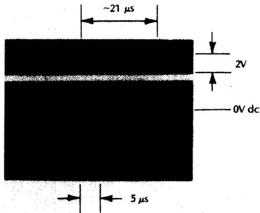
If this doesn't occur, then the divide-by-N circuitry on A10 is faulty.
