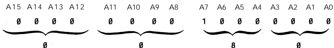
After going through the inverting line drivers U16, U18, and U8, the address lines become:
