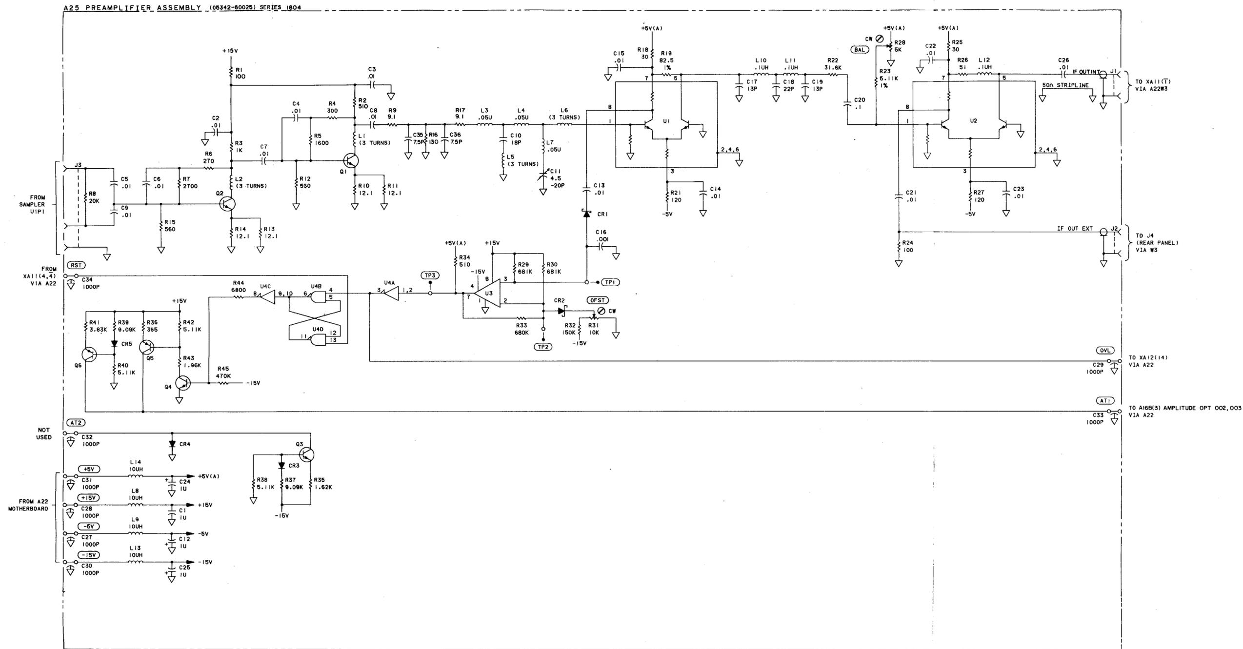
Figure 8-45. A25 Preamplifier Assembly
