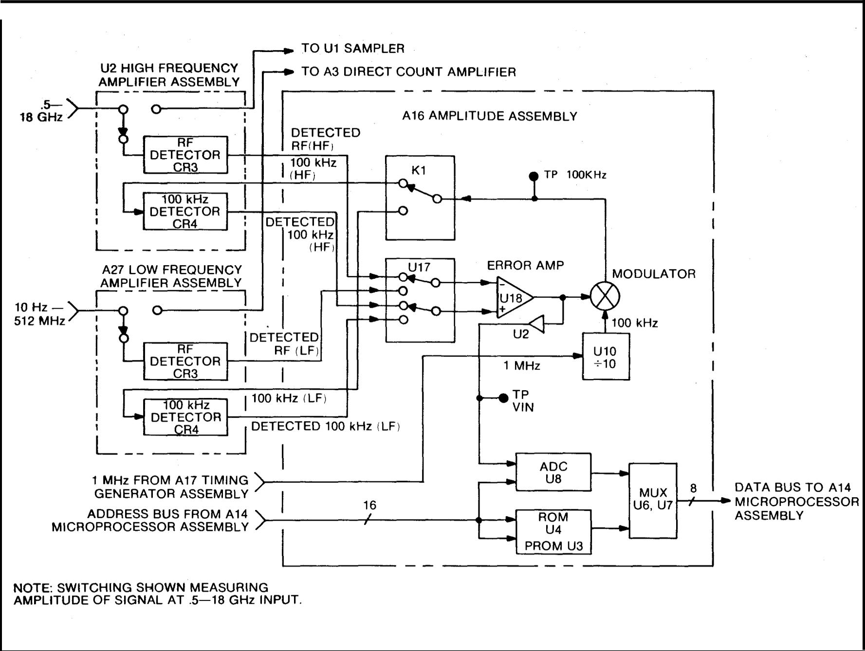
the microwave signal to U212 RF OUT (CR2 is off since the AMPL ON signal is at +0.7 volts). A positive signal at the AMPL ON input (approximately +2.5 volts) turns on CR2 and routes the signal to detector CR3. CR1 is off in this model. The detected microwave signal, DETECTED RF (HF), exists through feedthrough capacitor C10. This dc level can vary from -500  $\mu$ V (for inputs around -30 dBm) up to -2 volts (for +20 dBm inputs).
