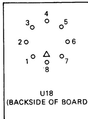
This voltage should be approximately -0.04 Volts. Increase the input level +10 dBm and measure A16U18(2). This voltage should be approximately -0.70 Volts. If not, check U17(15) for these voltages. If still not present, suspect bad cable or failed A27 Low Frequency Amplitude module.
