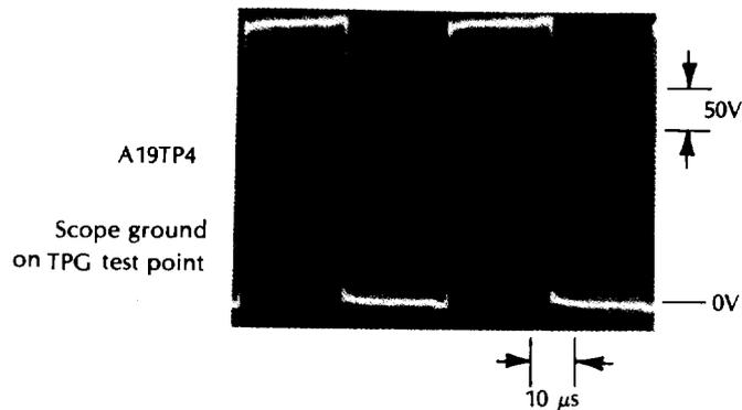
If the above waveform is not present, check the collector of A19Q1 for 300V (with respect to the test point TPG). If 300V dc is not present, suspect input rectifier A19CR1 and associated circuitry. If 300V dc is present, suspect open transistors Q1 and Q2.
