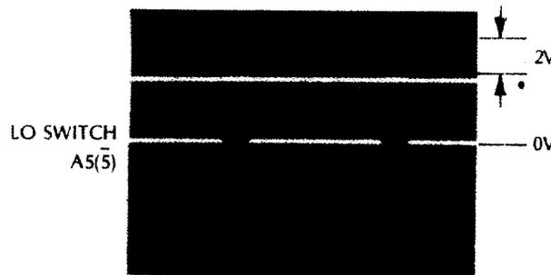
The time during which the signal switches between high and low levels in a pseudorandom fashion should be 360 ms. The time where the signal is high and not switching is controlled by the front panel sample rate control and resolution of counter. If the rear panel switch is placed in the FM position, then the time during which the signal is switching should extend to 2.1 seconds (actually 2.096).
