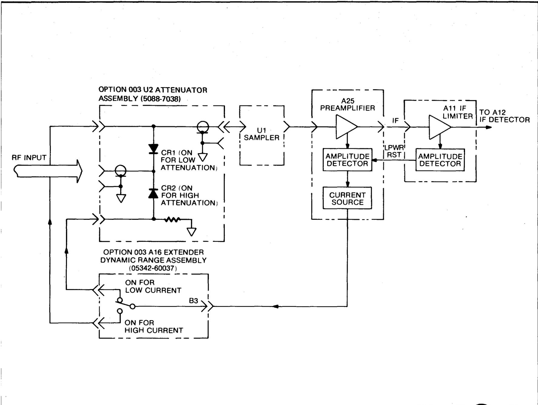
Figure 8-18. Option 003 Extended Dynamic Range Block Diagram
