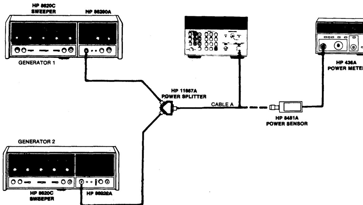
Set generator 1 to 18 GHz and at a level to deliver -5 dBm to the 5342A. To set this level, disconnect generator 2 from the 11667A and terminate that input port of the 11667A with a 909A (Option 012) 50Ω termination. Connect the 8481A to the 5342A end of cable A and adjust the 86290A output for a -5 dBm reading.
