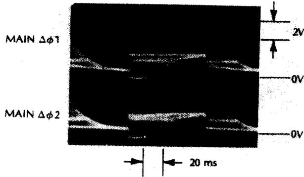
If these signals are not present, then either the divide-by-N or the phase detector on A10 is faulty. If this signal is present but there is no MAIN CNTRL sweep signal at XA8(T) as in step 1, then A9 is faulty.
