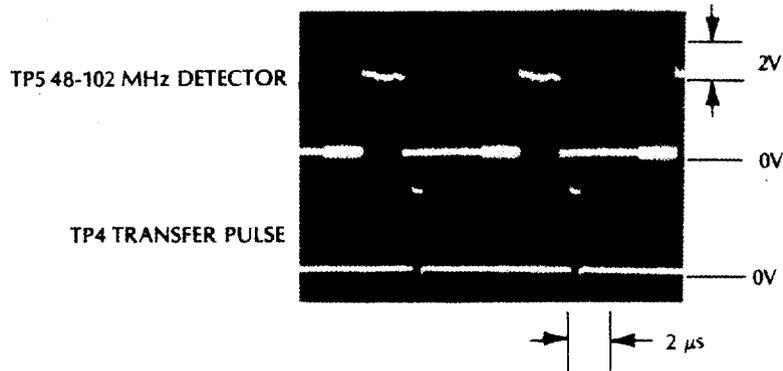
Transfer pulse occurs outside the detector pulse so that a low is transferred into U13.
