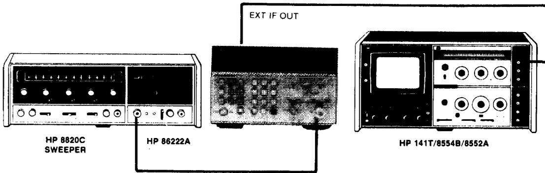
Set the 8620C to 1.2 GHz at approximately -20 dBm. Place the 5342A in AUTO, 500 MHz—18 GHz range, and in diagnostic mode 2 (press SET, SET, 2) so that the counter continuously displays the A counter contents as it remains in the harmonic determination routine. The trace on the spectrum analyzer should show two IF's, indicating that the A5 Multiplexer is switching between the main synthesizer and the offset synthesizer.
