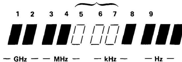
A dc voltage of 0 to 10 volts, corresponding to the selected digits, will be present at the DAC OUT connector on the rear panel. Selected digits 000 produces 0V output, 999 produces 9.99V output.
