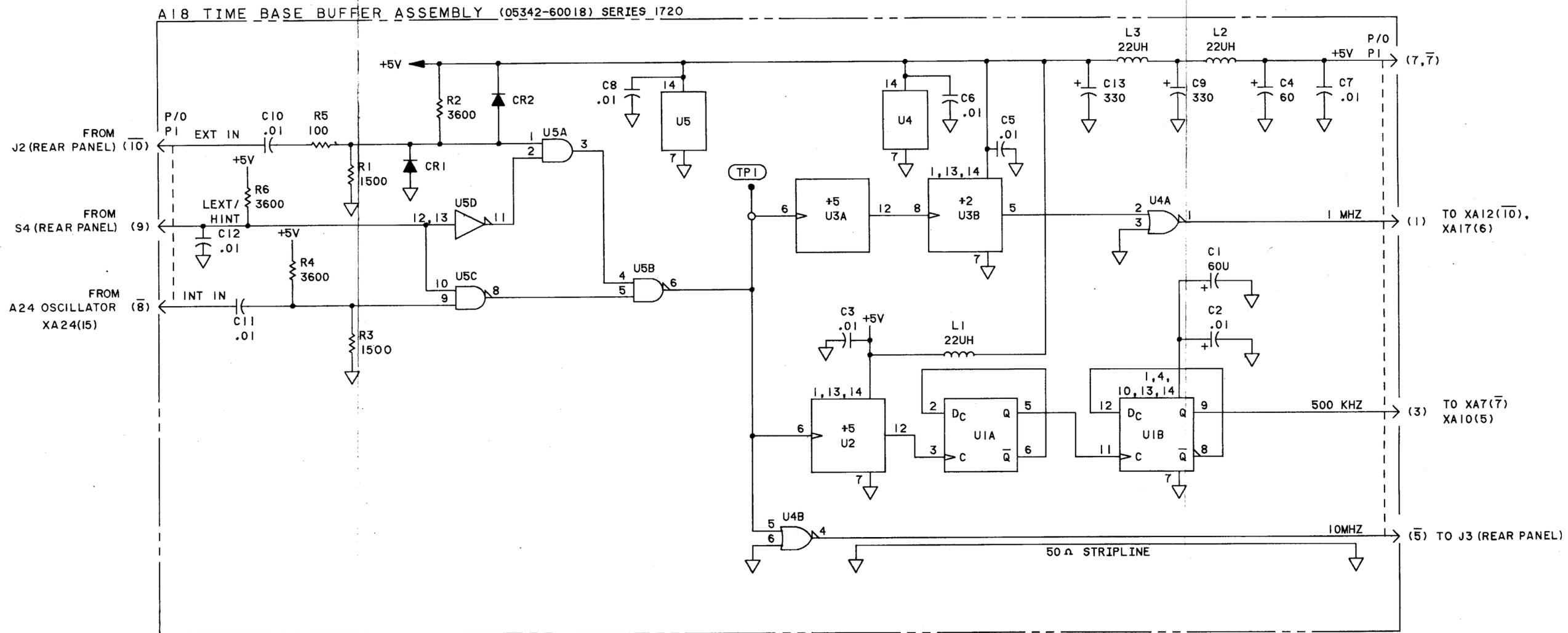
Figure 8-42. A18 Time Base Buffer Assembly
