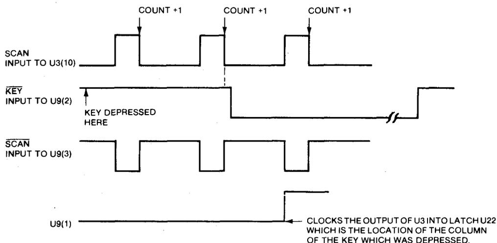
8-140. With KEY low and SCAN low, U9(1) goes high which clocks latch U22 and causes it to store the address (0000 to 1100) of the column of the key which was pushed. Since there are two keys per column, another line is used to indicate top or bottom row. The output of U9(1), which clocks U22, also clocks U19A. U19A(5) will be low if a top row key is pushed and will be high if a bottom row key is pushed. In this manner, the microprocessor determines exactly which key has been depressed.
