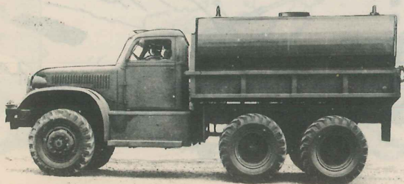
FIGURE 7 - This gravity feed tank is portable.
