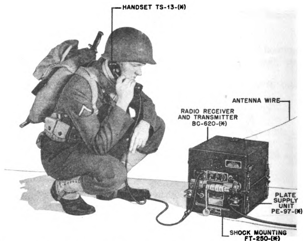
Figure 2. Radio Receiver and Transmitter BC-620-(*), With Plate Supply Unit PE-97-(*), and Shock Mounting FT-250-(*)
