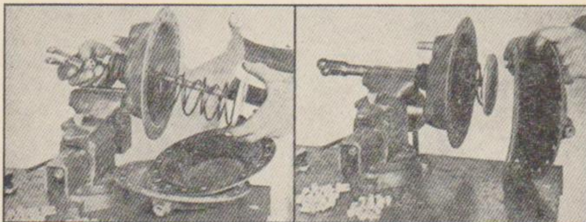
FIGURE B. BRAKE CHAMBER— REPLACING SPRING
