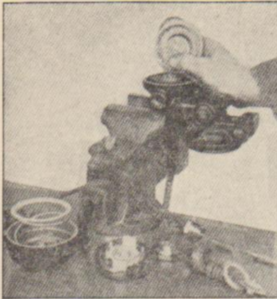
FIGURE H. LIFTING OUT SPRING AND STRAINER
