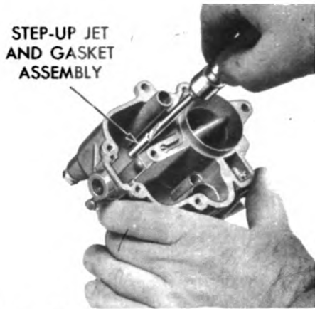
1—REMOVING OR INSTALLING STEP-UP JET
