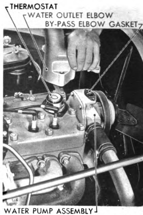
Figure 35—Thermostat Installation
