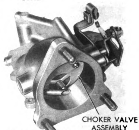
6—CHOKER VALVE INSTALLED
