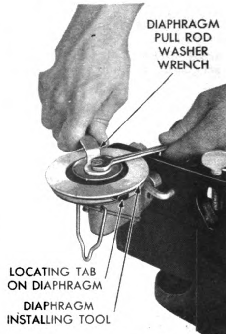
Figure 116—Diaphragm Installation
