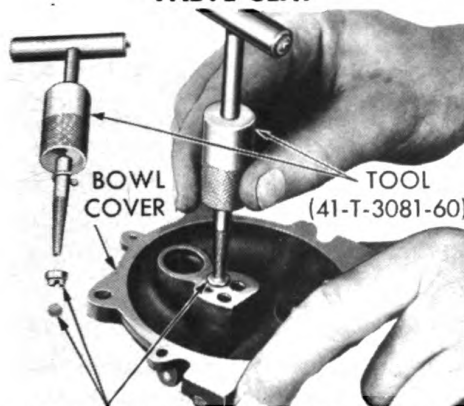
REFILL CHECK VALVE BODY AND DISK 3—REMOVING ACCELERATING PUMP REFILL CHECK VALVE
