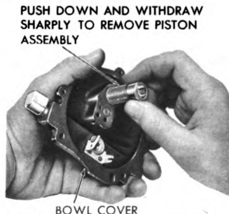
2—REMOVING VACUUM ACCELERATING PUMP PISTON ASSEMBLY
