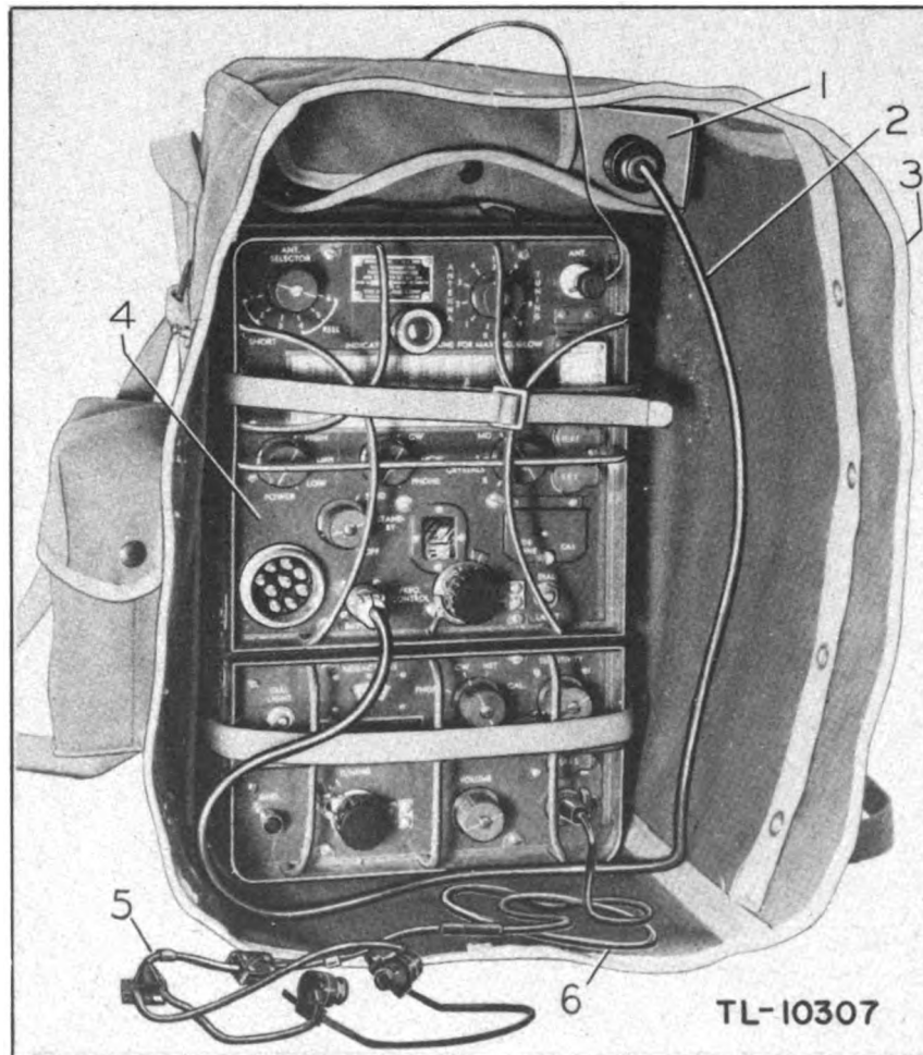
Figure 16—Receiver of Radio Set BC-1306 Operating from Battery BA-48
