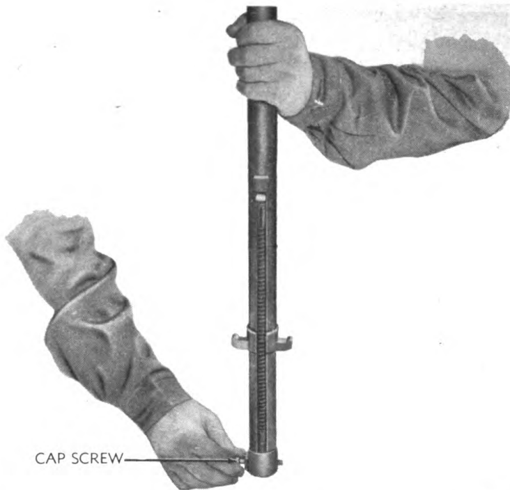
Figure 190. Disassembly of 20-mm hydraulic charger M5.
