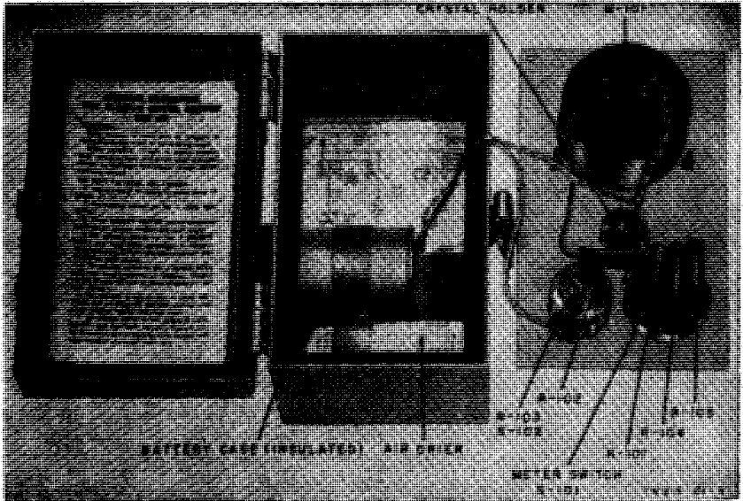
Figure 12. Crystal Rectifier Test Set TS-268C/U, under panel view.
