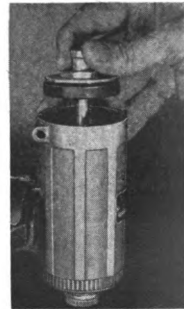
Figure 225 Removing Air Motor Piston
