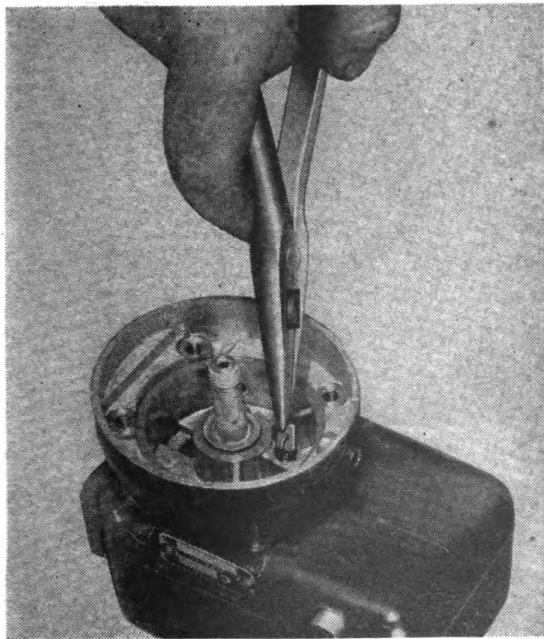
Figure 121 Inserting Oil Scraper
