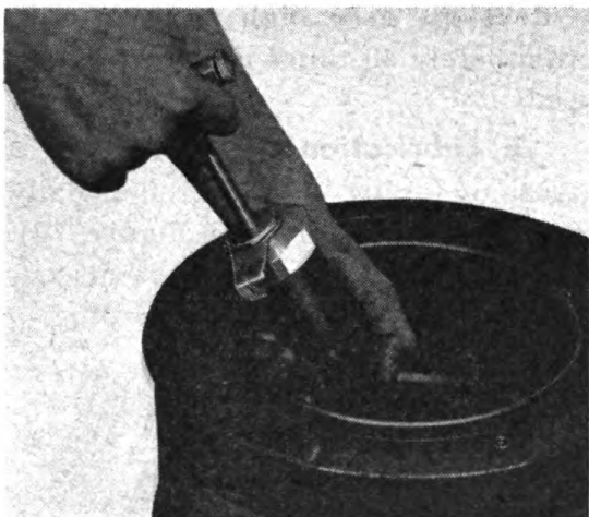
Figure 72 Filling Cylinder with Lubricant
