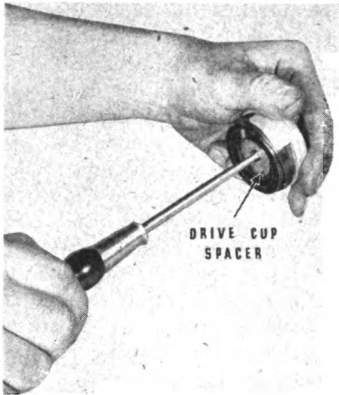
Figure 116 Winding the Spring before Sliding into Cup
