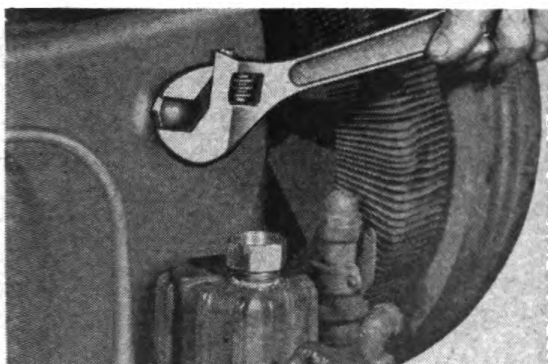
Figure 153 Removing Oil Circulating Ring Retainer
