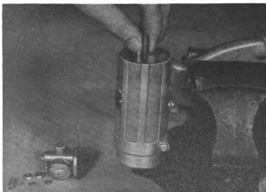
Figure 220 Removing Bottom Air Valve Spring
