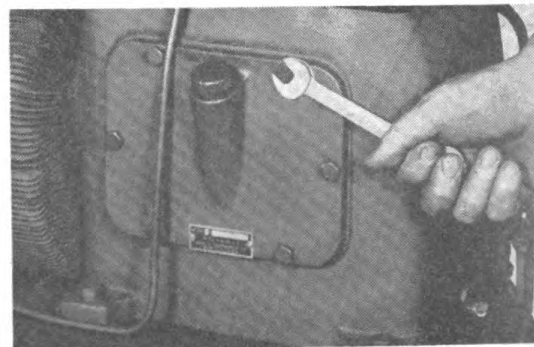
Figure 150 Removing Inspection Plate Screw
