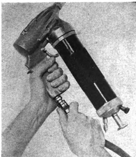
Figure 69 Attaching Air Hose to Gun *
