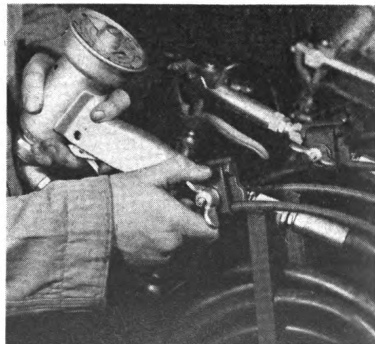
Figure 16 Releasing Hose Clamp from Rim of Reel
