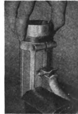
Figure 224 Removing Locking Sleeve
