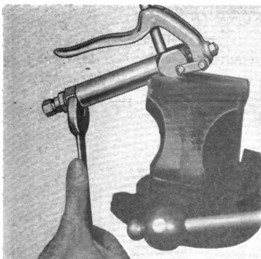
Figure 187 Removing Retaining Bushing
