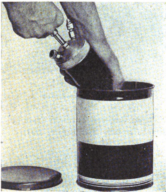
Figure 67 Filling Cylinder with Lubricant
