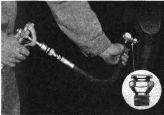
Figure 23 Lubricating Bearing equipped with Giant Button Head Fitting
