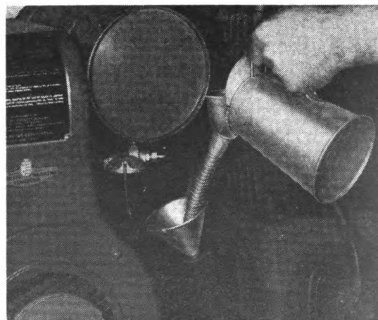
Figure 35 Filling Compressor Crankcase with Oil
