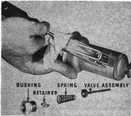
Figure 192 Cleaning Valve Seat
