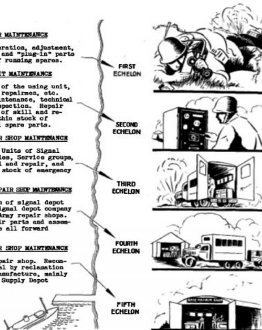
FIGURE 1301. Echelons of Signal Repair Theater of Operations
