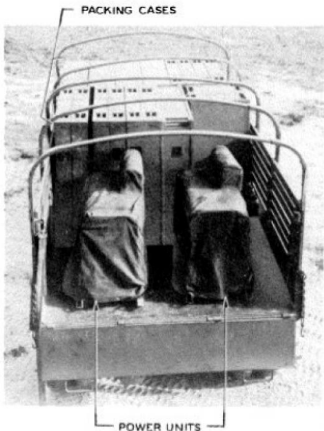
FIGURE 504. Operations Center AN/TTQ-1 Equipment Packed in Truck
