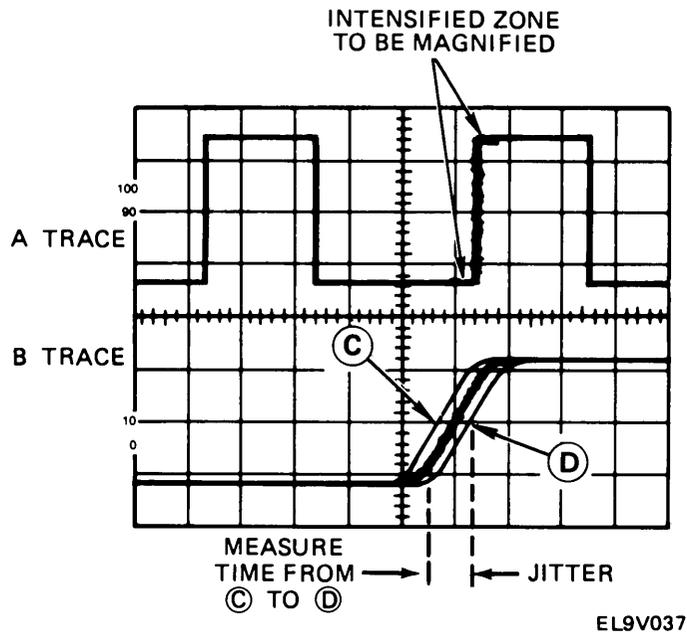
p. Triggered Magnified Sweep Measurement.
