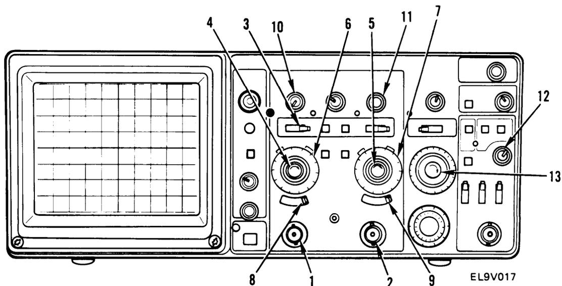
3. Set CH 1 or CH 2 VOLTS/DIV variable control (4 or 5) to CAL detent position, and set appropriate VOLTS/DIV switch (6 or 7) for desired deflection.
