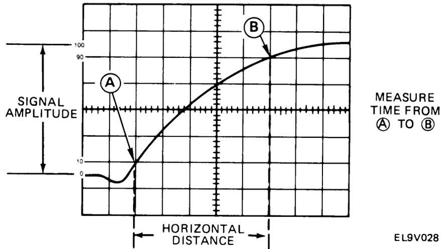
8. Determine horizontal distance between 10% and 90% points (points A and B) and calculate time duration using formula:
