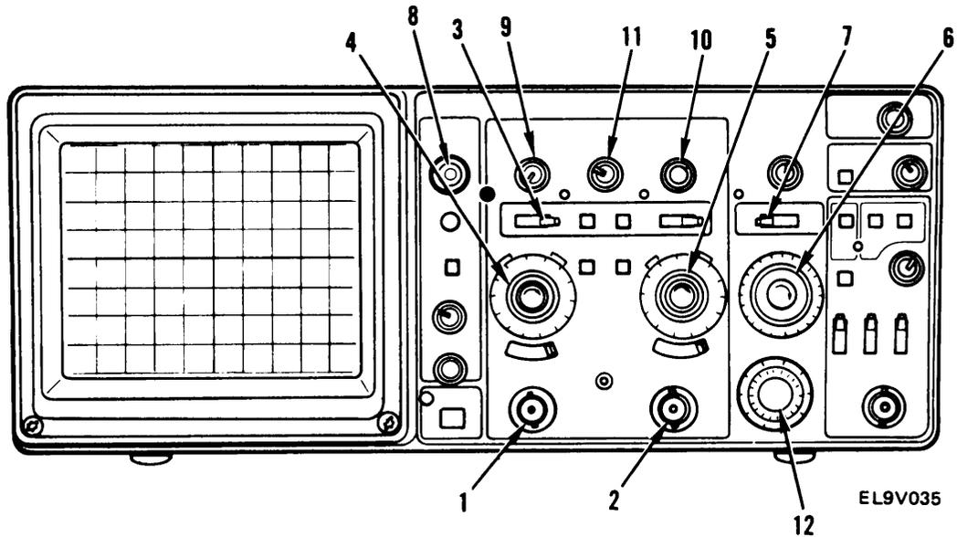
4. Set appropriate CH 1 or CH 2 VOLTS/DIV switch (4 or 5) to provide display amplitude of two or three divisions.
