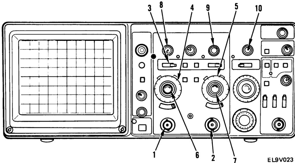
4. Adjust CH 1 or CH 2 VOLTS/DIV switch (4 or 5) and appropriate VOLTS/DIV variable control (6 or 7) for display amplitude of five vertical divisions.
