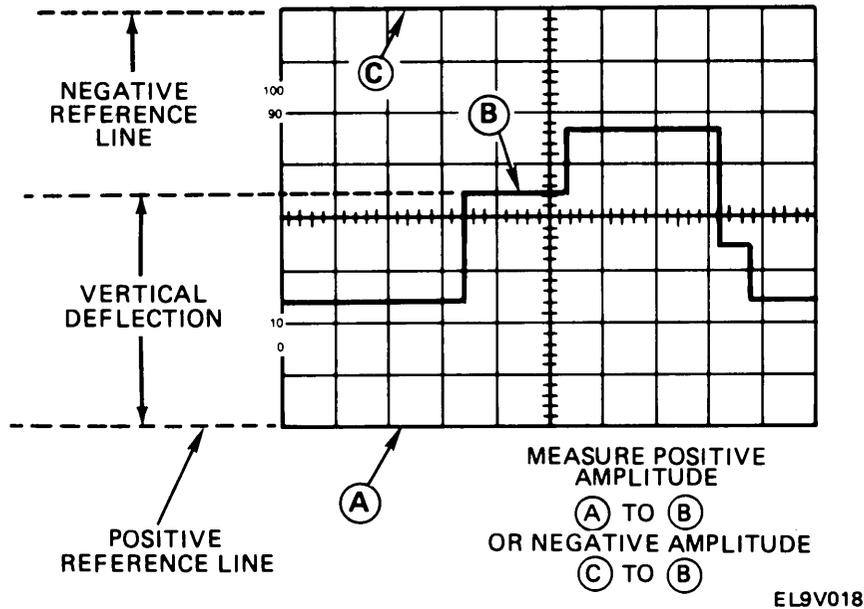
11. Count number of divisions of vertical deflection between ground reference line and point on waveform at which voltage level is to be determined.
