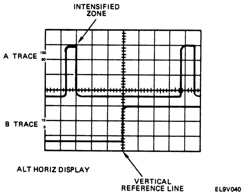
5. Ensure that SEC/DIV variable control (6) is in CAL detent position and set A SEC/DIV Switch (7) to sweep speed setting that displays measurement points on waveform.
