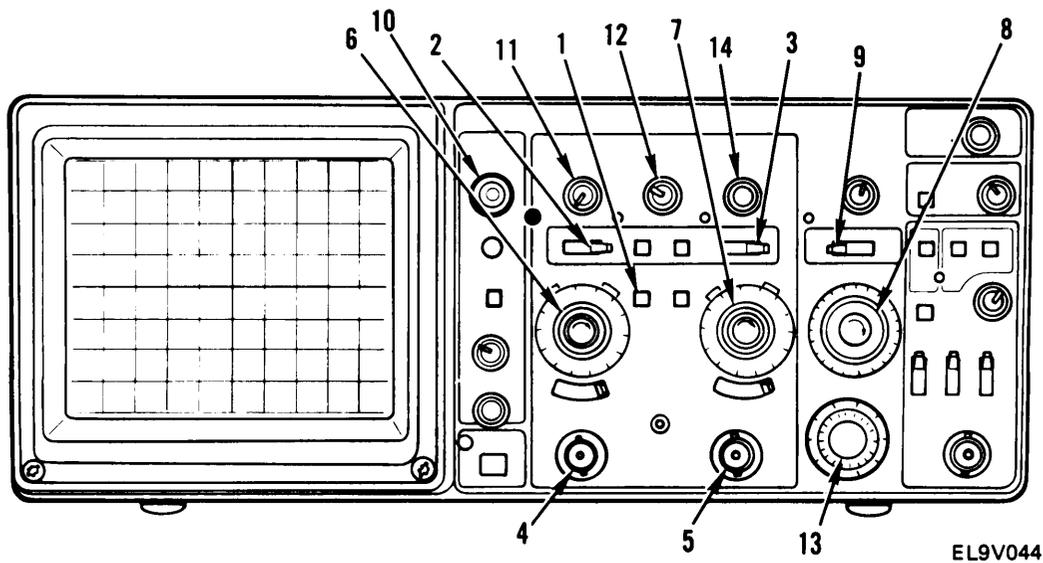
5. Using either probes or cables with equal time delays, connect known reference signal to CH 1 OR X connector (4) and comparison signal to CH 2 OR Y connector (5).
