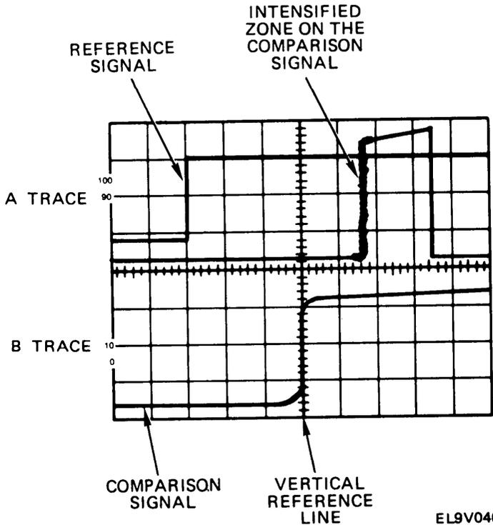
16. Calculate time difference between reference signal and comparison signal using formula:
