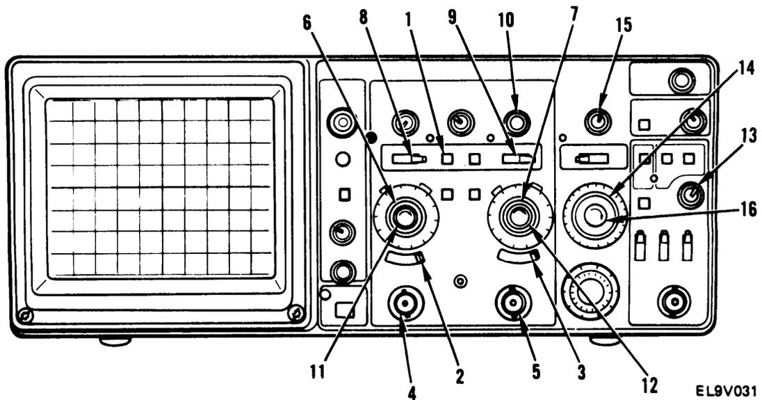
9. Adjust both CH 1 and CH 2 VOLTS/DIV variable controls (1 1 and 12) until two displays are equal in amplitude.
