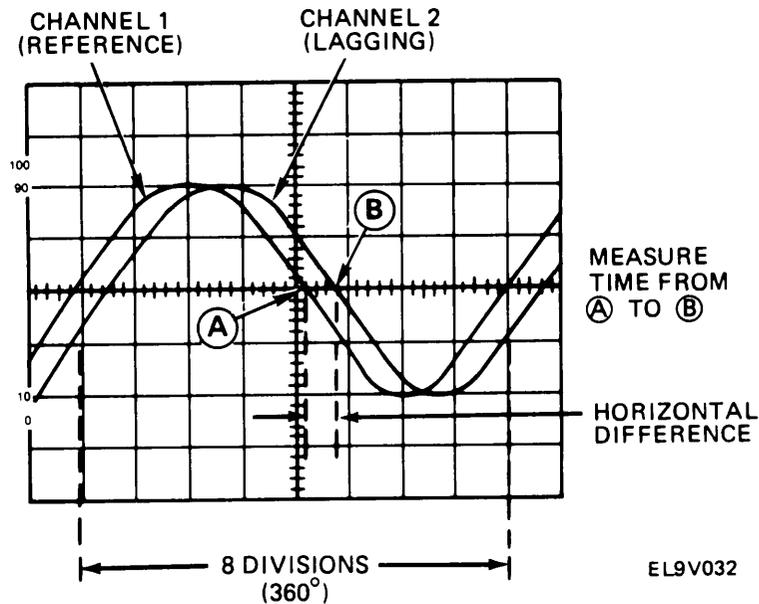
14. Determine horizontal difference between corresponding points on waveforms at common horizontal graticule line and calculate phase difference using formula:
