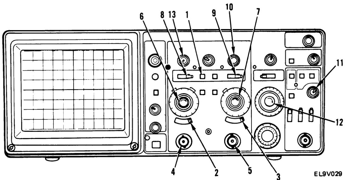
9. Adjust A TRIGGER LEVEL control (11) for stable display.
