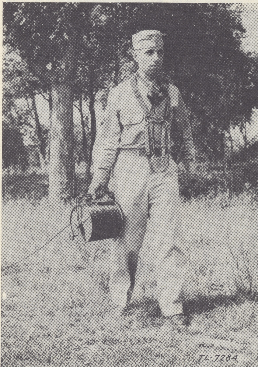
Figure 3. Laying wire with Reel Equipment CE-11.
