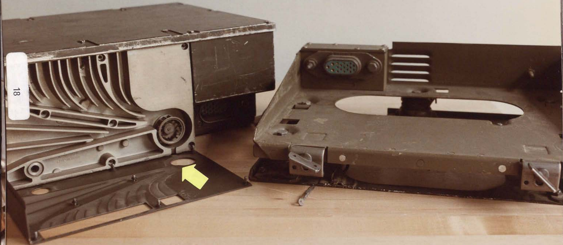
FIGURE 13. RT-524/VRC RADIO WITH MT-1029/VRC MOUNT, REAR PLATE REMOVED, SHOWING FAN LOCATION; ARROW POINTS TO DENT ON PLATE.
