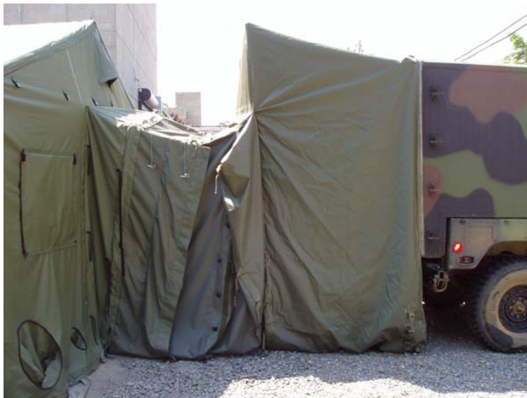
Figure 17. Boot Wall Installed.
