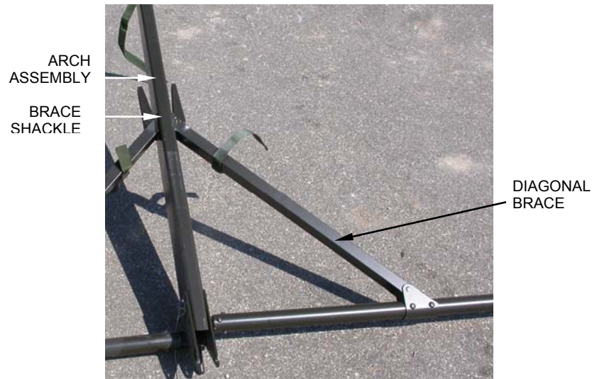
Figure 13. Locking Purlin Diagonal Brace.
