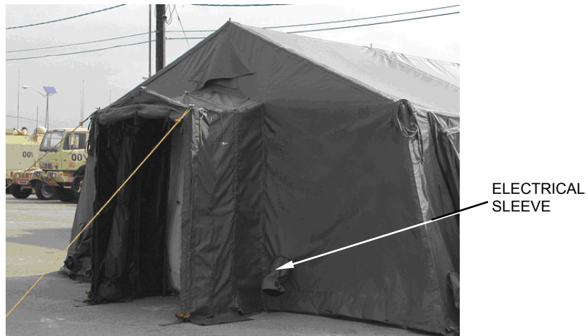
Figure 49. Electrical Sleeve Location.
