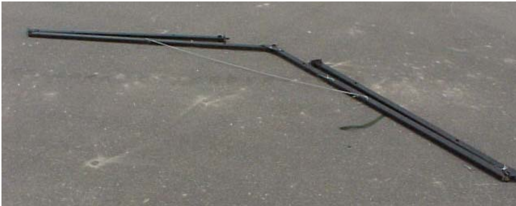
Figure 9. Arch Assemblies, Cable Attached.
