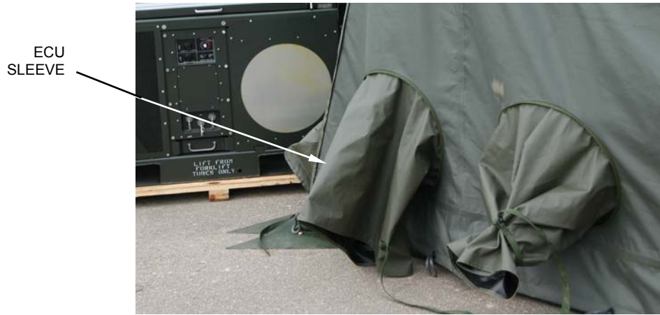
Figure 50. ECU Sleeve Location.
