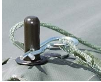
Figure 26. Hitch Clip Pin in Spindle.
