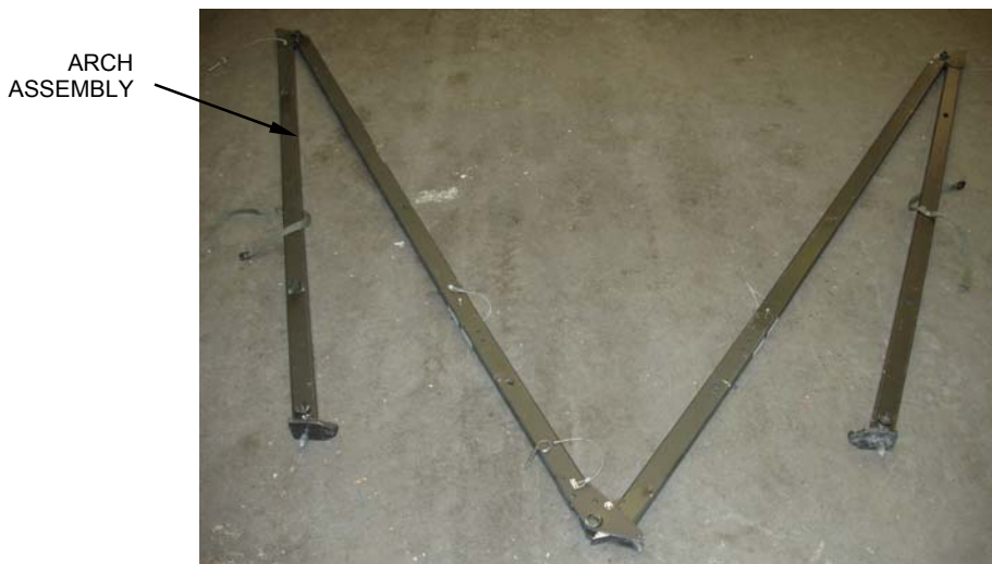
Figure 7. Connected Arch Assemblies, Flat.
