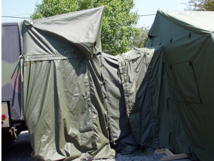
Figure 16. Excess Fabric, Rolled and Buckled.
