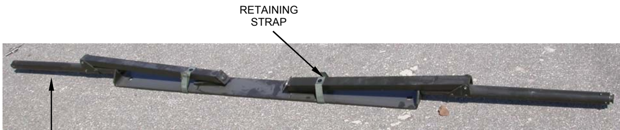
Figure 1. Door Sill Assembly (Folded for Transport).
