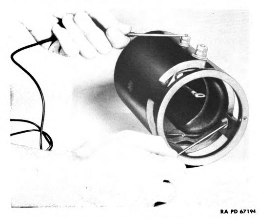
Figure 110—Testing Generator Field Coils for Open Circuit
