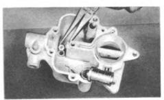
32. MAIN METERING JET AND GASKET INSTALLATION
