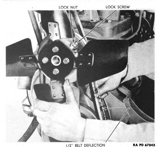
Figure 139—Fan Belt Adjustment
