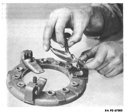
Figure 149—Release Lever and Eyebolt Removal
