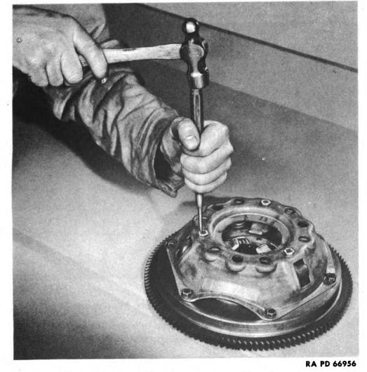
Figure 156—Locking Release Lever Adjusting Nut
