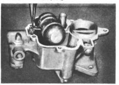
7. FLOAT ASSEMBLY AND PIN REMOVAL
