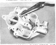
11. DISCHARGE BALL CHECK SPRING AND PLUG REMOVAL
