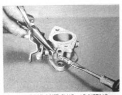
16. IDLE PORT RIVET PLUG. ADJUSTING SCREW, AND SPRING REMOVAL RA PD 66992
