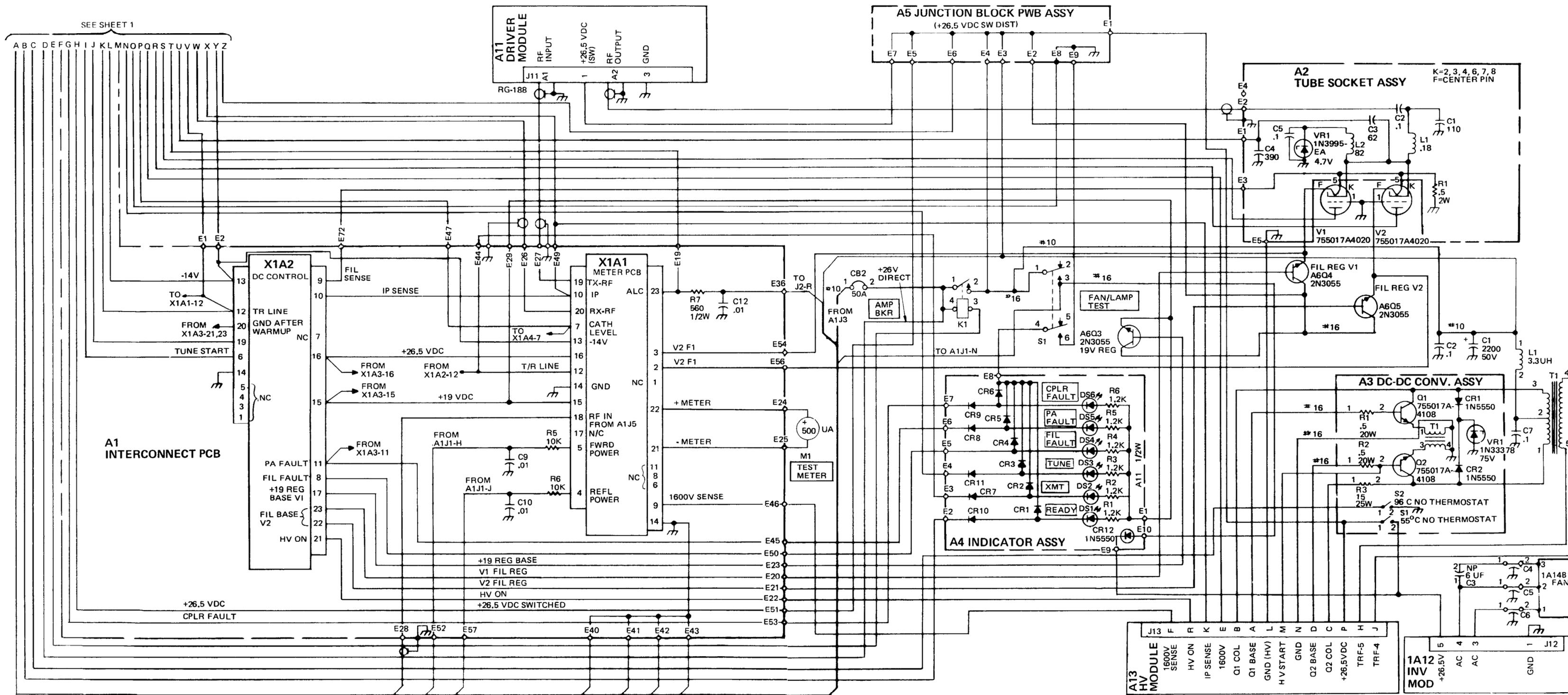
Figure 6. Case Assembly 1A14 Interconnection Diagram (Sheet 2 of 2)
