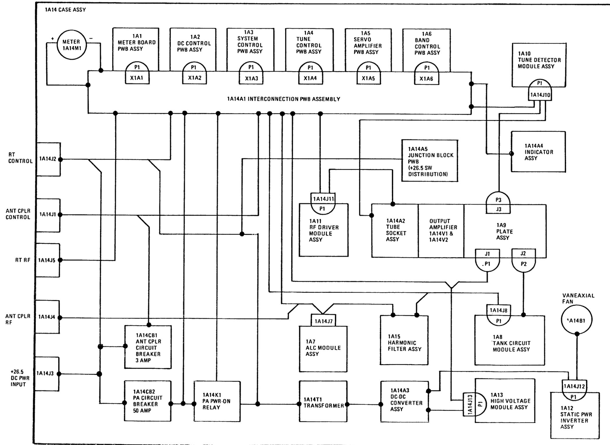
Figure 4. Unit Cabling and Connector Diagram
