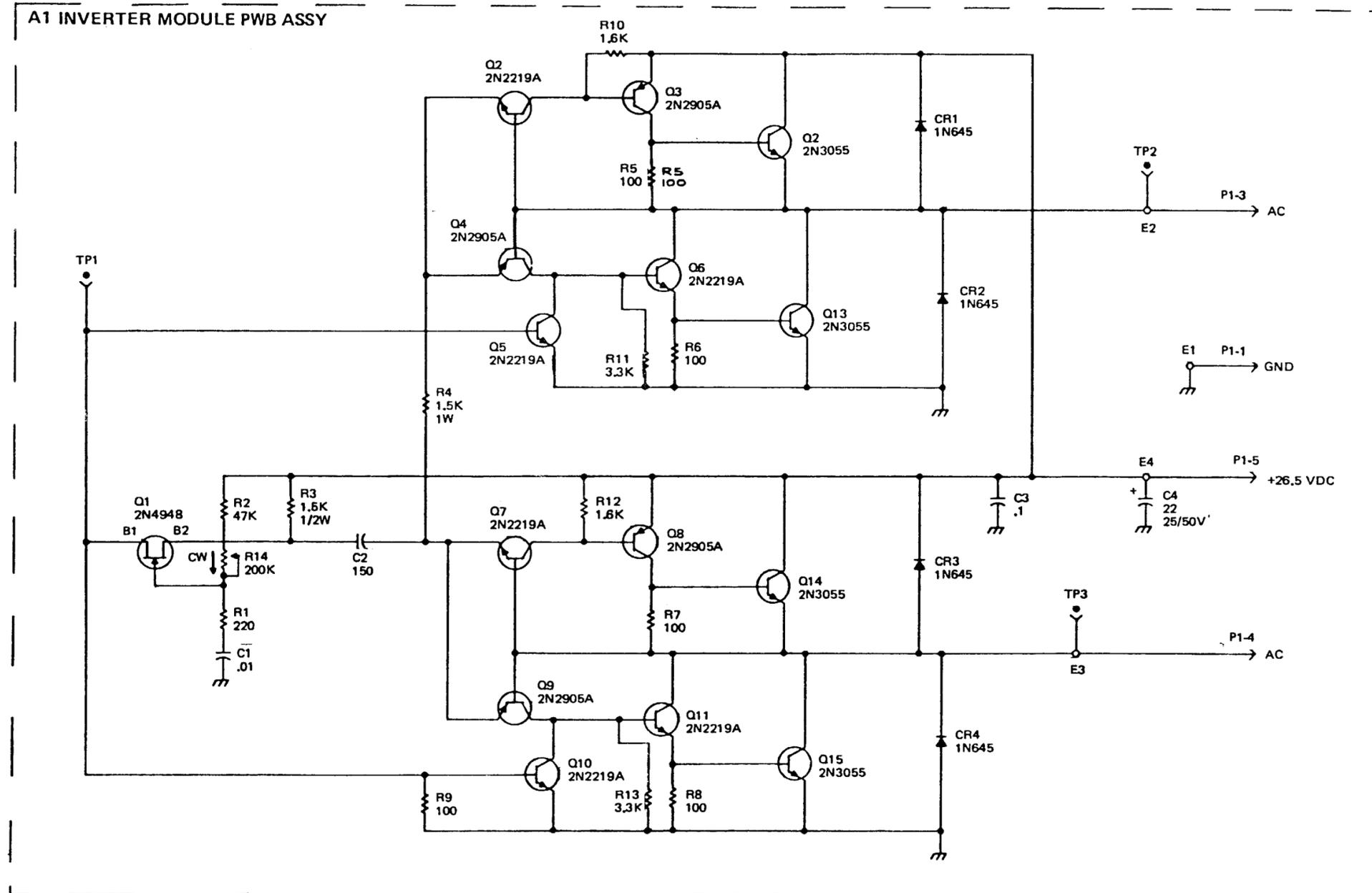
Figure 19. Static Power Inverter Assembly 1A12, PN 755017A4900 (Sheet 1 of 2)
