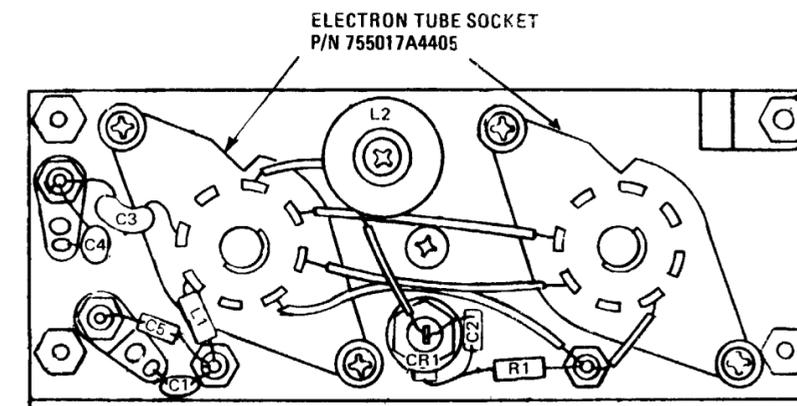
Figure 23. Tube Socket Assembly 1A14A2, PN 755017A4400
