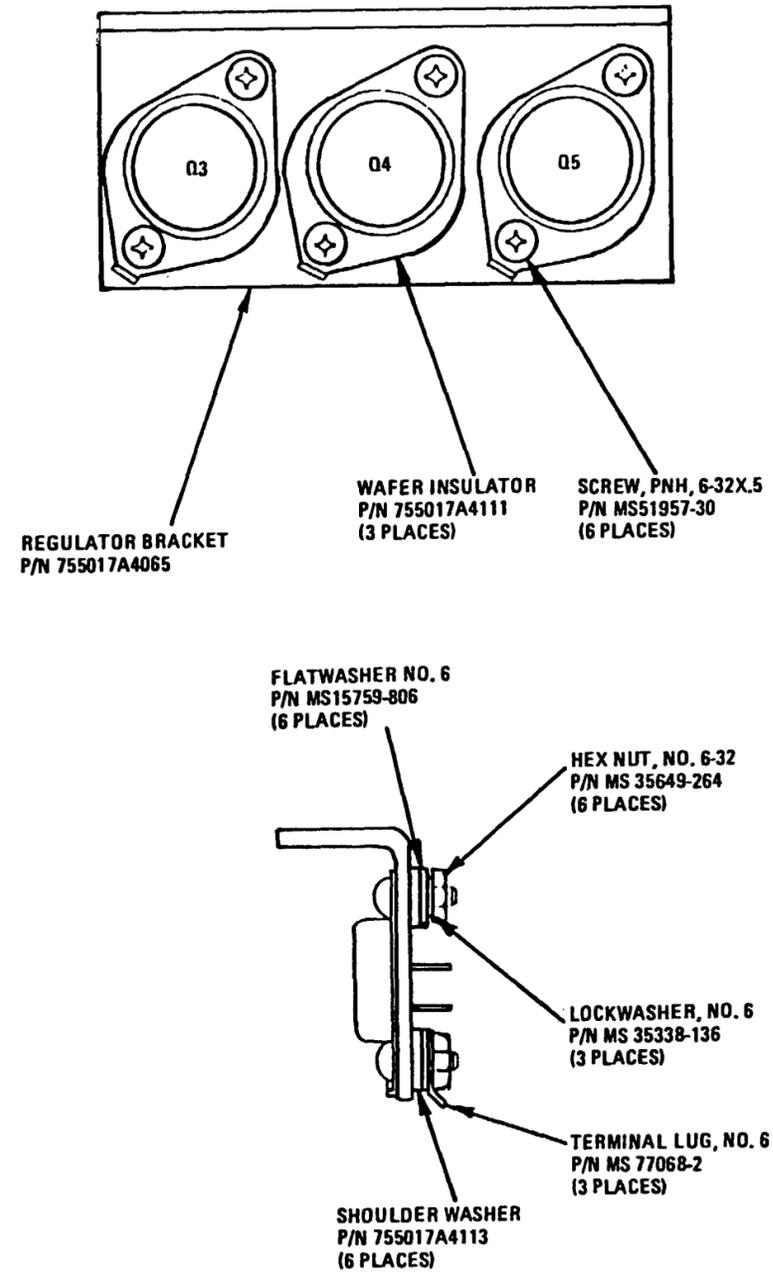
Figure 26. Regulator Assembly 1A14A6, PN 755017A4031
