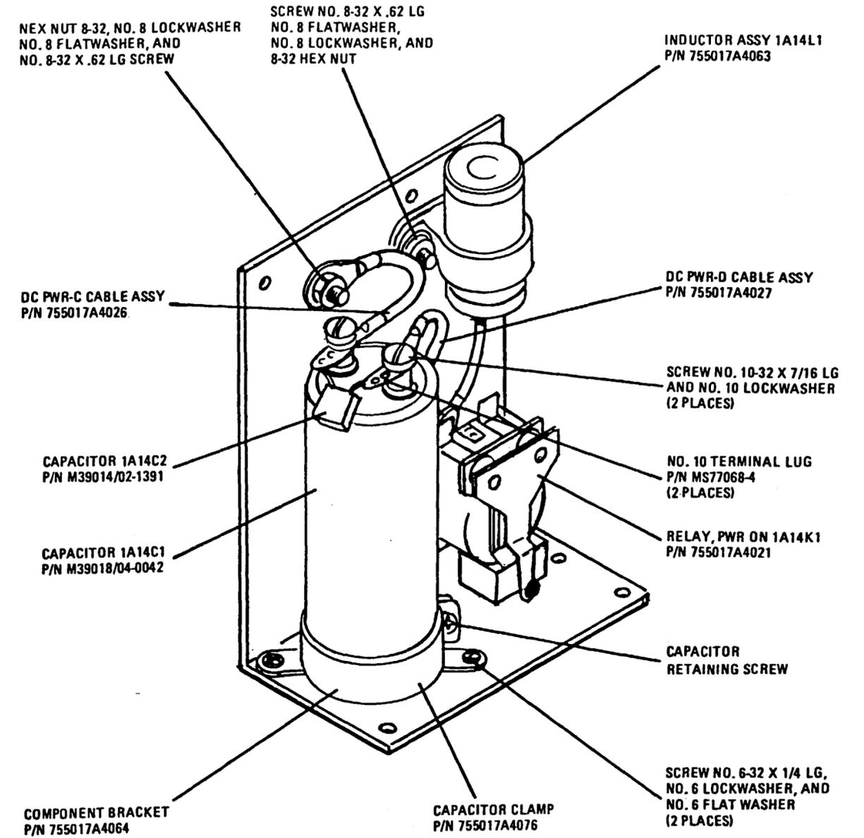
Figure 27. Component Bracket Assembly, PN 755017A4064
