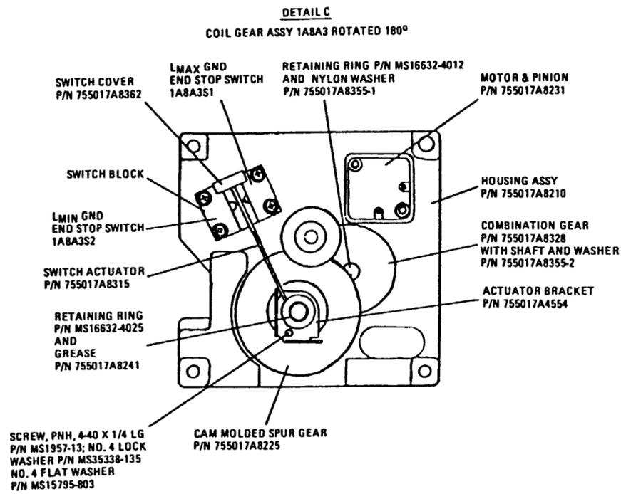
COIL GEAR ASSEMBLY 1A8A3, PN 755017A4550
