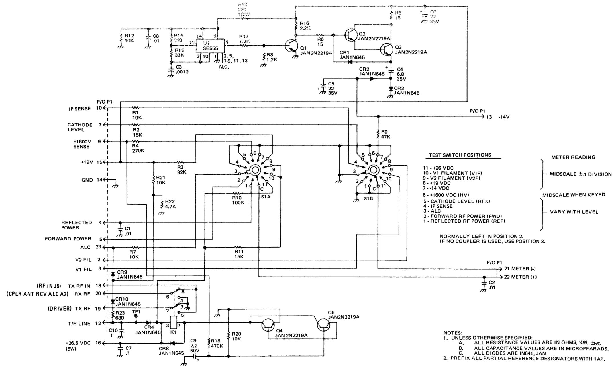
Figure 8. Meter Board PWB Assembly 1A1, PN 755017A4210 (Sheet 1 of 2)
