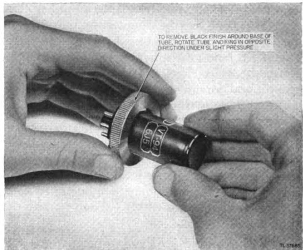
Figure 8. Removing black finish to insure grounding.
