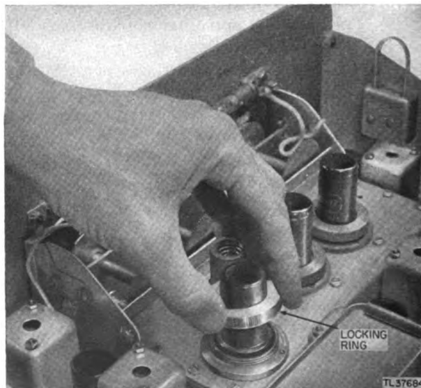
Figure 7. Receiver—top view showing tube locking rings.
