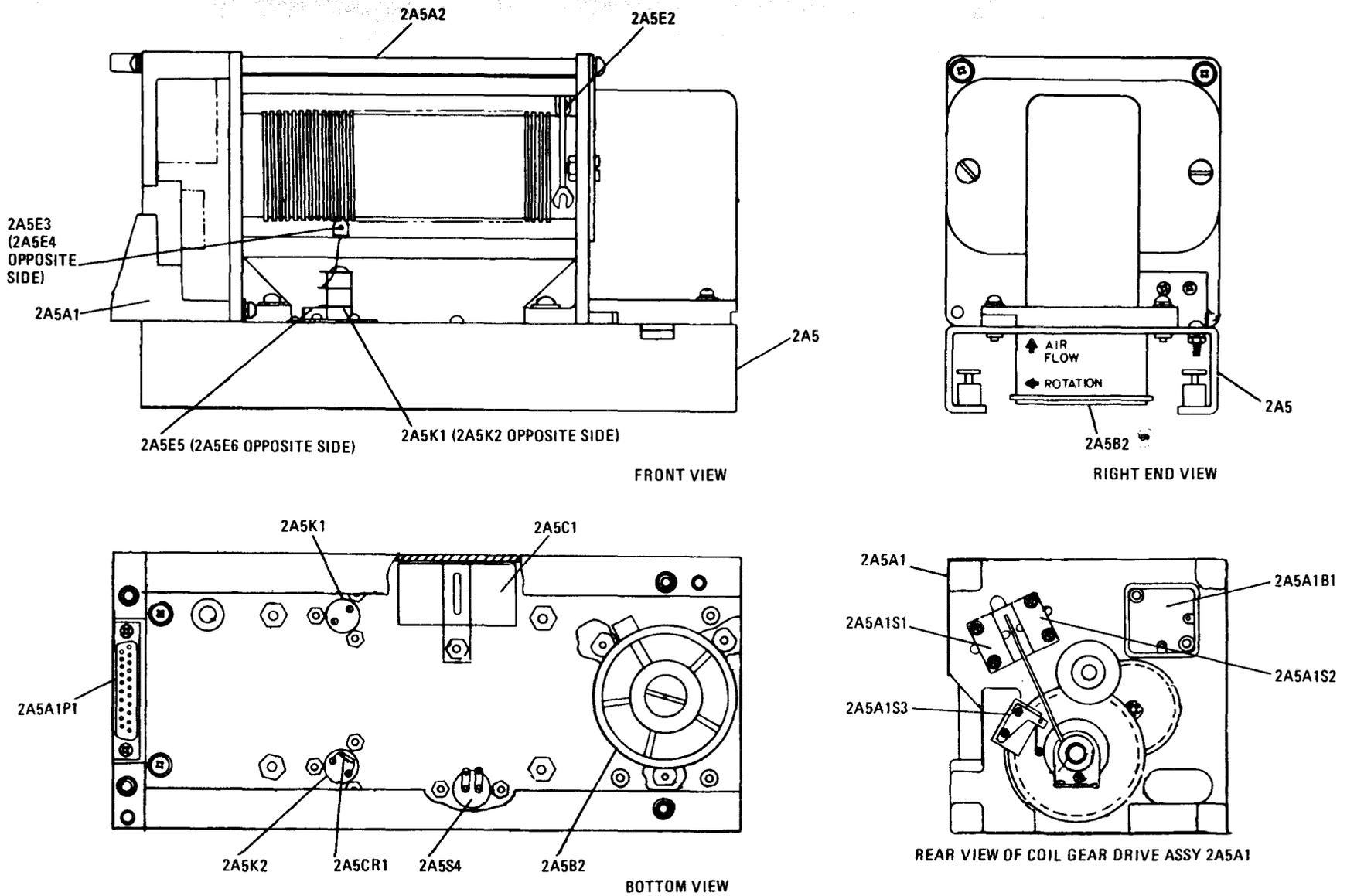
Figure 3-31. Inductive RF Tuner Assembly 2A5 Component Locations
