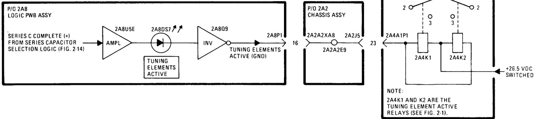
Figure 2-15. Simplified Tuning Elements Active Logic Diagram
