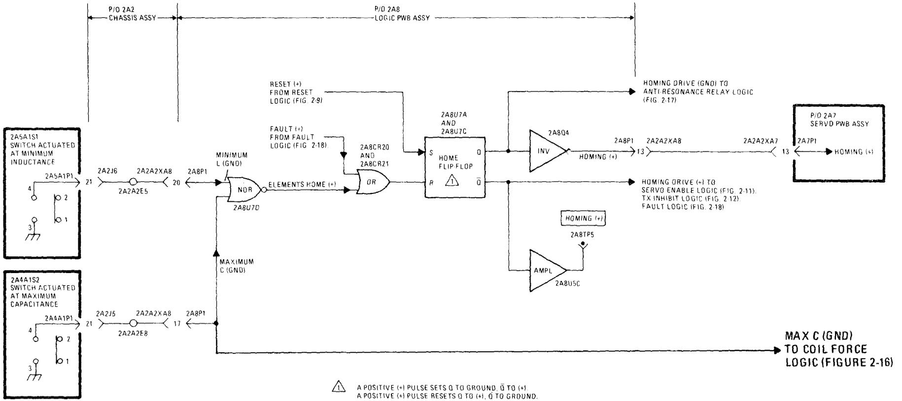
Figure 2-10. Simplified Homing Logic Diagram
