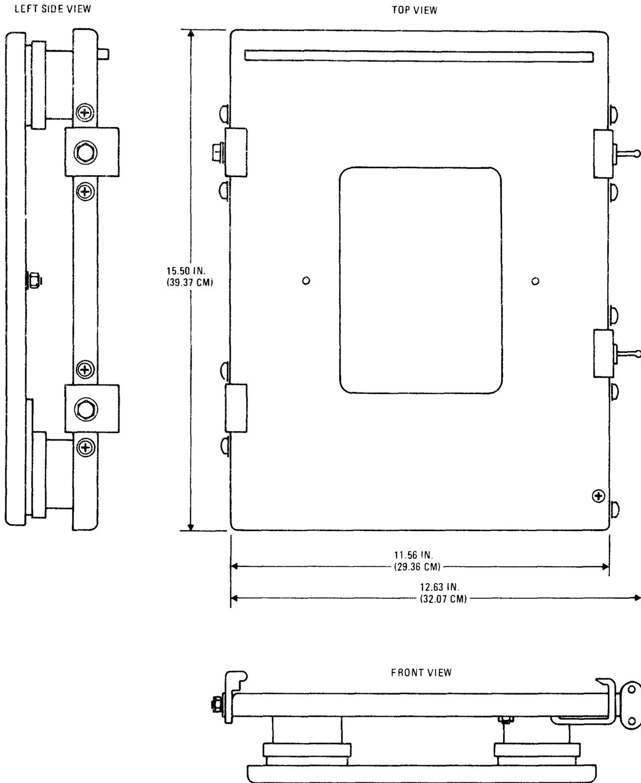
Figure 1-6. Antenna Coupler Mount MT4495/GRC-193 Detail Views
