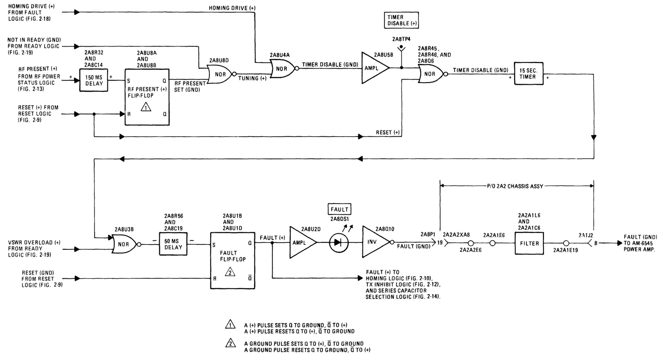
Figure 2-18. Simplified Fault Logic Diagram
