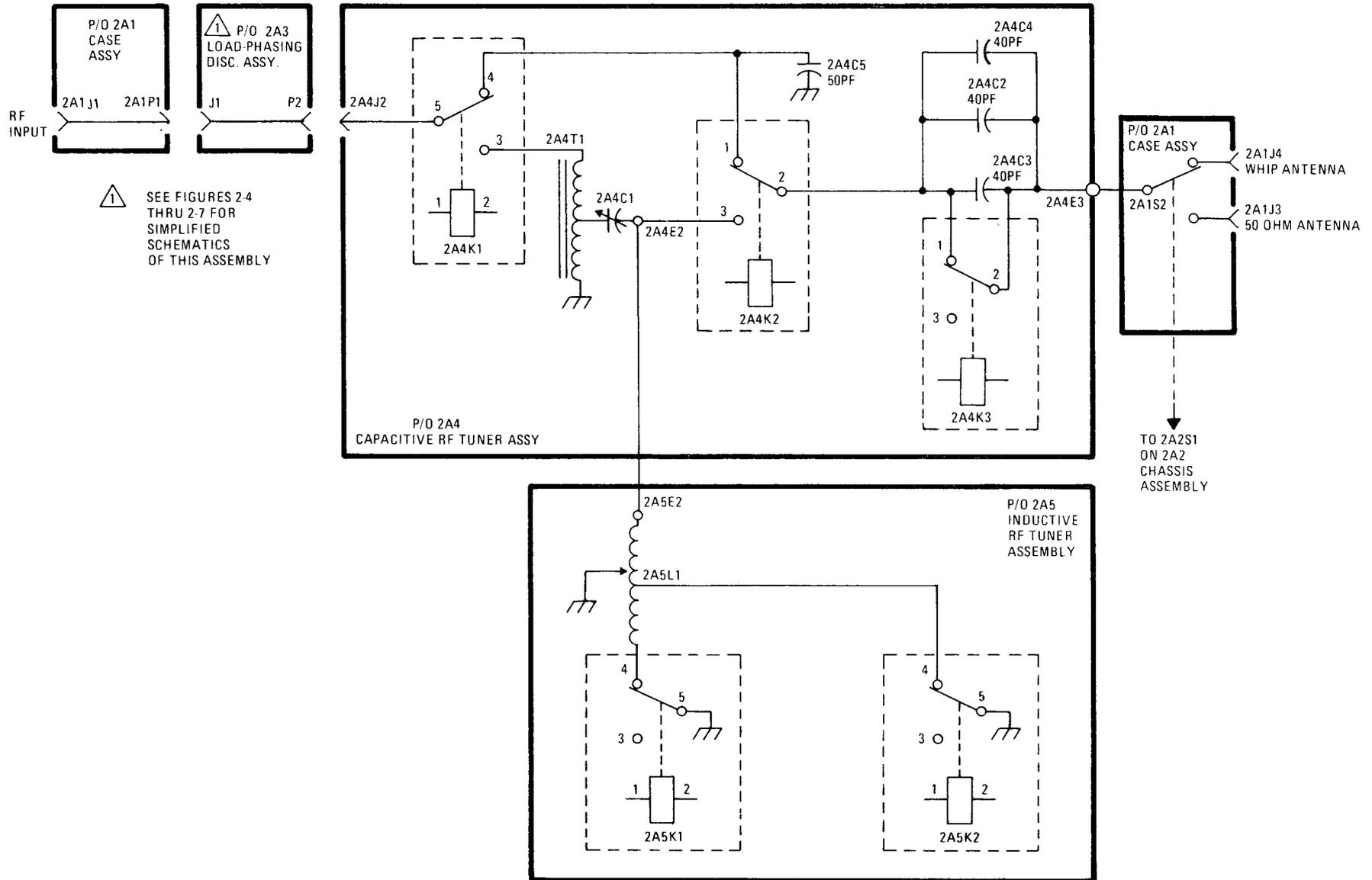
Figure 2-1. RF Flow Diagram
