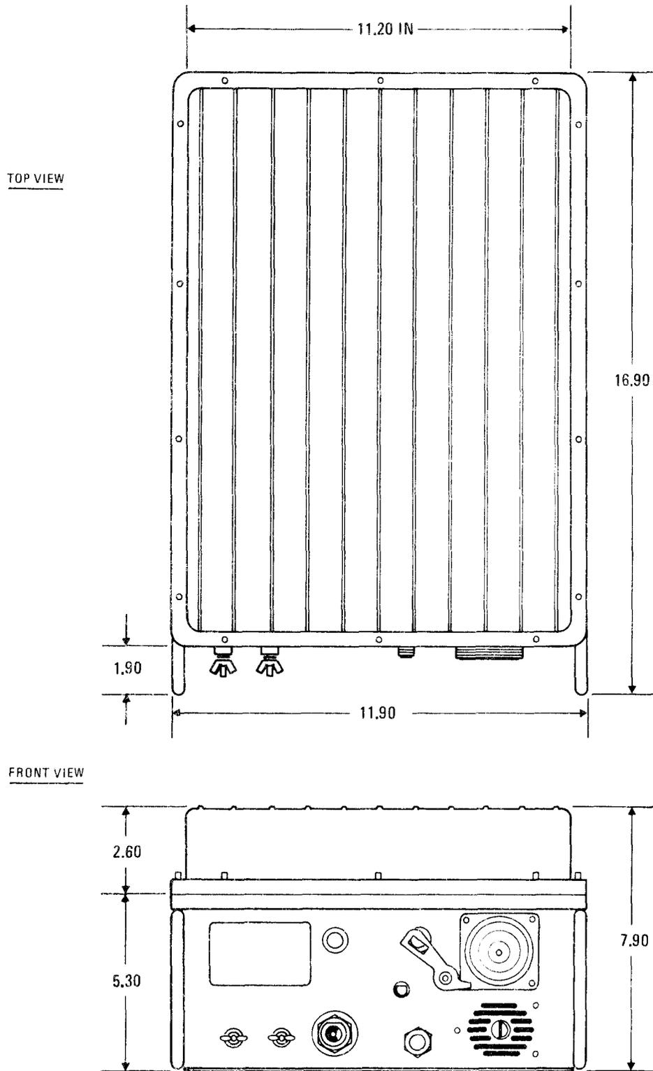
Figure 1-8. Antenna Coupler CU-2064/GRC-193 Dimensioned Views
