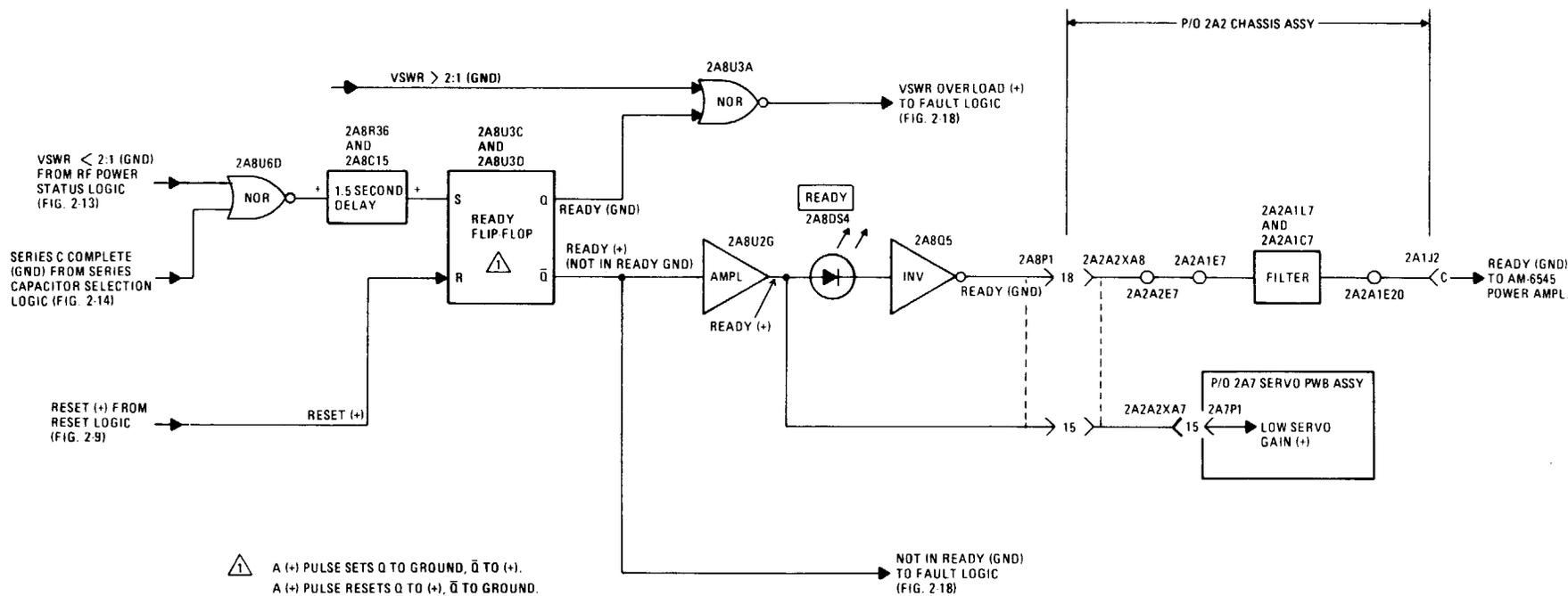
Figure 2-19. Simplified Ready Logic Diagram
