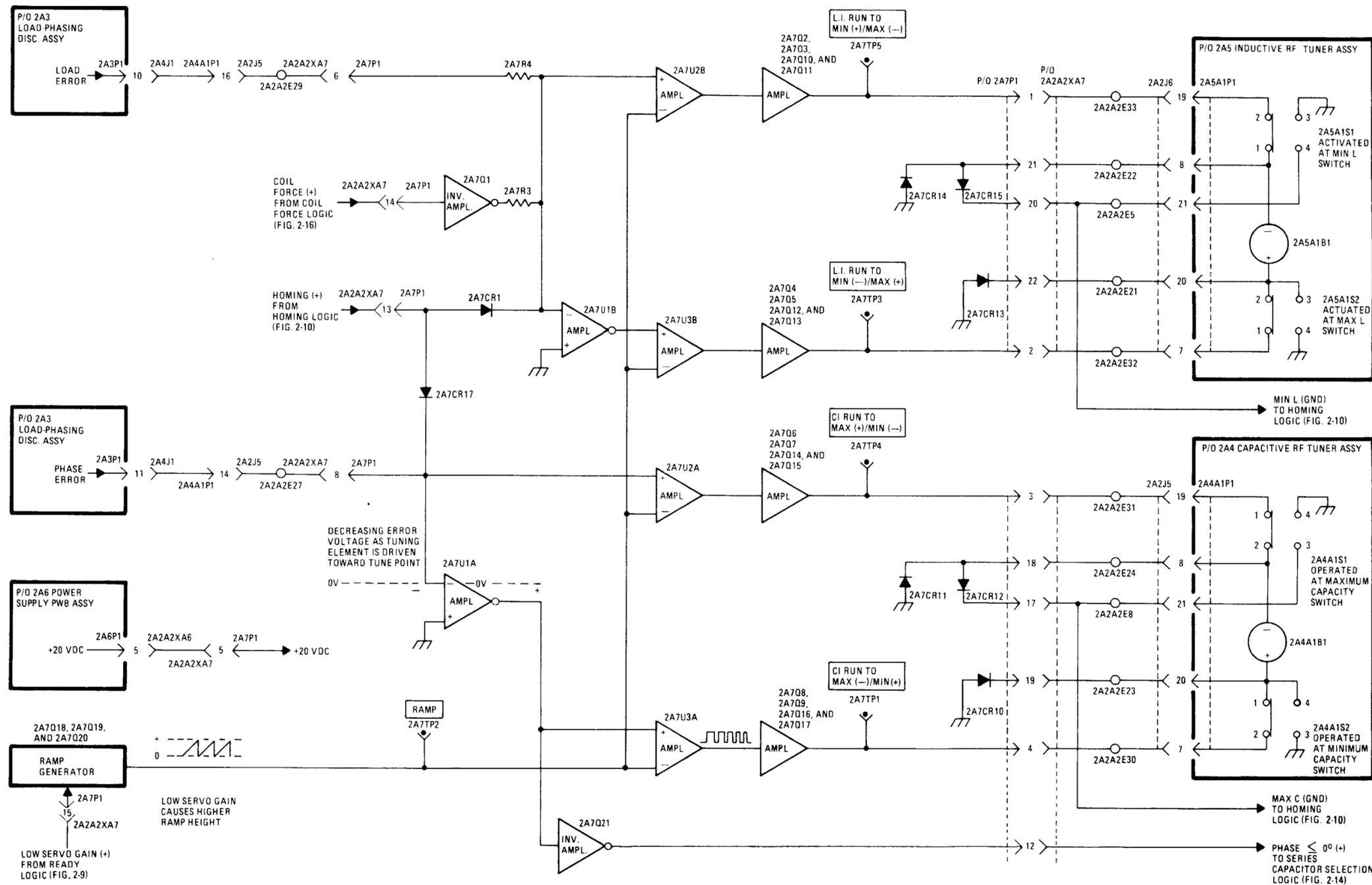
Figure 2-21. Simplified Servo PWB 2A7 Circuit Diagram
