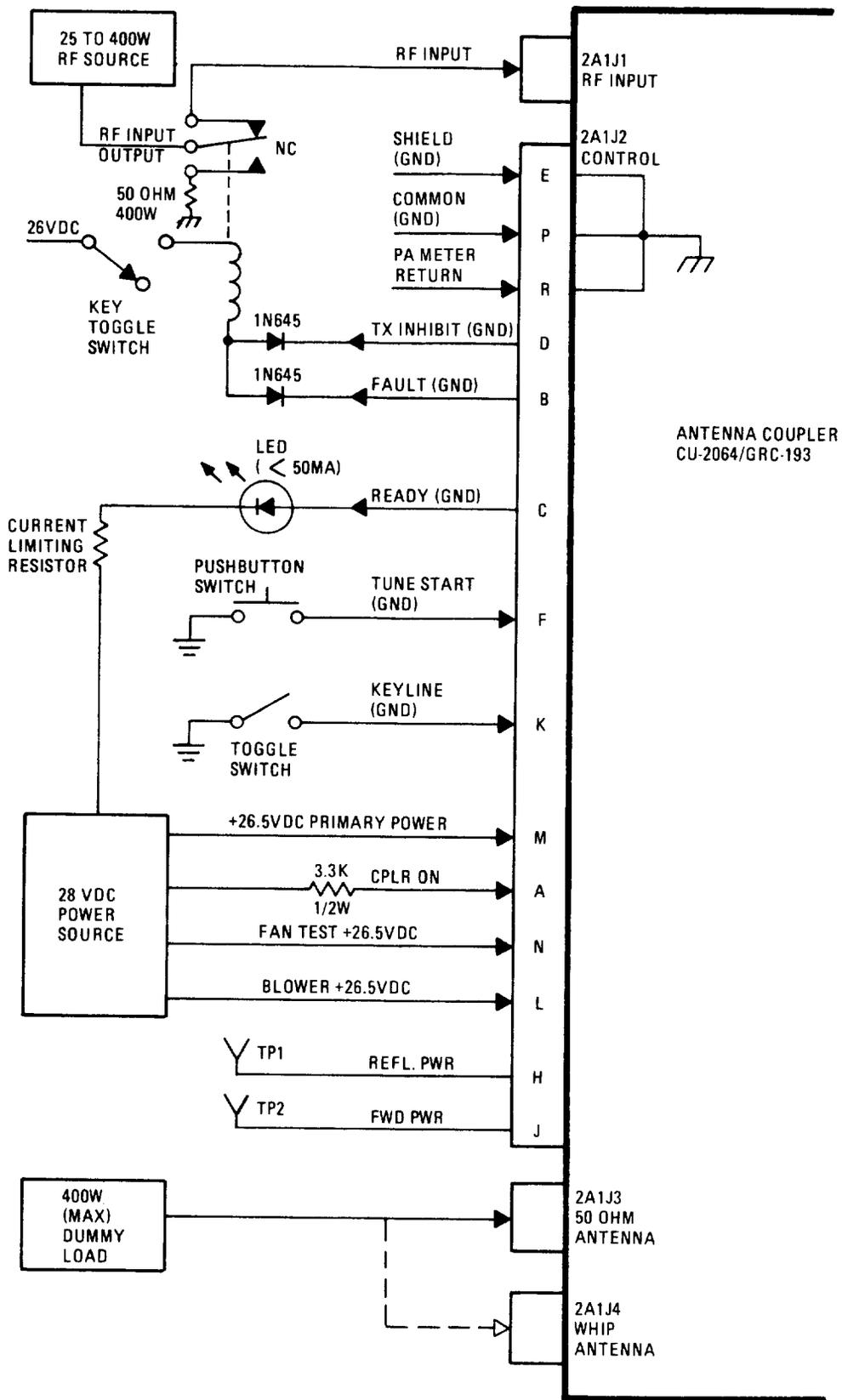
Figure 3-1. Special Test Setup for Testing Coupler
