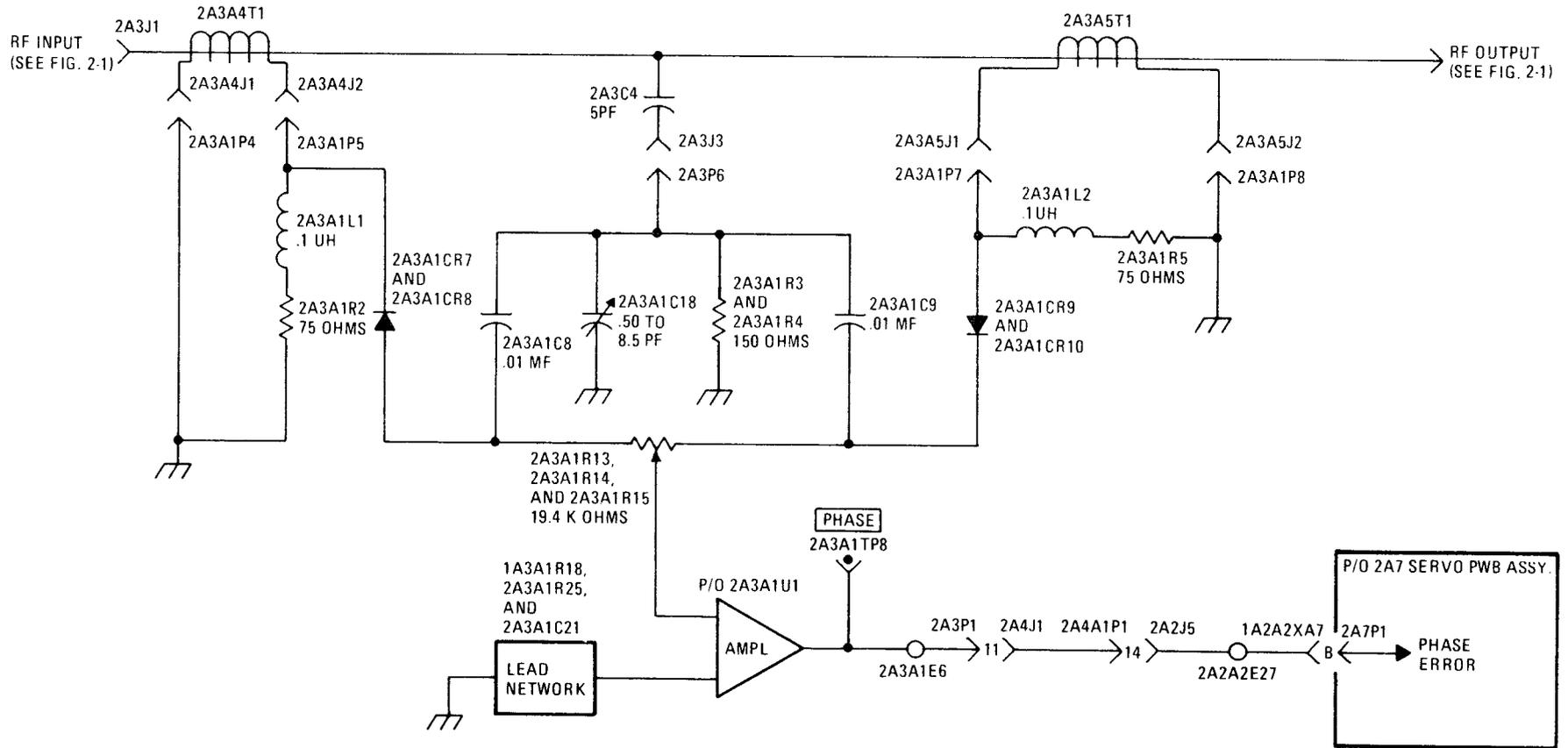
Figure 2-6. Simplified Phasing Discriminator Circuit Diagram
