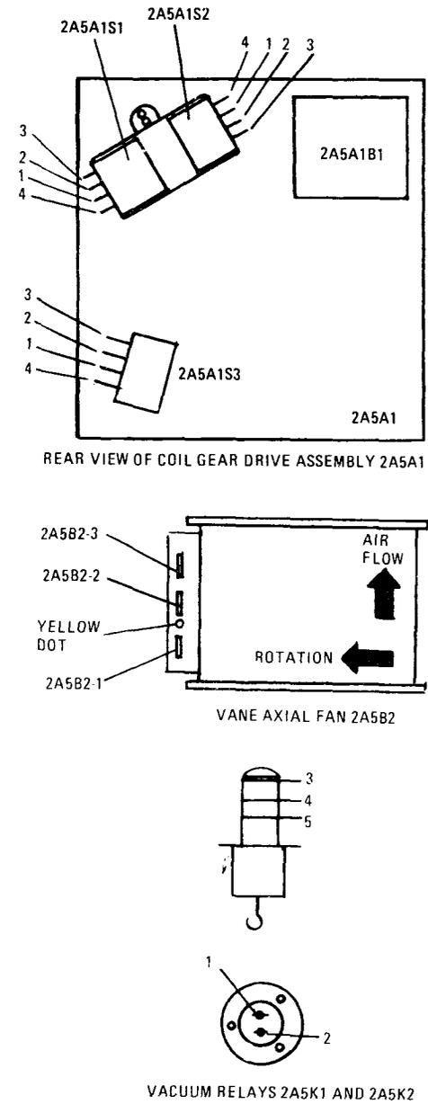
Figure 3-32. Inductive RF Tuner Assembly 2A5 Component Lead Identification Details
