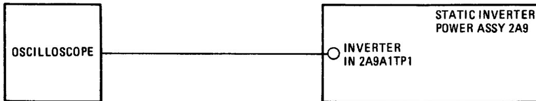
Figure 3-14. 400 Hz Zero Beat Adjustment Setup - Static Inverter Power Assembly 2A9
