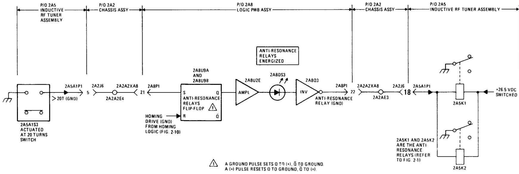
Figure 2-17. Simplified Anti-Resonance Relay Logic Diagram
