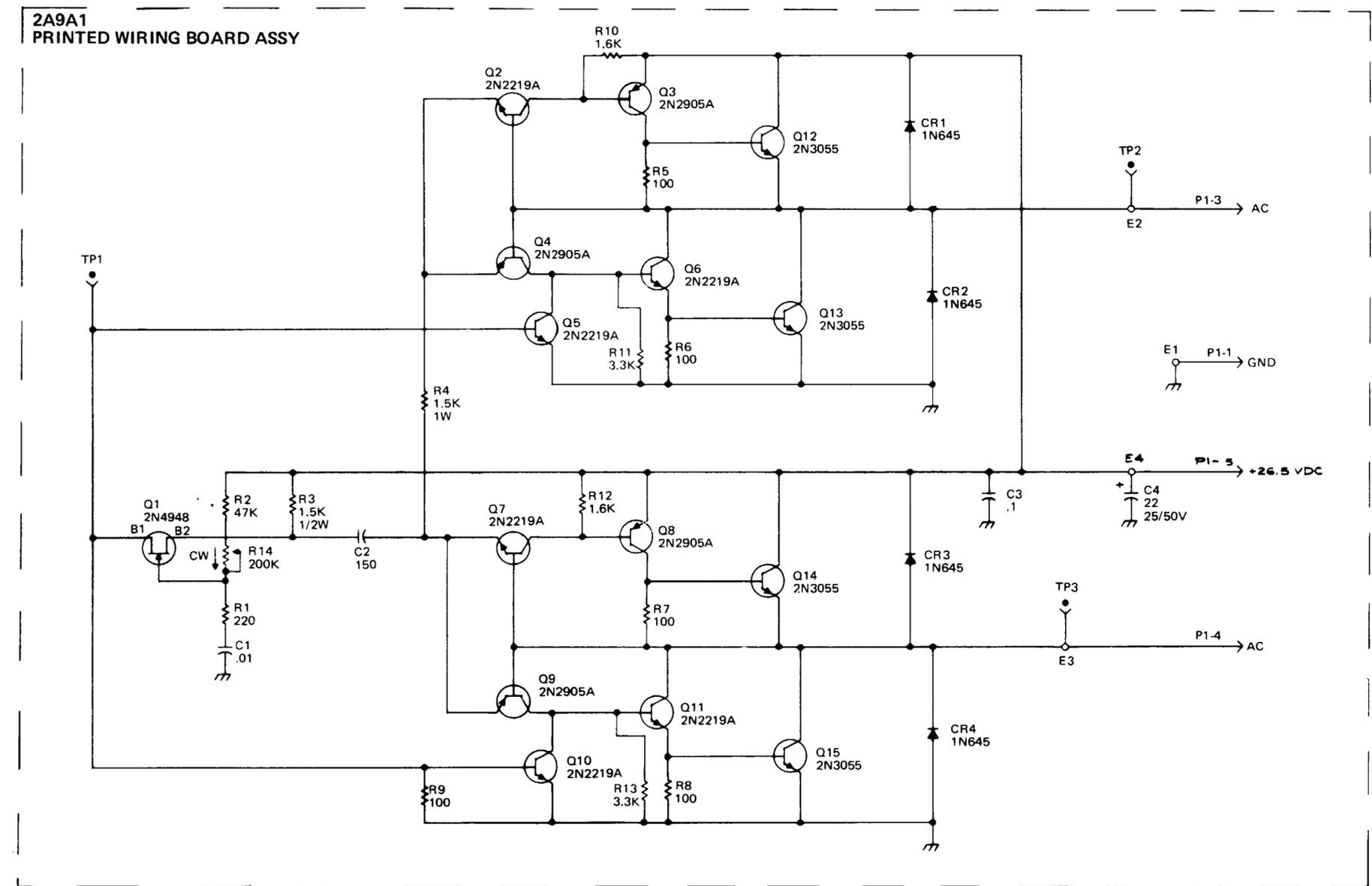
Figure 3-45. Static Inverter Power Assembly 2A9 Schematic Diagram
