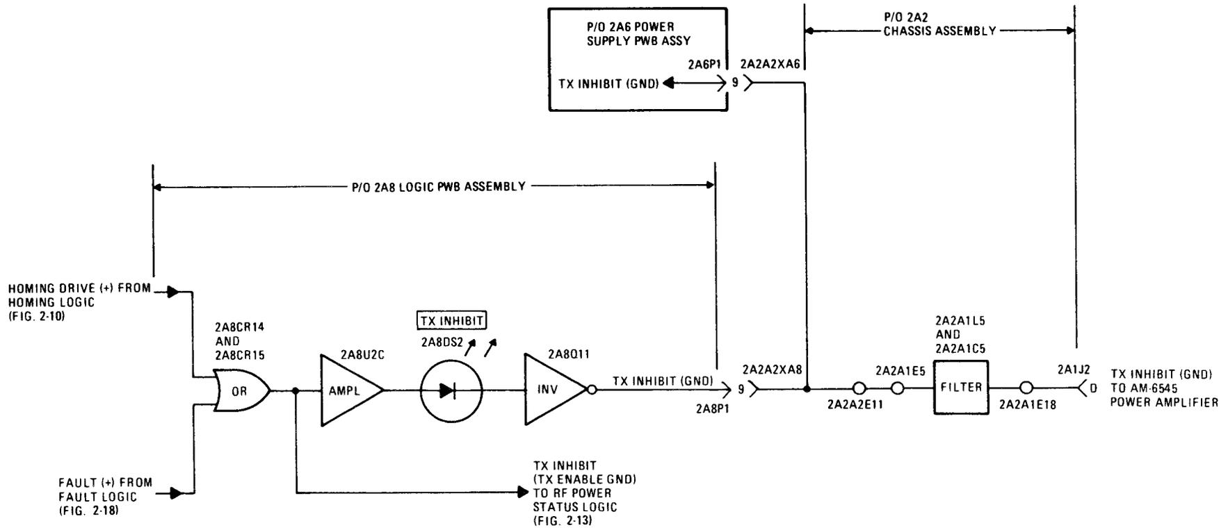
Figure 2-12. Simplified Transmitter Inhibit (TX Inhibit) Logic Diagram
