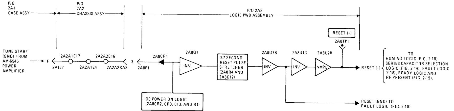
Figure 2-9. Simplified Reset Logic Diagram
