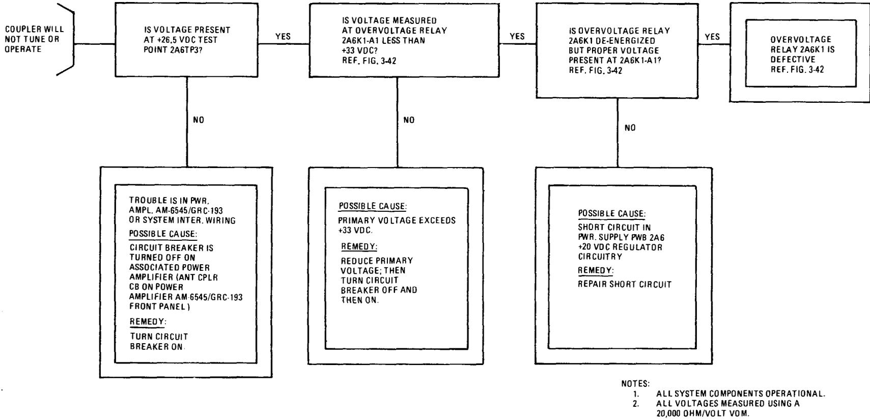
Figure 3-5, Dc Power Fault Logic Diagram
