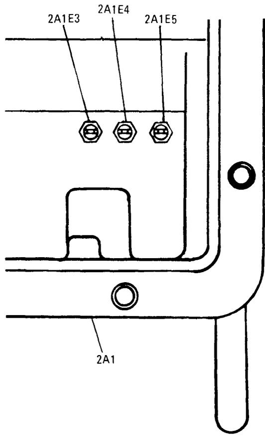
CASE ASSEMBLY 2A1 FAN CONNECTION POINTS
