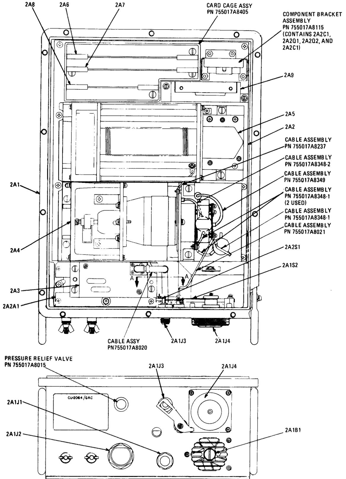
Figure 3-21. Antenna Coupler CU-2064/GRC-193 Component Locations
