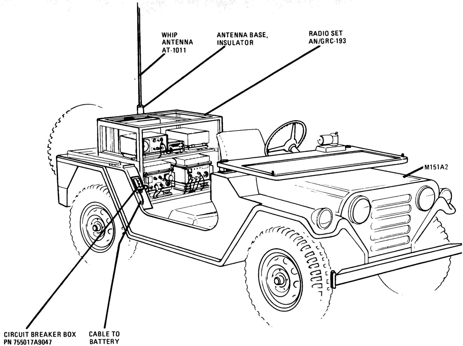
Figure 1-3. Radio Set AN/MRC-138 Component and System Relationships
