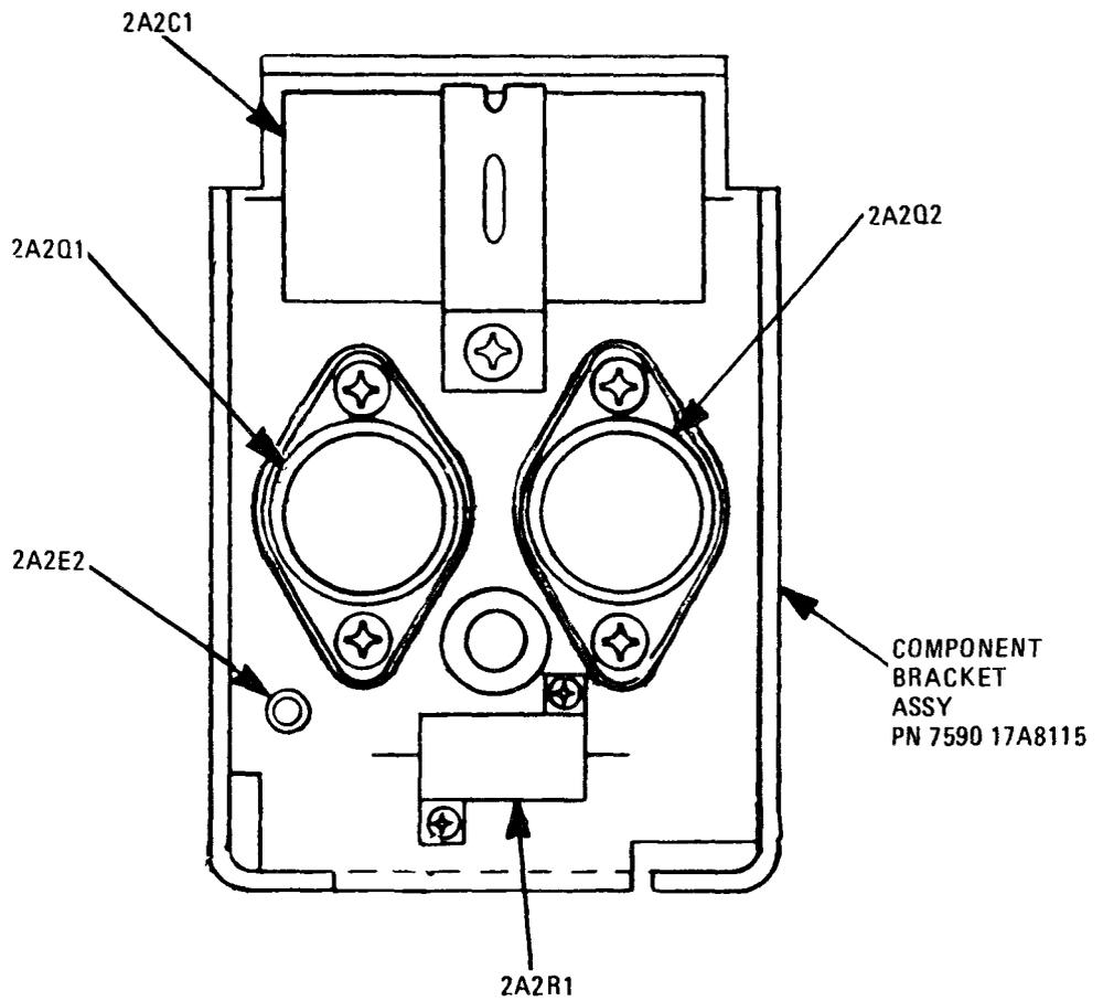
Figure 3-23. Component Bracket Assembly Part No. 755017A8115 Component Locations
