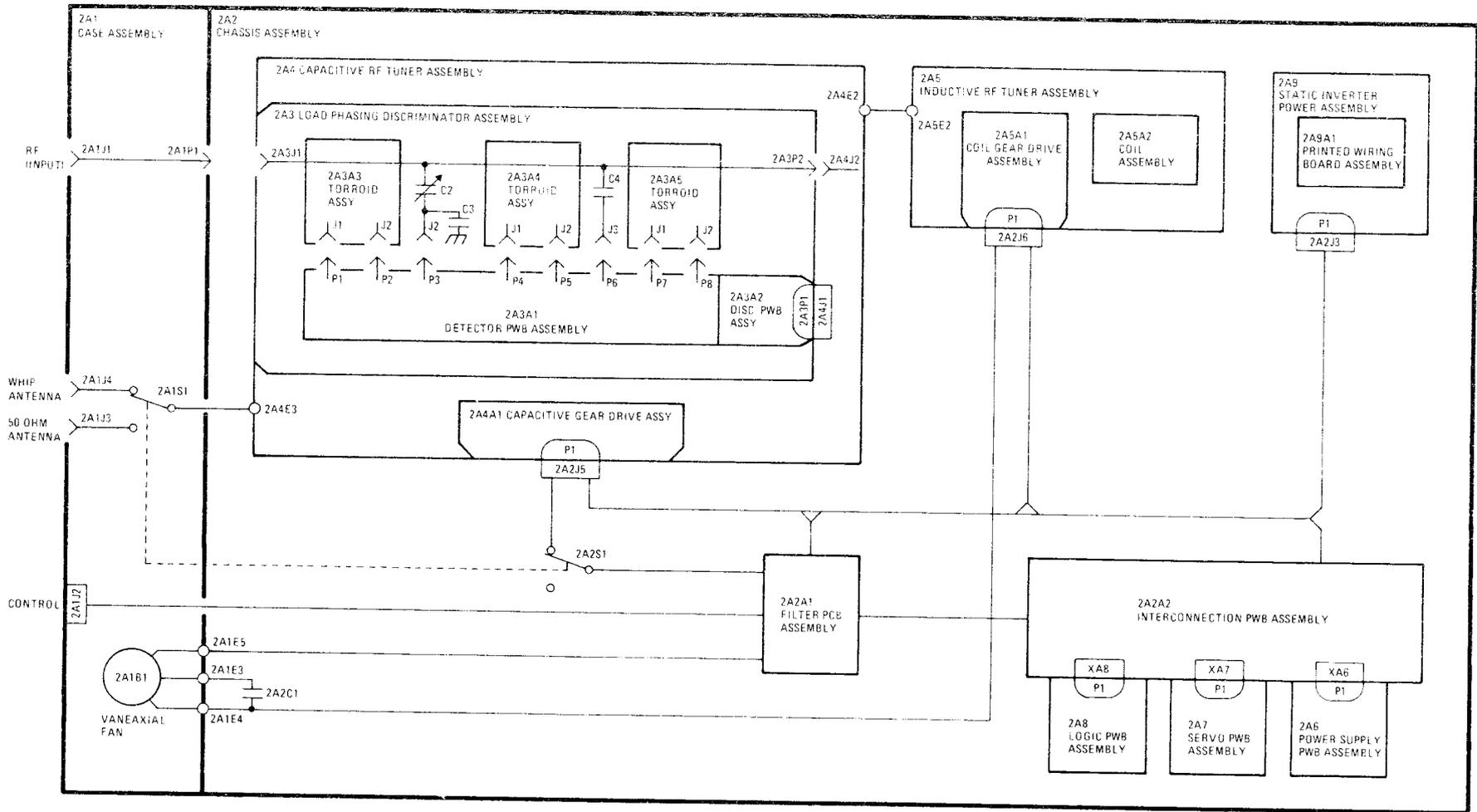
Figure 1-5. Antenna Coupler CU-2064/GRC-193 Component Interconnection and Identification
