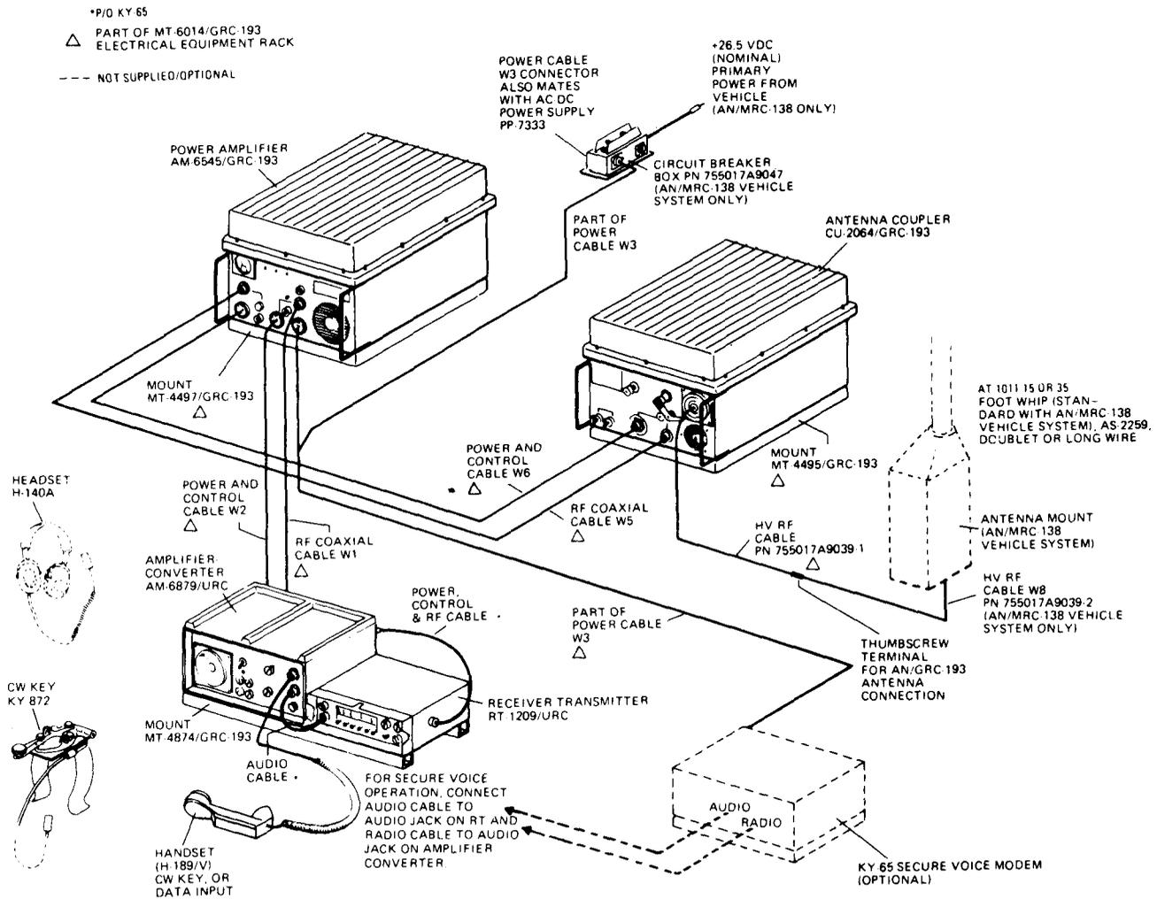
Figure 1-2. Radio Set AN/GRC-193 and Radio Set AN/MRC-138, Component and System Relationships
