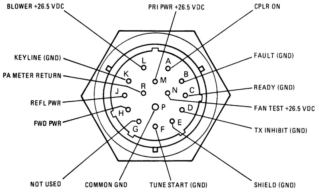
Figure 1-9. Connector 2A1J2 Pin/Functional Identification
