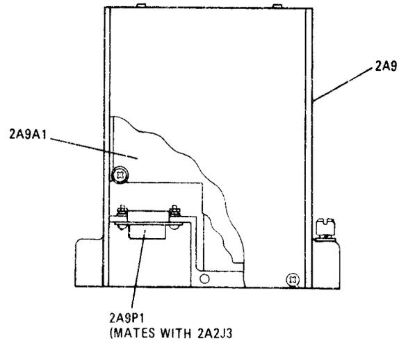
Figure 3-36. Static Inverter Power Assembly 2A9 Component Locations
