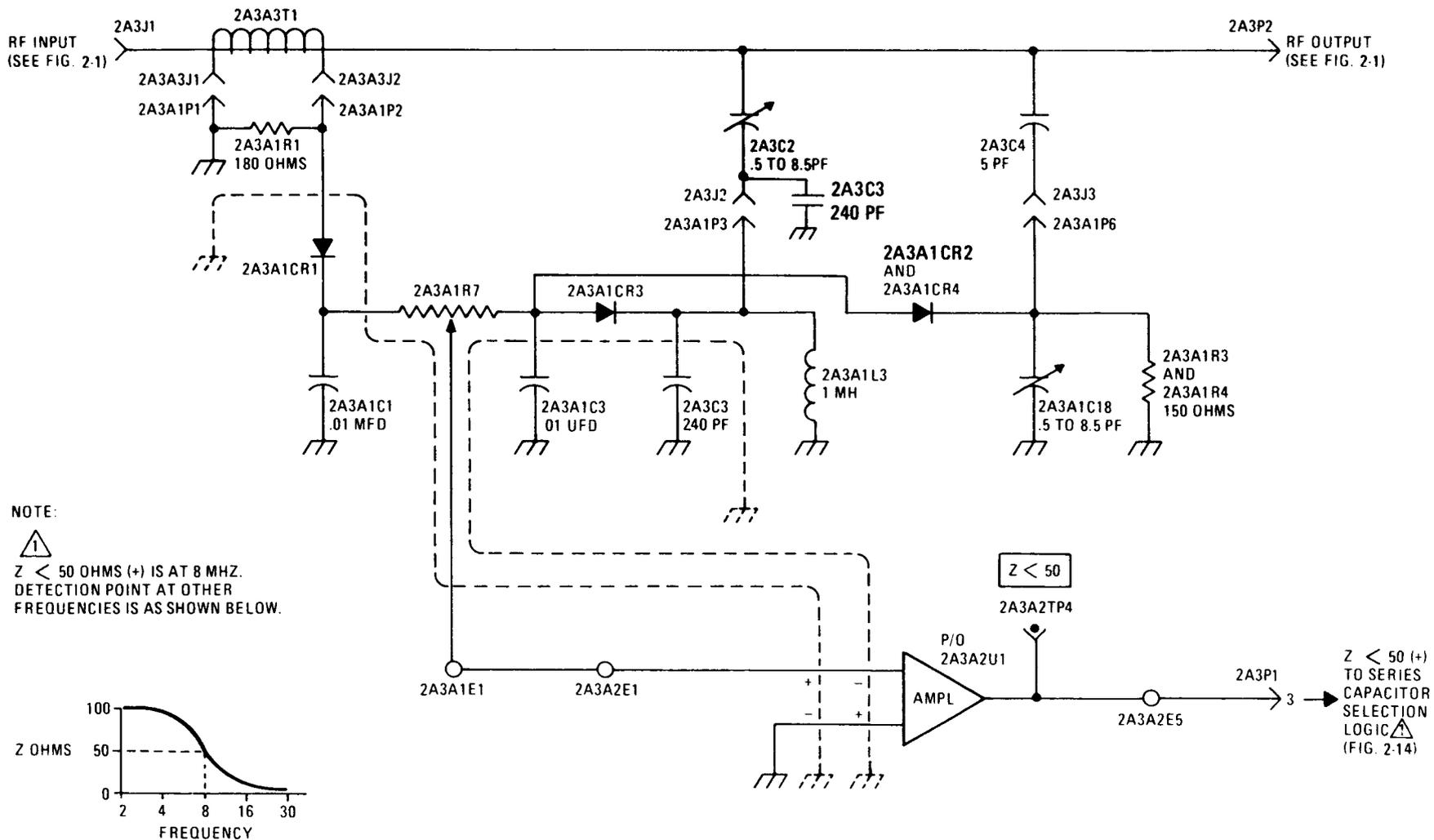
Figure 2-5. Simplified Z Discriminator Circuit Diagram
