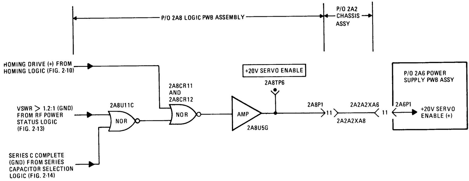
Figure 2-11. Simplified Servo Enable Logic Diagram
