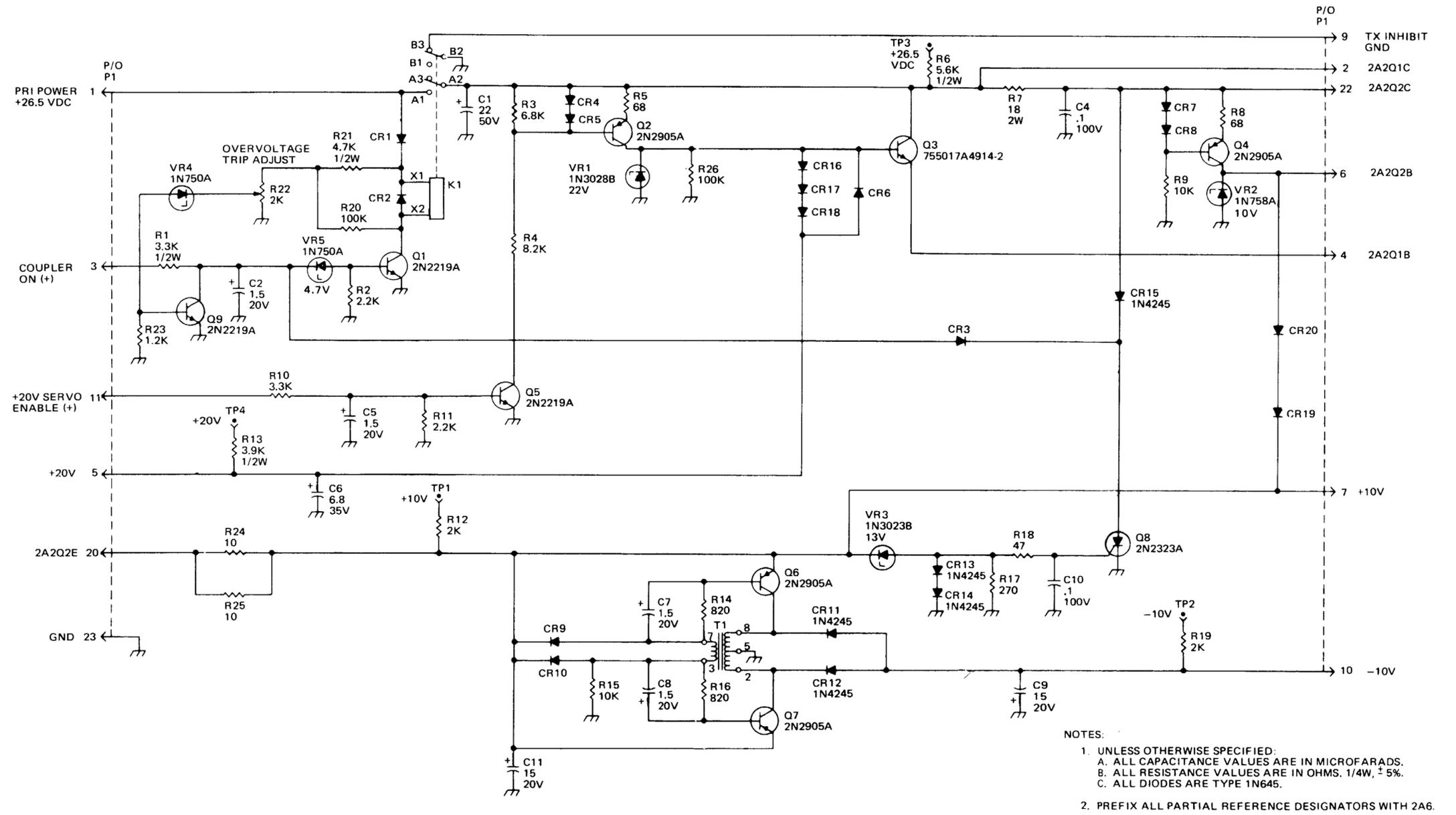
Figure 3-42. Power Supply Pwb Assembly 2A6 Schematic Diagram
