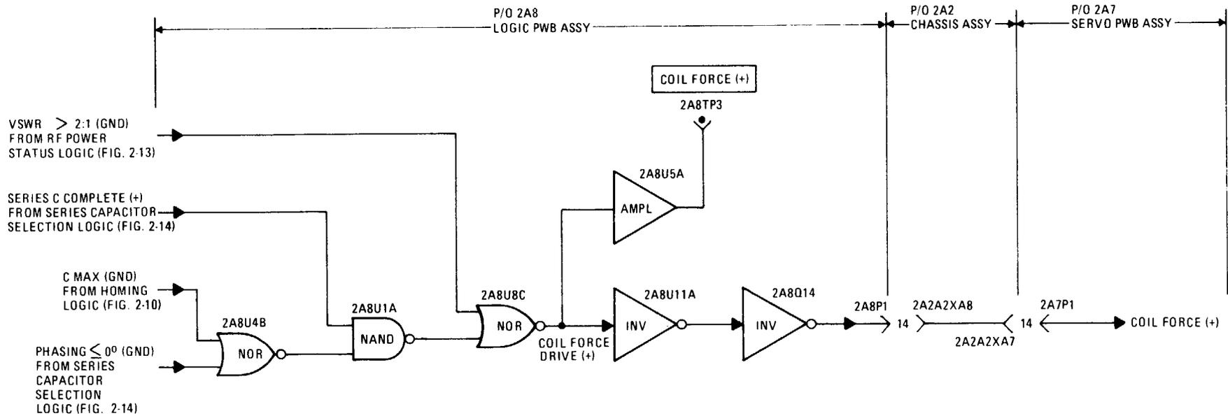
Figure 2-16. Simplified Coil Force Logic Diagram
