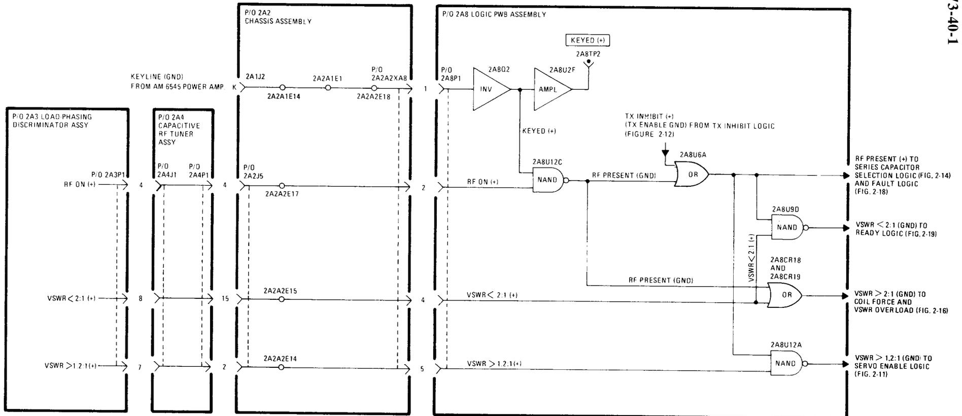
Figure 2-13. Simplified RF Power Status Logic Diagram
