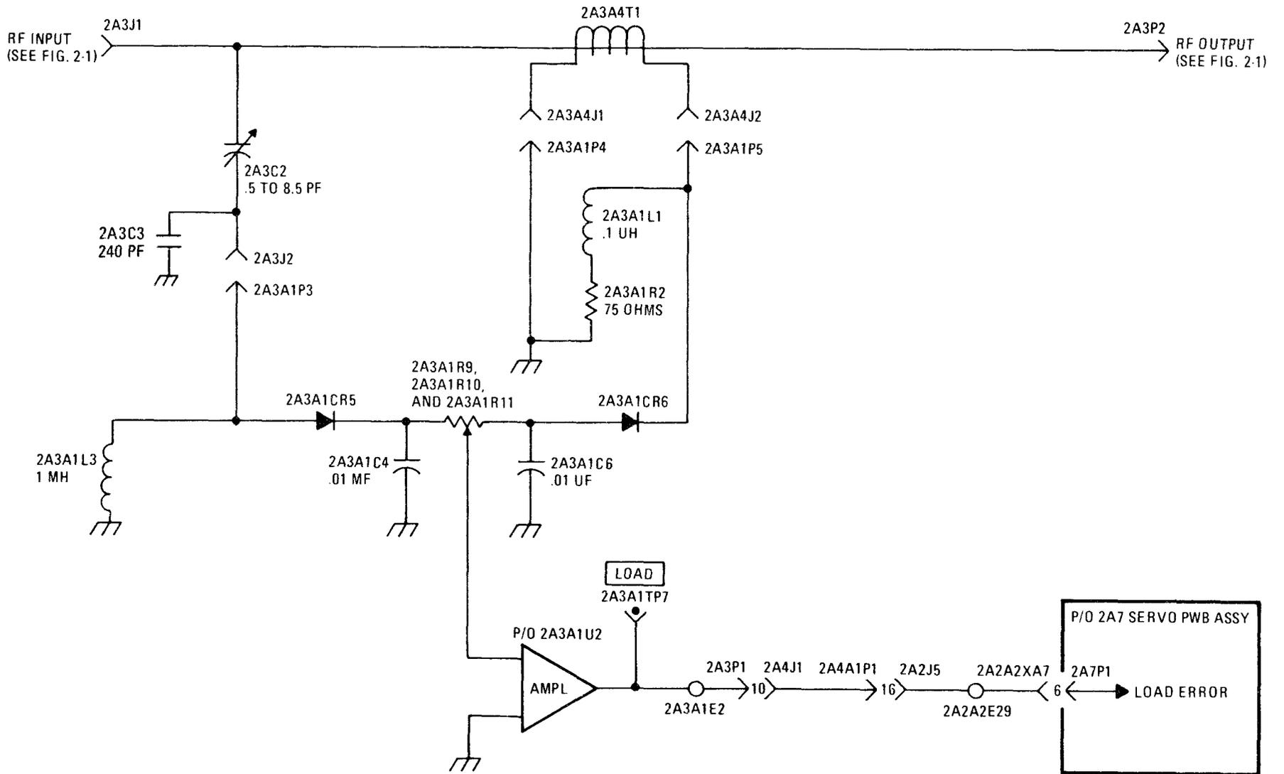
Figure 2-7. Simplified Loading Discriminator Circuit Diagram
