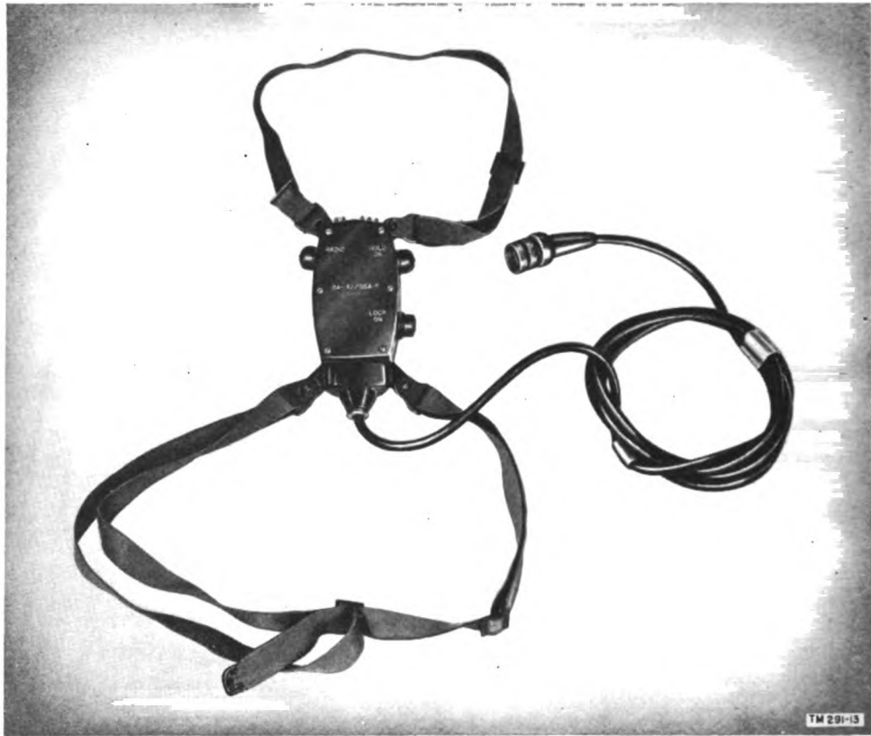
Figure 11. Chest Set Group AN/GSA-6, assembled.
