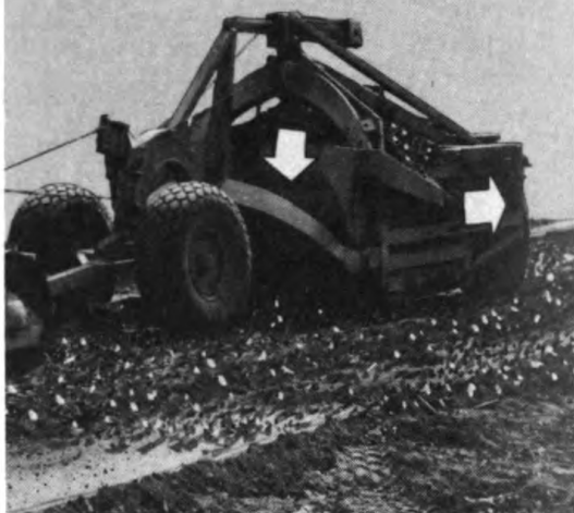
BACK UP WHILE LOWERING APRON AND RAISING BLADE
