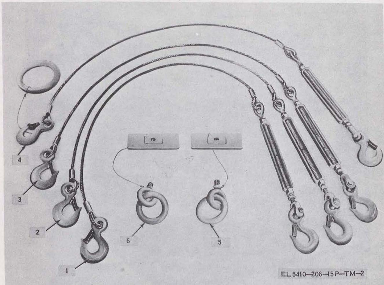
Figure 2. Sling assembly multiple leg.
