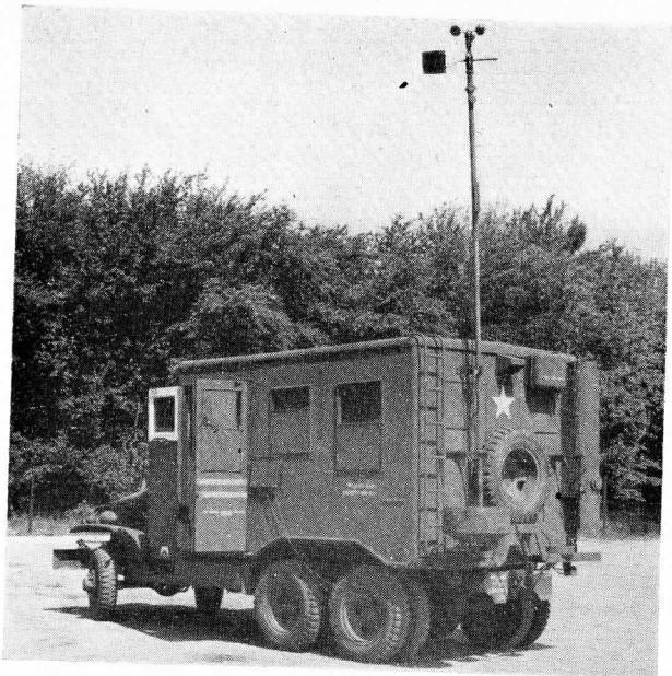
THE SCM-1 IS A MOBILE WEATHER STATION. SHOWN IN THE REAR VIEW ABOVE IS THE CEILING LIGHT PROJECTOR AND THE WIND EQUIPMENT.
