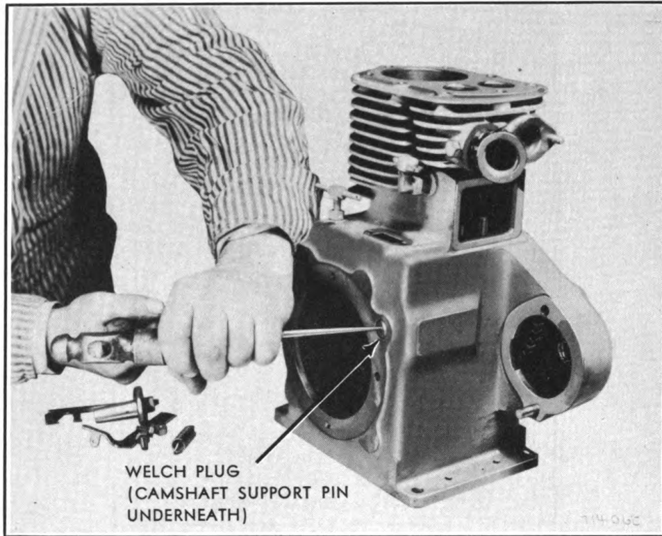
FIG. 110 Removal of Camshaft Support Pin
