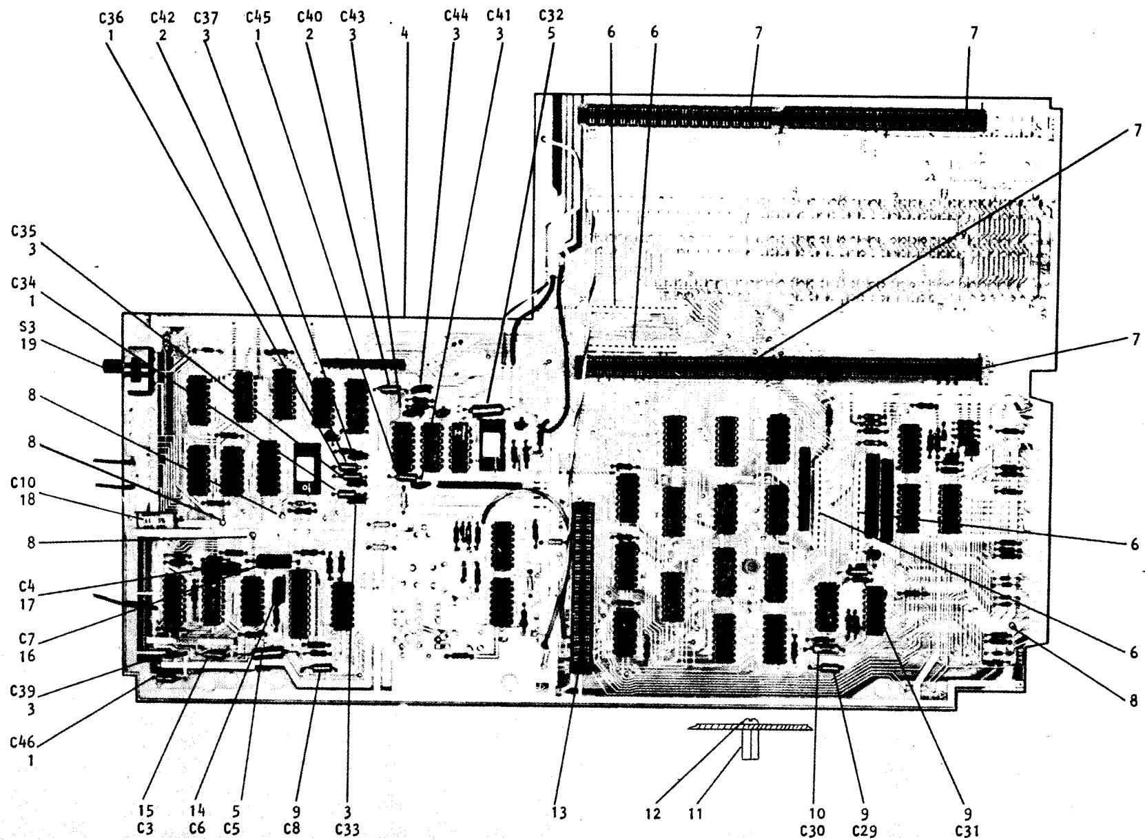
Figure 2. A1 Circuit Card Assembly (Sheet 1 of 4).
