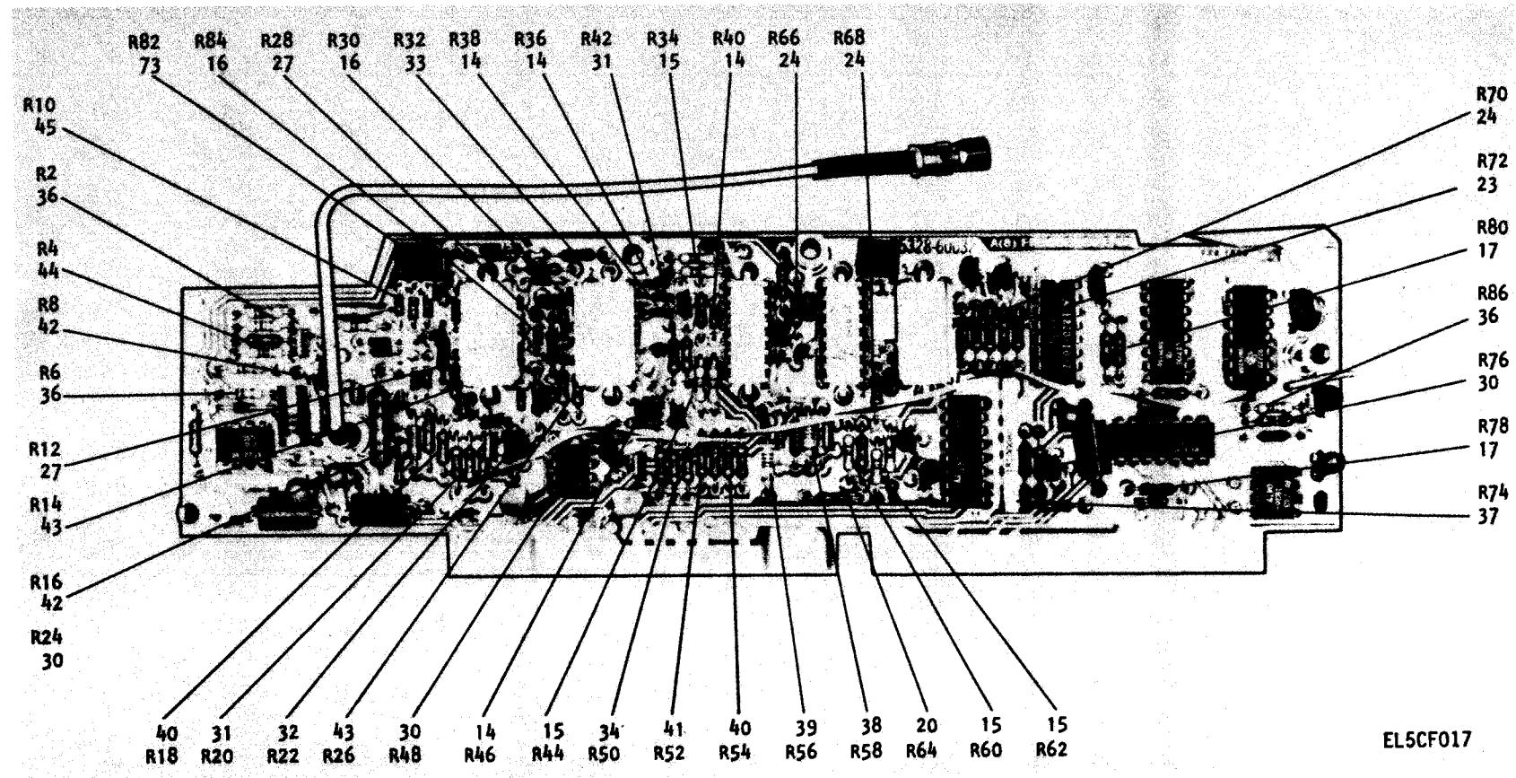
Figure 5. A8 Circuit Card Assembly (Sheet 3 of 5).
