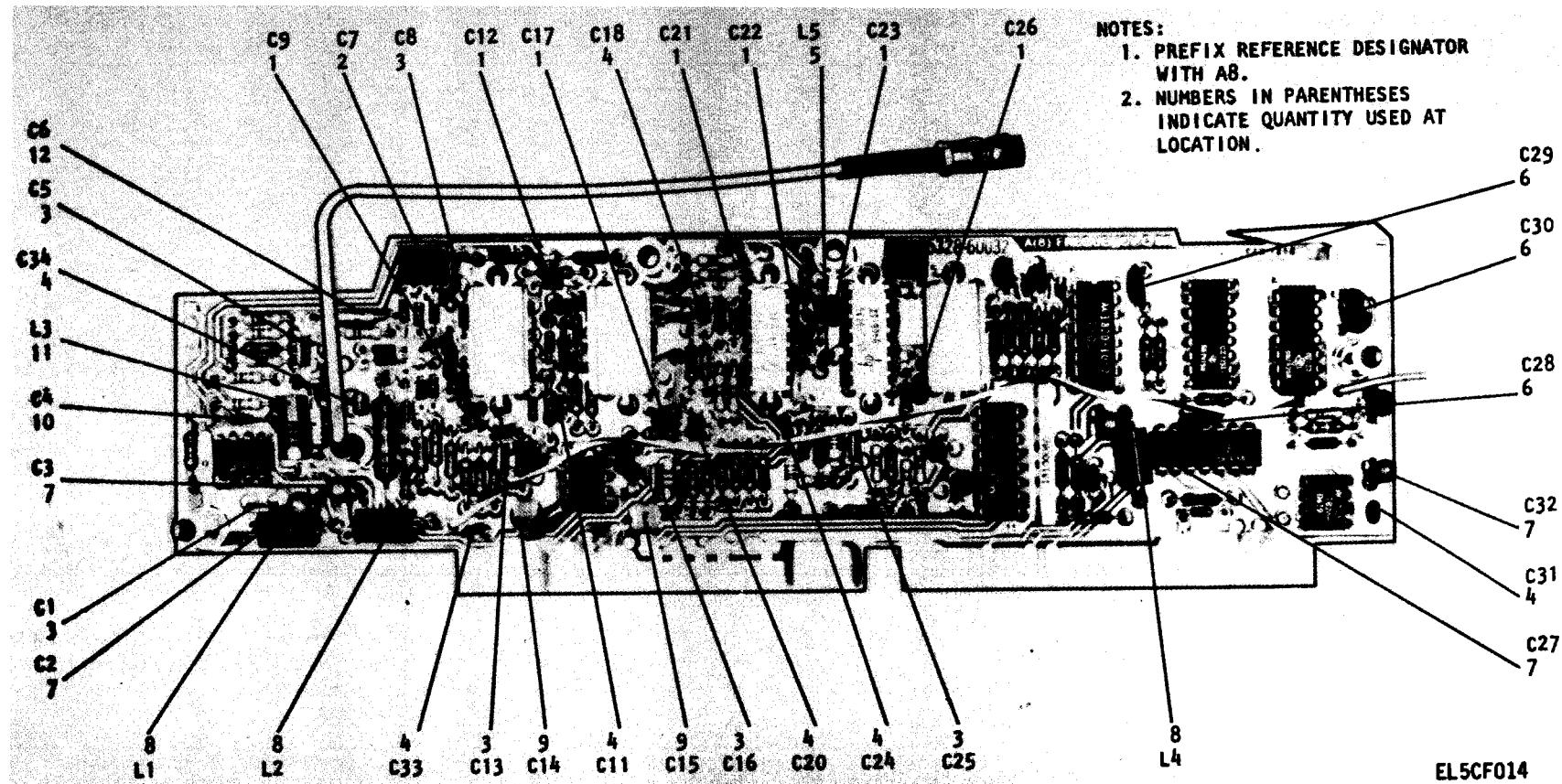
Figure 5. A8 Circuit Card Assembly (Sheet 1 of 5).
