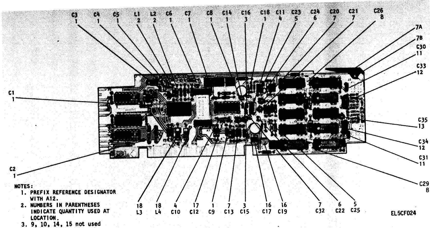
Figure 6. A12 Circuit Card Assembly (Sheet 1 of 3).
